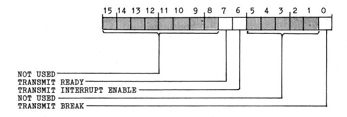
FIGURE 3-3: XCSR (17XXX4) REGISTER FORMAT
