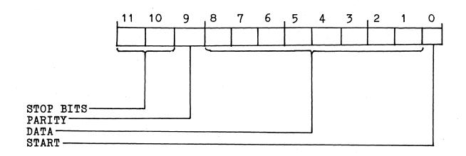
FIGURE 3-6: ASYNCHRONOUS TRANSMISSION FORMAT
