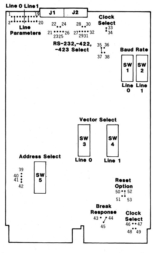
FIGURE 2-1: SWITCH AND JUMPER LOCATIONS
