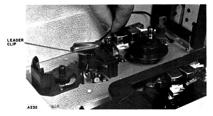
Figure 4-5. Removing the Leader Clip From the Clip Channel
