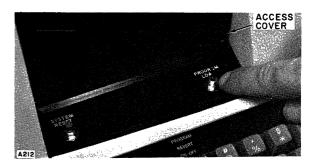
Figure 2-1. Location of the Power On/Off Switch
