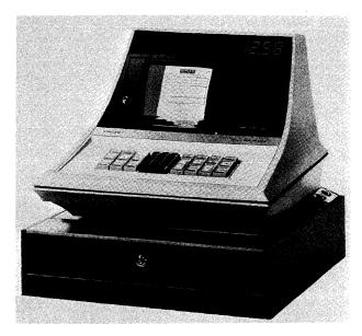
Singer's MDTS Data Terminal, the key component of the Modular Data Transaction System, is a "computerized cash register" that can be used effectively with the System Ten in either an on-line or off-line mode.
