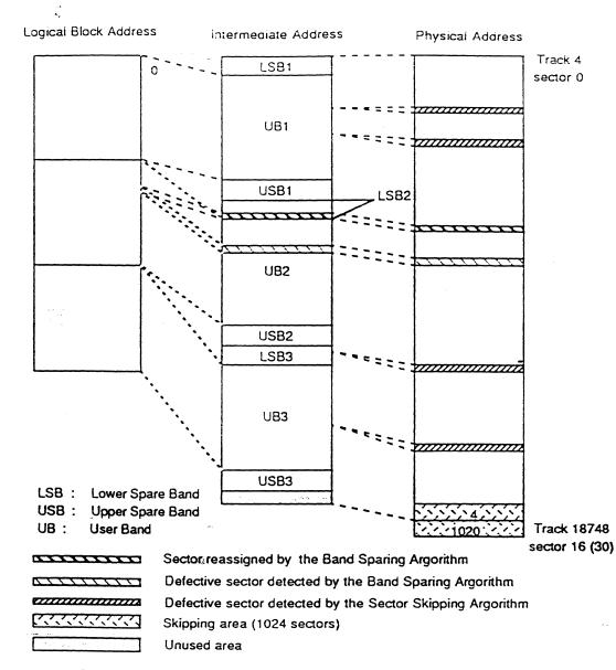
Fig. 3.3 An example of address allocation in Format Mode 2
