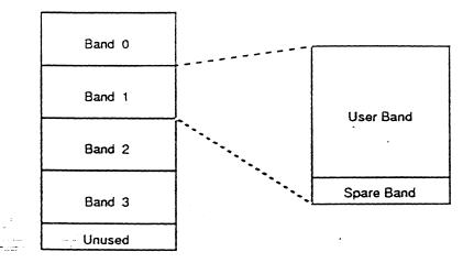
Fig. 3.2 Structure of Bands, Linear Replacement Algorithm
