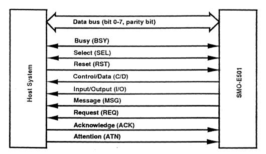
Fig 5.1 : SCSI Data Bus and Signal Lines
