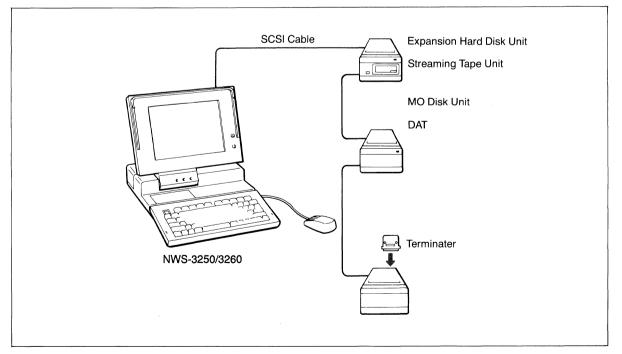
\*Connection between the NWS-1250 and the first storage device must be done via the PCZ-310T SCSI cable.
