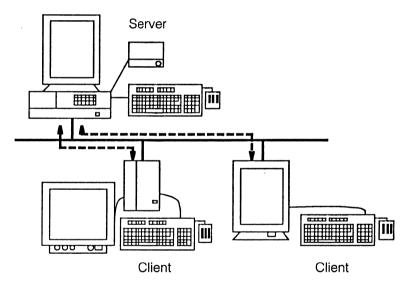
When booting the Client, all of the Client data including the program and the kernel program must be downloaded from the Server.
