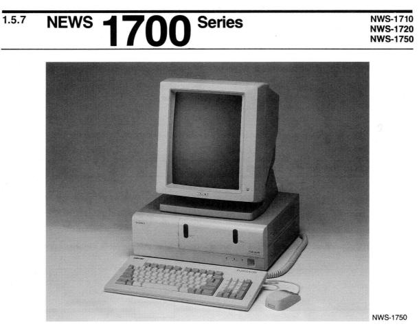
The incorporation of the latest 32-bit microprocessor MC68030 and a high-speed cache memory makes the NWS-1700 Series a powerful 4.3 MIPS machine.
