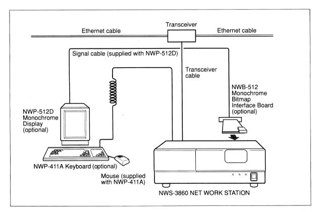
When using the workstation as a standalone system, no Ethernet transceiver is required.
