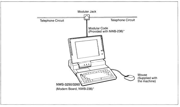
\*NWB-238 is designed based on the Japanese telecommunication standard and can be used only in Japan.
