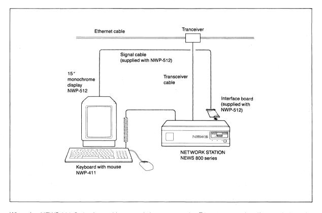
When the NEWS 800 Series is used in a stand-alone system, the Ethernet transceiver illustrated above is unnecessary.
