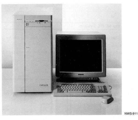
Featured in the NWS-900 Series is an internal 125-Mbyte streaming tape drive and a hard disk capacity of 1.1 Gbytes (for NWS-921). Also included are VME slots for four triple height Eurocards and four option board slots, offering expandability to a more advanced system.
