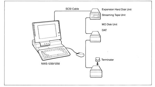
\*Connection between the NWS-1250 and the first storage device must be done via the PCZ-310T SCSI cable.
