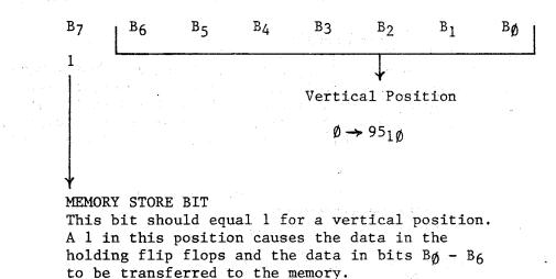
When programming a design to appear on the screen there are two ways the characters can be loaded the method you use depends on how your software is organized. One method is to just send out successive coordinates (H1, V1); (H2, V2) etc., until all H, V locations are specified. With this method two bytes must be sent out for each character.
