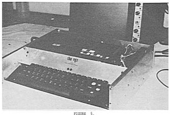
The Video Graphics Terminal prototype with the top cover removed
