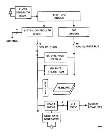
FIGURE 3. VGT Control Processor
