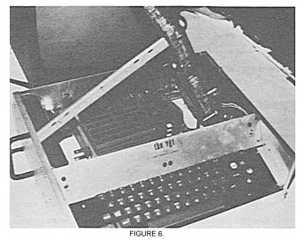
The Video Graphics Terminal with the control electronics up and the memory boards
