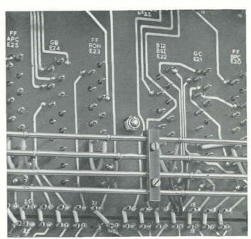
Close-up of a section of STANTEC-ZEBRA printed circuit showing wrapped-joint technique at terminals.
