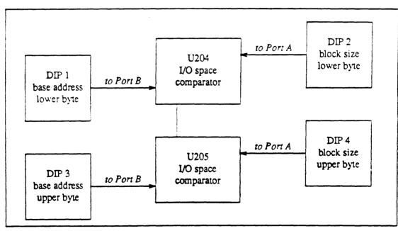
3.3. VMEbus to Multibus Addressing During a VME read cycle to a Multibus card, P1 address lines A01-A23 are transferred to the Multibus adapter card in conjunction with P1 address strobe (AS) and P1 data strobes (DS0, DS1). If the Multibus board is a 24-bit address master, the four high-order address bits (A23-A20) are passed through by setting switch sections 5-8 of DIP switch 11 ON. Address lines which pass on to
