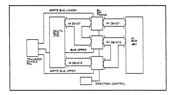
FIGURE 7C-4: VME/MULTIBUS DATA TRANSFERS
