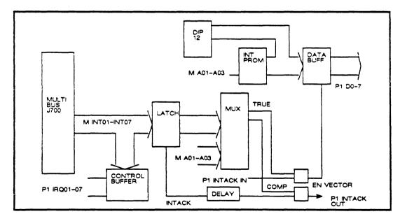
FIGURE 7C-5: INTERRUPT LOGIC
