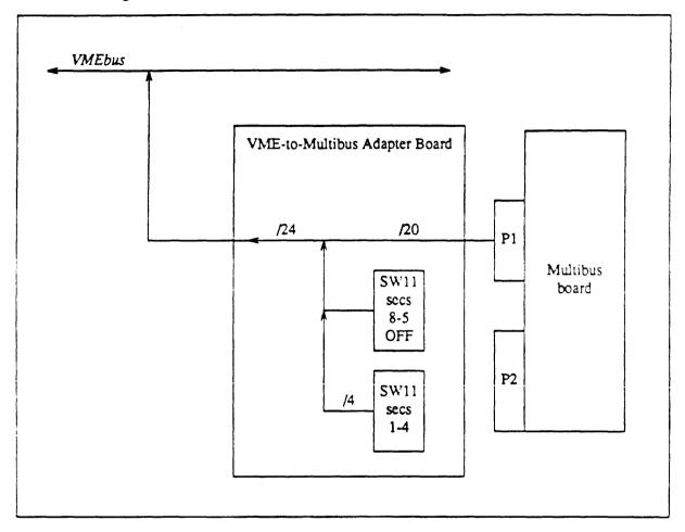
Figure 2-12 20-bit Multibus DMA Cycle
