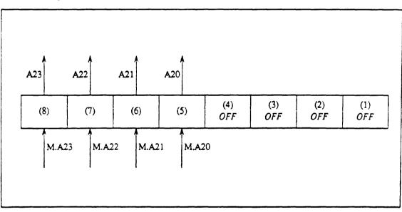
Figure 2-10 DIP Switch 11, Sections 5-8
