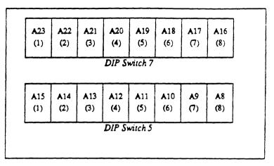
Figure 2-3 Address Switches for the 24-Bit Multibus Memory Space
