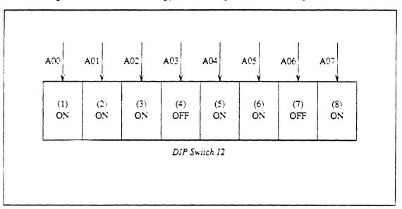
Figure 2-14 Switch Setting for an Interrupt Vector Number of 0x48
