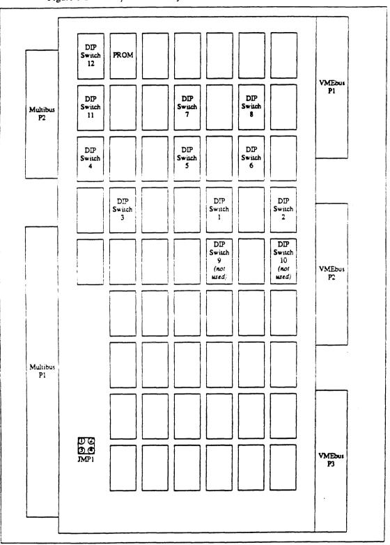
Figure 1-2 Adapter Board Layout
