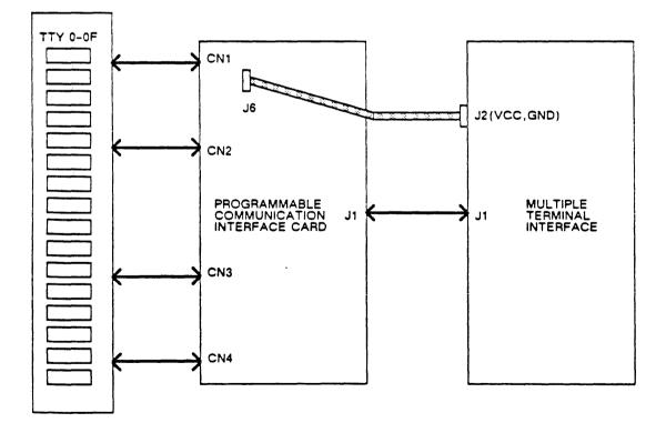
FIGURE 7C-14: PROGRAMMABLE COMMUNICATION INTERFACE (SECOND ALM BOARD)
