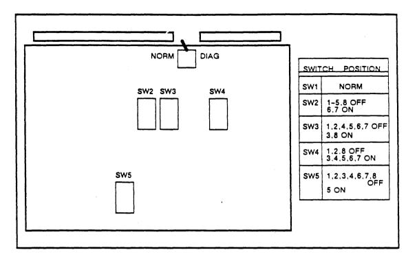
FIGURE 7C-13: ALM BOARD DIP SWITCH SETTINGS
