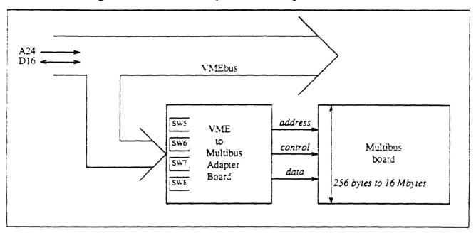
Figure 2-2 Multibus Memory Address Decoding
