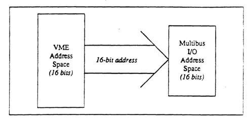
Figure 3-3 VME and Multibus I/O Address Space
