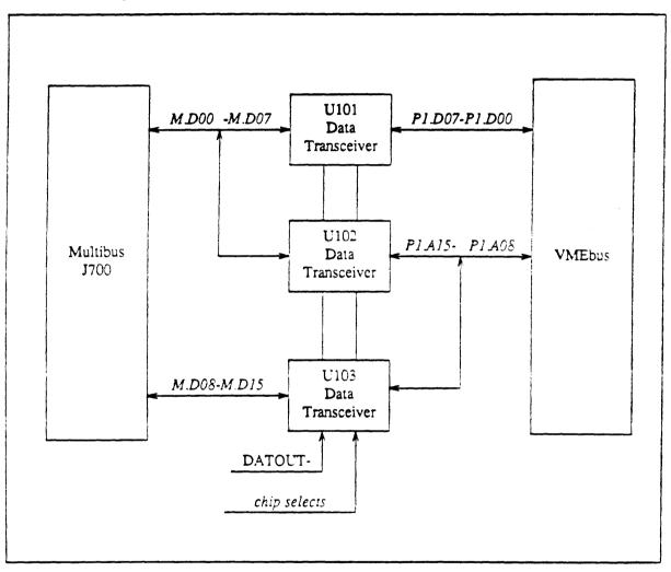
Figure 3-7 Data Signal Flow: Multibus Board to VMEbus
