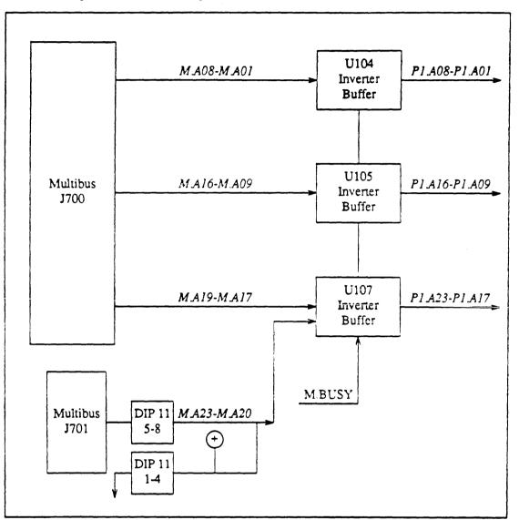
Figure 3-6 Address Signal Flow: Multibus Board to VMEbus
