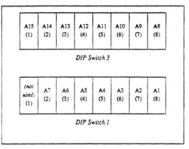
Figure 2-8 Address Switches for the Multibus I/O Space
