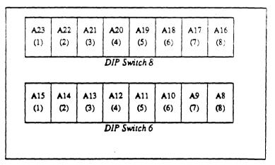
There is a separate switch section for each address bit from A8 to A23.
