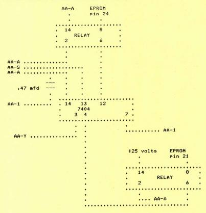
Above is the schematic for Jack's Automatic EPROM Programmer Switcher. His revised wiring list for the EPROM Programmer is on page 5/6 -7. Please note that the BASIC listings for the EPROM PROGRAMMER and for the PLOT programs are NOT published in this issue! Only the instructions for these five programs are given here, so that you can decide whether or not they will be useful enough to purchase in cassette form from JACK BUILT PROGRAMS.
