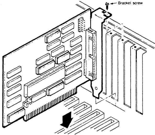
**SC5500 Internal Tape Controller Board**
