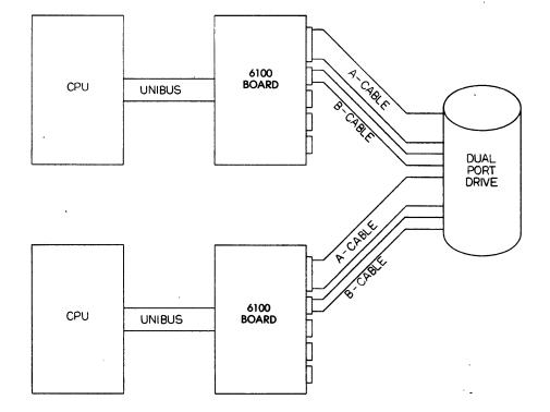
Figure 1-2. Dual Port Configuration
