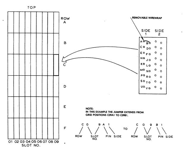
Figure 4-3. NPG Jumper Location
