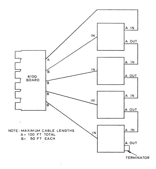
Figure 1-1. Disk Drive Configuration
