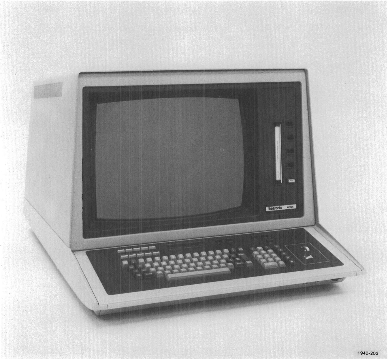
Figure 1-1. TEKTRONIX 4054 Graphic Computing System.
