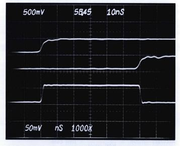
Fig 2: The delay time between the input of a delay line (upper trace) and the output of the delay line (middle trace) is measured digitally. Lowe trace is 7D15 Pseudo Gate display.
