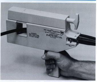
The CT-5 is a clip-on High-Current Transformer designed to extend the measurement capability of TEKTRONIX clip-on current probes. Maximum low-frequency performance is obtained using the P6042 DC Current Probe. Maximum pulse current up to 50,000 A may be measured provided the 8 A-sec rating is not exceeded. It may also be used with the P6021 (not compatible with P6022) in conjunction with a current probe amplifier for measurements at normal power line frequency and above.
