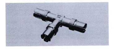
This coaxial tee has a 16.67-ohm resistor in each leg, connected so that the tee looks like 50 ohm if two legs are terminated in 50 ohm. It is designed for use in broad-band 50-52 systems where the mismatch introduced by ordinary "Tee" connectors is undesirable. It is especially useful in a time-domain reflectometer set-up where test line, pulser, and oscilloscope must be coupled with a minimum of reflection-producing discontinuities.
