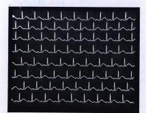
8-Channel Y-T Displays—Full-Screen normal or single sweep displays are swept at 10 μs to 50 s full scale, from a time base internal the 4701. Oscilloscope-type triggering also provided. Simulated ECG is shown.
