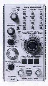
The exceptionally fast sweep speed of the 7B92 matches the ultra-high bandwidth of the 7904/R7903 mainframes. Four display modes contribute more to the superior performance of the overall package. They are normal, intensified delaying sweep (controllable contrast), delayed sweep and alternate. Alternate mode, when selected, displays the main sweep with the intensified portion and the delayed waveform at the same time.
