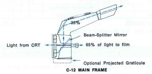
The C-12 mirror system provides a straight-on view of the CRT, and minimizes parallax due to an external graticule. An optional Projected Graticule accessory provides changeable parallax-free graticules of various patterns; see page 208.
