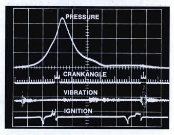
Simultaneous displays of four engine parameters provide the operator with one comprehensive picture of the total engine performance and make identification of malfunctions easy.
