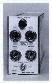
The 7M11 is a passive dual DELAY LINE unit for use with the 7000-Series sampling system. In low-repetition rate applications, requiring the sequential mode of operation, the 7M11 provides the trigger source and signal delay necessary to view the triggering event at the faster time per division settings. Very fast triggering events will not be displayed at the slower time per division settings of most sampling sweep units.
