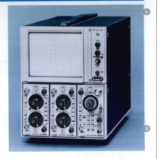
The new 5400-Series combines outstanding versatility and low cost in a 60-MHz, general-purpose, plug-in oscilloscope system. It features CRT READOUT of plug-in scale factors, a three plug-in mainframe, a choice of \*17 plug-ins, and easy benchto-rackmount convertability.
