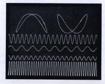
MIXED X-Y and Y-T Displays—Simultaneous display of four frequencies versus time and two frequencies versus two other frequencies. Other display combinations include 1 X-Y with 6 Y-T displays and 3 X-Y with 2 Y-T displays.
