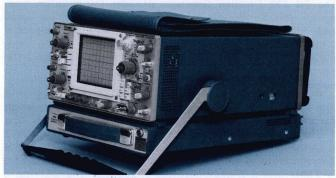
The 1106 Battery Pack provides compact battery operation for the Option 7 version of the 465 and 475. The addition of Option 7 allows these scopes to operate on 12 or 24 VDC. he 1106 Battery Pack supplies 24 VDC with 140 watt-hour capability to the instrument.
