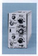
The 7A24 and 7A26 Dual-Trace Amplifier plug-ins provide a maximum bandwidth of 350 MHz with  $50-\Omega$  input (7A24) and 200 MHz with  $1-M\Omega$  input (7A26), for the 7000-Series mainframes. This bandwidth is constant for all deflection factors from 5 mV to 5 V. Other features include versatile trigger source selection, five operating modes, and a bandwidth limiting switch for low-frequency applications.
