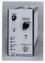
25 Hz or less ( $\pm 20\,^{\circ}\mathrm{C}$  to  $\pm 75\,^{\circ}\mathrm{C}$ ) 30 Hz or less (0°C to  $\pm 20\,^{\circ}\mathrm{C}$ ) with P6021 (lower -3 dB). 250 Hz or less with P6022 (lower -3 dB). \*Refer to Ruggedized Oscilloscope System.
