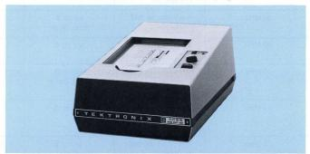
The 4632 Video Hard Copy Unit makes facsimile copies from refreshed CRT display terminals or analog TV signals. It accepts video information, consisting either of composite video or separate video and composite sync, and produces a sharp copy of the displayed information.
