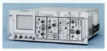
The R7704 requires 7 inches of rack height and is the only four-plug-in rackmount oscilloscope available today; it offers 175 MHz bandwidth.
