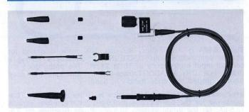
The P6065A is a miniature passive probe with precise 10X attenuation for use with the TEKTRONIX 465 Oscilloscope. When used with the 465 Oscilloscope, the bandwidth will be 100 MHz. When compensated to other 20-24 pF input capacitance instruments the bandwidth will be at least 75 MHz.
