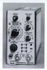
The 7A22 is a differential amplifier for use with all 7000-Series mainframes. Basic performance features are 10  $\mu$ V/div to 10 V/div deflection factors, DC to 1 MHz bandwidth with selectable HF and LF -3 dB POINTS, common mode rejection ratio of 100,000:1 at 10  $\mu$ V/div, DC coupled, differential signal range  $\pm$ 1 V at 10  $\mu$ V/div, and a DC OFFSET feature with  $\pm$ 1 V range  $\pm$ 100,000 div at 10  $\mu$ V/div.
