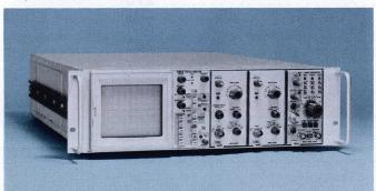
The R7903 Oscilloscope is the widest bandwidth, real-time oscilloscope available in a 5¼-inch rackmount. General-purpose measurements up to 500 MHz at 10 mV/div can be made using
