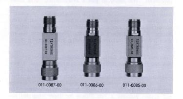
Attenuators are all supplied with Type N fittings. See accessory section for adapters for other series. Frequency range is DC to 12.4 GHz. Power rating is 2 W average, 300-W peak. Impedance is 50  $\Omega$ .
