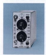
The 5A48 Dual-Trace Amplifier provides 60-MHz bandwidth for the 5403 Oscilloscope. It features five operating modes, selectable trigger source, and calibrated deflection factors of 1 mV/DIV to 10 V/DIV (bandwidth reduced below 5 mV/DIV).
