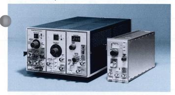
The TM 500 calibration system provides the signals required to calibrate most oscilloscopes. This system consists of the PG 506 Calibration Generator, SG 503 and SG 504 Sine Wave Generators, and the TG 501 Time Mark Generator. Any of the other TM 500-Series plug-ins can be used along with these units to comprise a complete test and measurement system.
