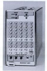
The 7M13 Readout Unit provides front-panel keyboard operation for convenient access to the CRT READOUT characters. The 7M13 is designed for use in all 7000-Series mainframes except those without CRT READOUT, and will function in any plug-in compartment. A remote-advance cable is supplied with the 7M13 to provide connection to the shutter x-sync connector of the C-50-Series Cameras. An optional cable is available for cameras using an ASA connector for x-sync.
