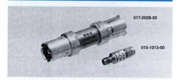
The coupling capacitor is a short length of coaxial line having a disc capacitor (4700 pF,  $\pm$ 20%) in series with the inner conductor. Reflection ratio (in 150-ps TDR system), maximum is 0.03. Voltage rating is 200 Volts.
