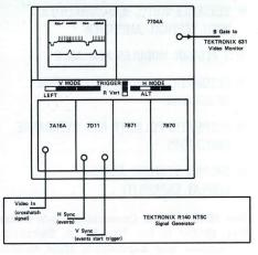
Fig. 5: Equipment set up for figures 3 and 4.
