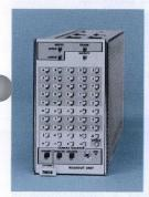
The 7M13 Readout Unit provides front-panel keyboard operation for generation and display of up to 20 CRT READ-OUT characters (10 at the top of the CRT, 10 at the bottom). The 7M13 also contains a sequence counter which can be automatically advanced from the x-sync connector of an associated camera to label successive waveform photographs in a sequence.
