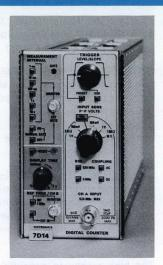
The 7D14 is a directly gated digital counter plug-in unit designed for use in all 7000-Series Oscilloscope mainframes except those without CRT READOUT. It will function in any plug-in compartment. The 7D14 has three modes of operation: Frequency—0 to 525 MHz, Frequency Ratio (A/B)—0 to 10<sup>5</sup>:1, and Totalize—0 to 10<sup>8</sup>.
