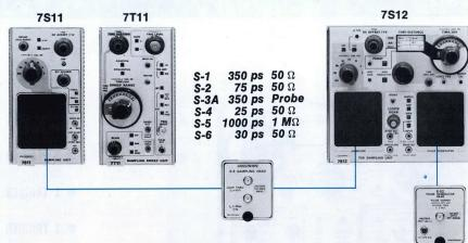
7S12-This unit features the flexibility of two plug-in heads for time domain reflectometry or general-purpose sampling. For TDR a sampling head, usually the S-6 feedthrough head, is used in one compartment. A pulse generator head is used in the other compartment as a pulse source. When the 7S12 is to be used as a general-purpose sampler, a trigger recognizer head is substituted for the pulse generator head.
