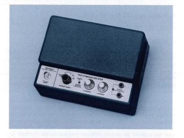
Indicator—Lamp indicates the presence of an output signal.
