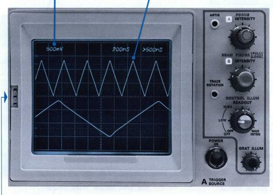
Three intensity controls allow independent adjustment of "A" sweep, "B" sweep, and READOUT brightness. When making measurements, you adjust the intensity of each sweep to the level that's best for your applications.
