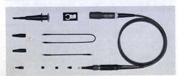
The P6052 is a passive dual-attenuation probe designed for TEKTRONIX low-frequency oscilloscopes that feature CF READOUT and trace-identification functions. A sliding collation the barrel of the probe selects 1X or 10X attenuation; a push button actuates the trace-identify function. A coding ring on the probe BNC output connector couples the control signals to the mainframe. The P6052 can be compensated for use with instruments having a nominal input capacitance of 15 to 55 pF.
