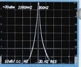
A signal at 1050 MHz showing the exceptional 30-Hz resolution band width capability of the 7L13. Note the CRT READOUT of center fre quency. (Mainframe 7904)
