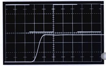
Upper display is a 60-Hz squarewave demonstrating the DC response of the P6042. The lower display is the same waveform at 10 ns/div. Double exposure photograph.
