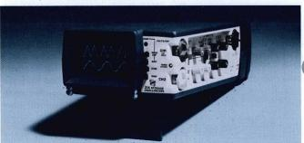
The 214 Storage Oscilloscope represents a breakthrough in portable oscilloscope design. It provides the same features as the 212: dual-trace, battery operation, rugged plastic case, and integral high-impedance probes. To these features, the 214 adds storage and single-sweep capabilities with no increase in either instrument size or weight. All of these features combine to make the 214 suitable for a wide range of installation and service applications.
