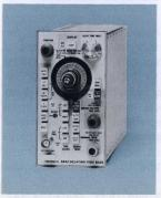
The 5B42 Dual Time Base is designed specifically for use with the 5403 Oscilloscope. It provides delayed sweep, triggering to 60 MHz, single-sweep operation, and calibrated sweep rates from 10 ns/DIV to 5 s/DIV.
