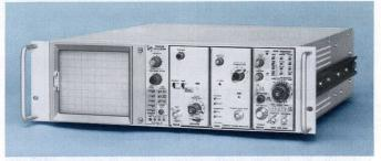
The R7403N requires only 51/4 inches of rack height in a standard 19-inch rack. It is fan-cooled and comes complete with slide-out chassis tracks.
