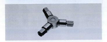
This coaxial tee is designed for use in broad-band,  $50-\Omega$ , systems where the mismatch introduced by ordinary "Tee" connectors is undesirable. Load isolation is nominally 6 dB while the voltage attenuation ratio is nominally 2X (input to either load arm, other load arm terminated in a standard  $50-\Omega$  termination). Maximum VSWR is 1.50 from DC to 12.00 GHz and 1.90 from 12.01 to 18.00 GHz. Power Divider SMA (3 MM)
