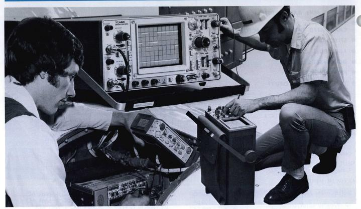
The purchase of a high-quality portable oscilloscope is an important investment. Thus, careful consideration must be given to your application or range of applications—present and future. The following are some areas to be considered when selecting a portable: (1) Measurement Capability; (2) Cost; (3) Size and Weight; (4) Durability; (5) Mobility; and (6) Battery and DC Operation.
