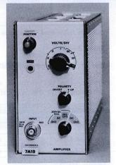
**Deflection Factor**— 10 mV/div to 1 V/div in 7 calibrated steps (1-2-5 sequence). Accuracy is within 3%.
