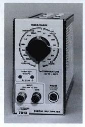
The 7D13 is a Digital Multimeter plug-in designed for use in all 7000-Series Oscilloscope mainframes except those without CRT READOUT. The 7D13 will function in any plug-in compartment.
