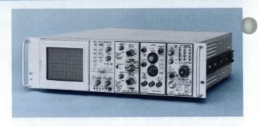
The R7313 requires only 51/4 inches of rack height in a standard 19-inch rack. It is fan-cooled and comes complete with slideout chassis tracks.
