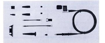
The P6053B is a miniature fast-rise 10X probe designed for TEKTRONIX instruments having a nominal input capacitance of 15 to 24 pF. The probe has a push button for actuating the trace-identify function of the oscilloscope mainframe and readout capability.
