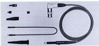
The P6049A is a miniaturized, 10X probe, for use with the 323, 324 and 326 Portable Oscilloscopes. The probes compensating box and cable is at right angles to the BNC connector to allow for compactness and easy use. The probe will compensate to oscilloscopes with input capacitance of 47 pF to 62 pF and input resistance of 1  $M\Omega_{\rm c}$
