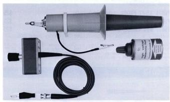
The P6015 provides 1000X attenuation for oscilloscope measurements up to 40-kV peak. Voltage or duty cycle derating is necessary for RF voltages at frequencies over 100 kHz, or in temperatures above 25°C.
