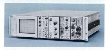
The R7903 requires only 51/4 inches of rack height in a standard 19-inch rack. It is fan-cooled and comes complete with slide-out chassis tracks.
