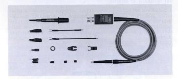
The P6048 is a low-capacitance, miniature probe designed for use with TEKTRONIX 100-MHz Oscilloscopes. It can also be compensated for use with other instruments that have a nominal input capacitance of 15 to 20 pF and inputs resistance of 1 M\Omega. The P6048 offers a new level of high-frequency measurement performance with its low 1-pF input capacitance. Its small size makes it easy to use, particularly for applications involving compact circuitry.
