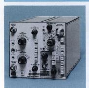
The 5S14N Dual-Trace Delayed Sweep Sampler unit brings low cost DC-to-1 GHz bandwidth to all 5000-Series Oscilloscopes. The two identical vertical channels provide dual-trace sampling at a sensitivity of 2 mV/div to 0.5 V/div. Five vertical display modes are provided with signal inverting capability in Channel 2.
