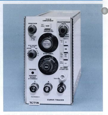
A front panel button switches the base/gate step generator output from current steps of the same polarity as the collector/drain sweep for checking transistors, to voltage steps of the opposite polarity of the collector/drain sweep for checking FETs in the depletion region. This button also internally switches the test fixture leads so that one test socket can be use to test both transistors and FETs.
