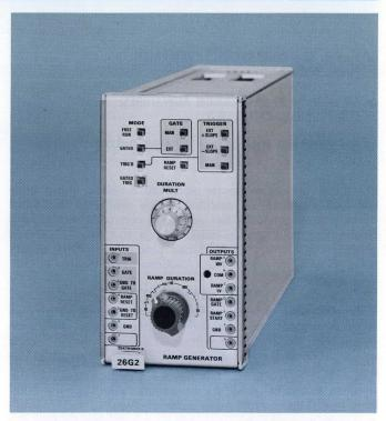
Ramp Reset-Terminates ramp and resets circuitry for generation of new ramp (locks out ramp until released).
