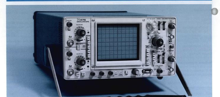
475 pictured above is identical in appearance to the 465 (not shown) except the 465 deletes the 0.01 and 0.02 μs TIME/DIV and 2 mV VOLTS/DIV switch positions.
