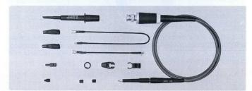
The P6012 is a miniature general-purpose probe designed for use with TEKTRONIX oscilloscopes having bandwidths up to 33 MHz. The probe can be compensated to match TEKTRONIX plug-ins and oscilloscopes with nominal input capacitances of 15 to 47 pF and input resistance of 1  $M\Omega$ .
