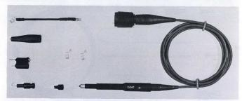
The P6056 is a miniature low-capacitance probe for use with 50  $\Omega$ , wide-band oscilloscopes. Bandwidth DC to 3.5 GHz. This probe can also be used with 50- $\Omega$  sampling systems, with an appropriate BNC adapter.
