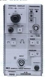
The M2 Sample/Hold Module in combination with the 7D12 measures voltage amplitude from ground to a selected point or the difference voltage between any two selected points (independent control of each point). The sample point(s) cabe triggered automatically, manually, or externally from sources such as: the oscilloscopes Delayed B Gate, the 7D15 Universal Counter/Timers Pseudo Gate, 7D11 Delayed Trigger Out, etc.
