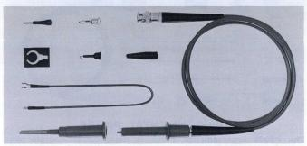
The P6028 is a general-purpose 1X voltage probe designed for use with TEKTRONIX oscilloscopes that have BNC input connectors. The P6027 is identical to the P6028 except for the UHF connector.
