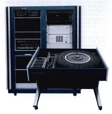
The TEKTRONIX S-3260 is an important, new automated test system. The results of years of test system design and manufacturing, it combines the most required test functions in a single product. The S-3260 is a major advance in state-of-the-art systems. It is built to perform GO NO-GO as well as engineering analysis testing of device measurements on all types of MOS, TTL, and ECL devices, circuit modules and printed circuit boards.
