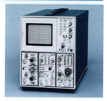
**Save**—Prevents erasing and storing additional displays, also extends viewing time of stored displays.
