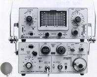
1401A-1 Portable Spectrum Analyzer shown with a 324 Option 76 Oscilloscope (P7 phosphor).
