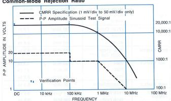
At least 2000:1, 10 mV/div to 50 mV/div (X10 Vc out) and 0.1 V/div to 5 V/div. AC Coupled input at least 500:1 at 60 Hz.
