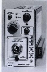
The 7S11 is a single-channel sampling unit for use in all 7000-Series mainframes. The input configuration employs the sampling "Plug-In Head" concept for maximum application range. The heads, which mount in the 7S11, cover a bandwidth from 350 MHz to 14 GHz. (See sampling head descriptions.)
