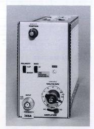
The 7A15A and 7A15AN are wideband plug-in amplifiers for all 10-Series mainframes. They feature constant bandwidth over the deflection factor settings. The two vertical mainframe channels allow the 7A15A/AN to be used alone, or with another vertical unit for dual-trace operation. Polarity of the display is
