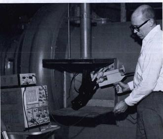
Typical application of the CT-5 clip-on high-current transformer, P6042 DC current probe and 7000-Series Oscilloscope measuring the running current of a 1500 hp delta-connected induction motor.
