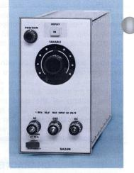
pickoff for basic measurements, and a built-in  $3\% \times 2\%$ -inch soldering pad matrix for use by the customer who wishes to build his own input circuits for special applications. Customerbuilt circuits are powered through the circuit board which provides access to all mainframe power supplies.
