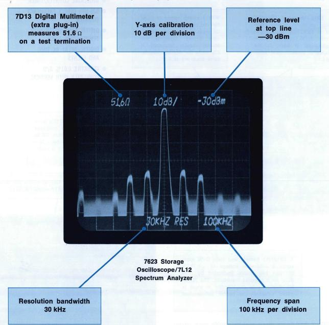
The photo above represents the high quality display a 7L12/7000-Series mainframe produces. The 7L12 combines with any 7000-Series mainframe to make an absolutely-calibrated spectrum analyzer.
