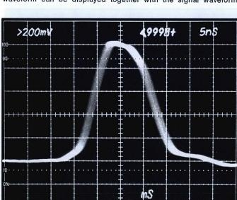
Fig. 1: 0.2  $\mu s$  time marker delayed 4.9998 ms by the 7D11 and displayed at 5 ns/div.
