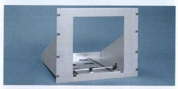
For rackmounting 500, 7500 and 7700-Series cabinet-type oscilloscopes in a standard 19-inch wide rack. Cradle mount consists of a cradle (or "shelf") without slide-out assemblies and a mask to fit over the regular instrument panel. 500-Series mask finish is blue vinyl, 7500 and 7700-Series mask finish is light gray.
