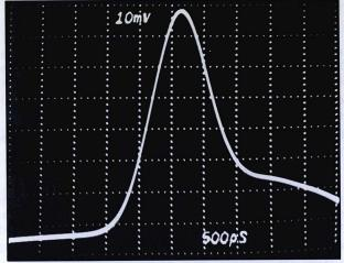
Fig. 1-TV display of one nanosecond wide impulse.
