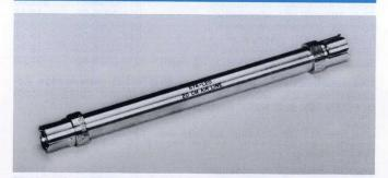
The 20-cm 50- $\Omega$  air line is useful as a time-delay device and as an absolute impedance in a time-domain reflectometer system. The characteristic impedance is 50  $\Omega$   $\pm$ 0.4%. Time delay is 0.6698 ns  $\pm$ 0.4%. 50- $\Omega$  Air Line 017-0084-00 \$22.00
