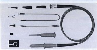
The P6060 is a precision passive probe with 10X attenuation, for use with TEKTRONIX low- and mid-frequency oscilloscopes used in differential applications. The precise attenuation also provides greater accuracy for single-ended input applications, such as amplitude measurements with a differential comparator. The probe can be compensated for use with any amplifier input having a nominal input capacitance of 15 to 55 pF and input resistance of 1  $\mbox{M}\Omega$ .
