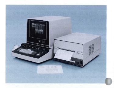
The 4601 Hard Copy Unit copies stored displays of the 4002A Graphic Computer Terminal and the 611 Storge Display Unit.
