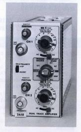
The 7A18/7A18N are dual-trace plug-in amplifiers for use with the 7000-Series mainframes. They are the basic building block for 3- or 4-trace operation. They feature constant bandwidth r all deflection factors, 5 operating modes (CH 1, CH 2, ALT, CHOP, ADD), trigger source selectivity and color-keyed control grouping. The trace IDENTIFY function is operative on 7A18 only. The 7A18N does not incorporate CRT READOUT, all other specifications are identical.
