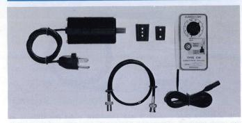
The 134 is used to extend the measurement capabilities of the P6021 or P6022 Current Probe. A CURRENT/DIV switch provides calibrated current steps from 1 mA/div to 1 A/div (with the oscilloscope or plug-in unit adjusted for a deflection factor of 50 mV/div).
