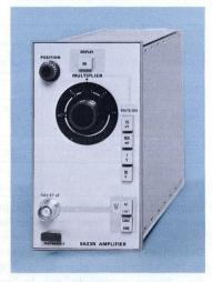
The 5A23N is a general-purpose amplifier for the 5000-Series Oscilloscopes. Featuring low cost and simplicity of controls, it is ideal for monitor and systems applications. It operates in the left or middle plug-in compartment of the 5000-Series mainframes for Y-T displays, or in the right compartment for X-Y displays.
