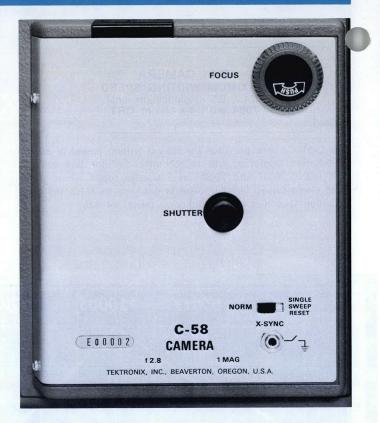
When the X-SYNC switch is in the SINGLE-SWEEP-RESET position, the shutter switch is connected via an adapter/beze connector to the sweep-reset line of a 7000-Series Oscilloscope. When the camera shutter opens, the shutter switch arms the oscilloscope sweep when it is in Single-Sweep Mode.
