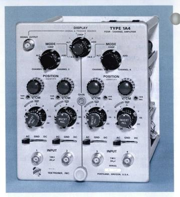
547, 549 and 556 Oscilloscopes. The front-panel output can also be cascaded with another channel, providing additional gain useful in many applications. Signal output amplitude is > 0.5 V/cm of display signal, unterminated at 1 kHz. Bandwidth is  $\leq$  20 Hz to  $\geq$  10 MHz (to approx 500 kHz with any channel operated in chopped mode). Approx 50- $\Omega$  output impedance.
