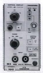
The M3 RMS Volts Module in combination with the 7D12 measures the true RMS voltage of signals from 40 Hz to 100 kHz. Voltages up to 1-kV peak can be measured while floating the input connectors.
