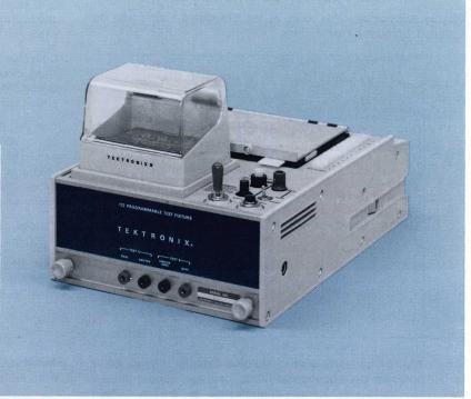
The 172 Programmable Test Fixture, when used with the TEK-TRONIX 576 Curve Tracer, permits the operator to program a sequence of tests on J FETs, transistors and diodes.
