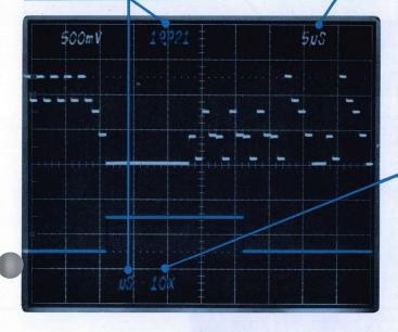
The 10X readout indicates the 7D15's measurement average. A range of averages in decade steps is available from 1X to 1000X. Increasing the averages by a factor of 10 increases the accuracy a factor of 10.
