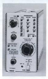
The 7B50 Time Base is recommended for use with the 7400, 7500, 7600 and Storage FAMILIES to provide bandwidth/sweep speed compatibility. However, it may be used in any 7000-Series mainframe. The 7B50 also has a horizontal amplifier input for uncalibrated X-axis deflection from an external source. The calibrated TIME/DIV range is from 5 ns/div. The 5 ns/div rate is obtained with the X10 MAGNIFIER.
