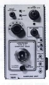
The 7S11 is a single-channel sampling unit for use in all 7000-Series mainframes. The input configuration employs the sampling "Plug-In Head" concept for maximum application range. The heads, which mount in the 7S11, cover a bandwidth from 350 MHz to 14 GHz. (See sampling head descriptions.)
