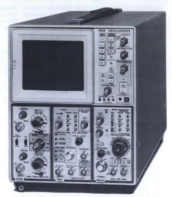
The TEKTRONIX 7633 Storage Oscilloscope provides 2200 div/ $\mu$ s (1000 cm/ $\mu$ s) stored writing speed and 100 MHz bandwidth. The instrument has three display modes: Stored, Nonstore and Save; and four storage modes: Bistable, Variable Persistence, Fast Bistable, and Fast Variable Persistence. The separate Reduced Scan selector is used, when needed, to get the top writing speed of 1000 cm/ $\mu$ s (using the center 8 x 10 reduced scan divisions, (.45 cm/div).
