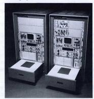
S-3110 and S-3111—designed to measure and test the performance of many types of active devices under simulated operating conditions. The systems are capable of testing such devices as diodes, transistors, integrated circuits, modules, and subassemblies. The systems will sequence up to 15 measurements in less than 150 ms.
