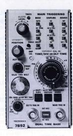
The 7B92 is recommended for use with the 7700 and 7900 FAMILIES. Its exceptionally fast sweep (500 ps/div) ideally matches the ultra-high bandwidth of the 7900 FAMILY and provides full bandwidth triggering for the 7700 FAMILY. Since the 7B92 uses only one horizontal compartment it permits usage of the other horizontal compartment for specialized measurements.
