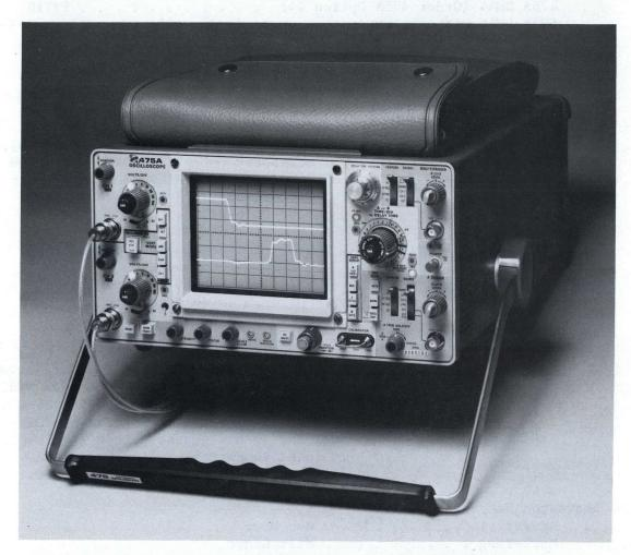
The 475A is an improved performance version of the 475 Portable Oscilloscope. It provides 250 MHz at 5 mV/div and a reduced spot size.
