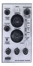
The 5CT1N Curve Tracer is a plug-in unit used in TEKTRONIX 5000-Series Oscilloscope systems for displaying characteristic curves of semiconductor devices to power levels up to 0.5 watts. The plug-in operates in either vertical deflection compartment of the mainframe. Horizontal deflection is achieved through a front panel source which drives the external input of either an amplifier or time base plug-in unit installed in the mainframe's horizontal deflection compartment.
