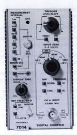
The 7D14 is a directly gated digital counter plug-in unit designed for use in all 7000-Series Oscilloscope mainframes except those without CRT READOUT. It will function in any plug-in compartment. The 7D14 has three modes of operation: Frequency—0 to 525 MHz, Frequency Ratio (A/B)—0 to 10<sup>5</sup>:1, and Totalize—0 to 10<sup>8</sup>.
