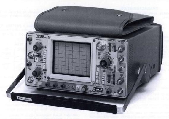
475 pictured above is identical in appearance to the 465 (not shown) except the 465 deletes the 0.01 and 0.02  $\mu$ s TIME/DIV and 2 mV VOLTS/DIV switch positions.
