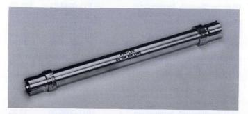
The 20-cm 50- $\Omega$  air line is useful as a time-delay device and as an absolute impedance in a time-domain reflectometer system. The characteristic impedance is 50  $\Omega$   $\pm$ 0.4%. Time delay is 0.6698 ns  $\pm$ 0.4%. 50- $\Omega$  Air Line 017-0084-00 \$26.00
