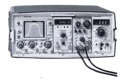
The Sweep System shown in the photograph includes SW 503 Option 1 Sweep Generator, DC 502 Option 7 Counter, SC 502 Oscilloscope, and DM 502 DMM in a TM 515 Power Module.
