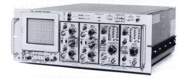
**Vertical Crossover**—Permits viewing the same signal on two time bases.
