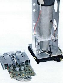
12KV post-accelerator crt and vertical system with delay line show high quality components and workmanship.
