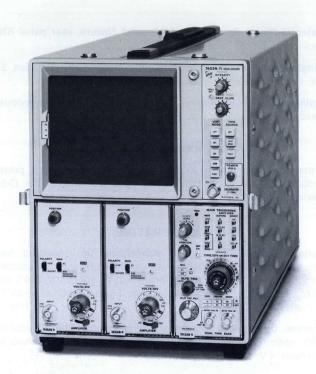
Shock (operating)—9 consecutive 400-pound hammer blows without failure from 1, 3 and 5 feet in vertical, horizontal, and longitudinal axis as per MIL-S-901 for Grade A, Class 1, Type A for lightweight equipment.
