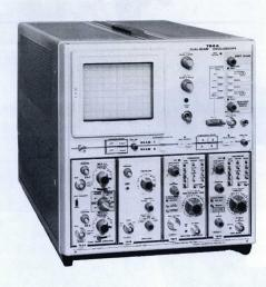
1 GHz using direct access). Unique features such as pulsed graticule and pulsed crt readout allow the pre- or post-photographic recording of important information such as vertical and horizontal scale factors, dates of tests, test number, and other pertinent data when recording single events.
