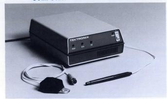
The TEKTRONIX 4953 and 4954 Graphic Tablets provide a convenient means for inputting graphics data to a computer, or onto the terminal screen, or into any other data system. The 4953 tablet is 11 x 11 inches while the 4954 offers a drawing-board sized tablet, 40 x 30 inches.
