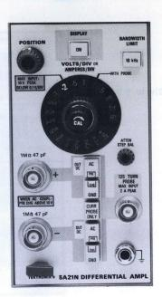
The 5A20N and 5A21N are 50  $\mu$ V/div, dc coupled differential amplifiers for the 5000-Series. The units are identical except that the 5A21N has a current probe input. Each plug-in is compatible with each compartment of the 5000 Series Mainframes.
