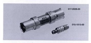
The coupling capacitor is a short length of coaxial line having a disc capacitor (4700 pF,  $\pm$ 20%) in series with the inner conductor. Reflection ratio (in 150-ps TDR system), maximum is 0.03. Voltage rating is 200 Volts.
