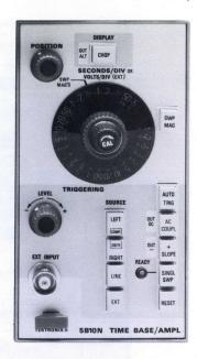
The 5B10N is a time base/amplifier plug-in unit for generating a sweep in the 5000-Series Oscilloscopes. An external input allows use of the 5B10N as a voltage amplifier with calibrated deflection factors of 50 mV/div and 500 mV/div.
