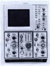
Crt readout provides quick on-screen reference of measurement parameters. And a selection of 30 different 7000-Series plugins permits 'custom-tailoring' the instrument to the job from the outset, and expansion of its capabilities as the needs arise.
