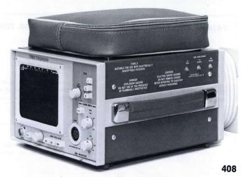
beats/minute. High limits must be continuous for 2 to 5 seconds for alarm. LOW RATE sets the lower limit between 15 and 150 beats/minute. For low-limit alarm, there must be two R-R intervals for excessive duration within 5 to 10 seconds of each other. Arrest alarm results when no beat is detected for approximately 6 seconds. Alarm may be reset by pressing the RESET push-button or turning off the low-rate control to the alarm-off position.
