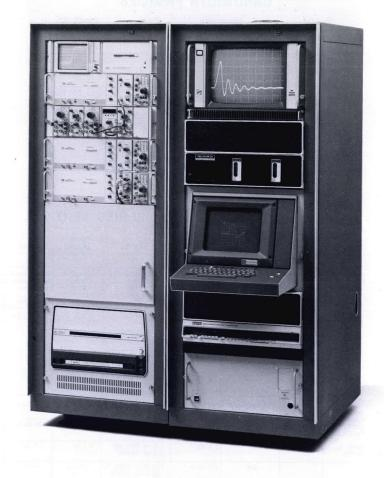
Up to four R7912's (one R7912 with 7A19 and 7B92 plug-ins is supplied).
