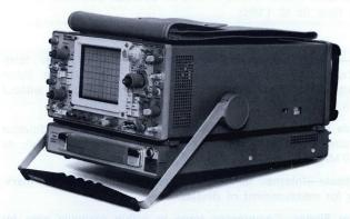
The 1106 is a convenient, snap-on battery power supply for TEKTRONIX 464, 465, 466, or 475 Option 7 Oscilloscopes.
