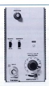
The 7A16A is a wideband plug-in amplifier for all 7000-Series mainframes. It features constant bandwidth over the deflection factor range of 5 mV/div to 5 V/div. Polarity of the display is selectable, as is bandwidth, which can be either FULL or limited to 20 MHz for low frequency applications.
