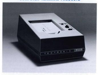
The 4623 Hard Copy Unit is designed to produce permanent, high quality, 8½ x 11-inch copies from the 4023 refreshed terminal. Four-channel input permits one 4623 to provide copies from up to four terminals. The first copy is produced in about 18 seconds, with additional copies of the same display taking about 8 seconds each.
