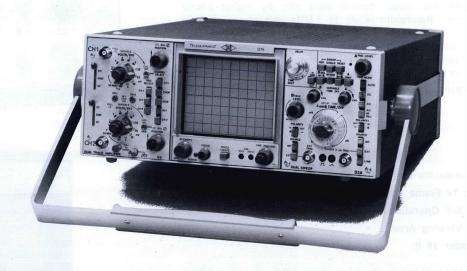
Portability and laboratory quality are combined in this 50-MHz Dual-Trace Oscilloscope for maximum utility in field service applications. Essentially a portable version of the D83, the D75 offers the same delayed and mixed sweep capability, 100 ns/div sweep rate (with X10 magnifier) and dual time base.
