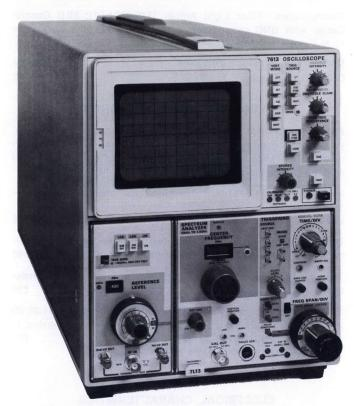
The 7L13 features 30 Hz resolution with less than 10 Hz of incidental FM (phase locked). The 7L13 is installed here in a 7613 variable persistence mainframe.
