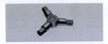
This coaxial tee is designed for use in broad-band,  $50-\Omega$ , systems where the mismatch introduced by ordinary "Tee" connectors is undesirable. Load isolation is nominally 6 dB while the voltage attenuation ratio is nominally 2X (input to either load arm, other load arm terminated in a standard  $50-\Omega$  termination). Maximum VSWR is 1.50 from dc to 12.00 GHz and 1.90 from 12.01 to 18.00 GHz. Power Divider SMA (3 MM) 015-1014-00 \$130.00
