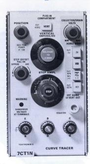
**Vertical Display Accuracy**—Within 5% in the X1 mode. Within 5%  $\pm 0.2$  nA per displayed horizontal volt when in the  $\pm 1000$  mode.
