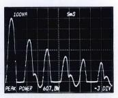
Power waveform resulting from multiplying current by voltage.
