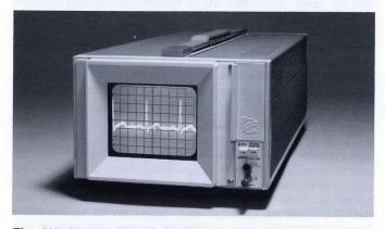
The 605 Storage Display Monitor features variable-persistence storage and X-Y-Z display capability. Simply turning a dial varies the length of time a waveform or image is held on the crt from a fraction of a second to more than 5 minutes.
