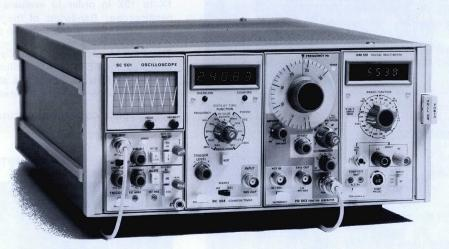
The TM 504 Power Module is a four-compartment mainframe for any combination of up to four TM 500-Series plug-in modules.
