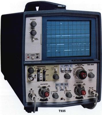
Dc to 35 MHz at 2mV/cm 10 ns/cm Sweep Rate (With 10X Sweep Expander) Delayed sweep (T935)
