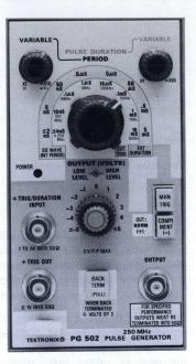
**Pulse Period**— 20 ns or less to 20 ms (within 5% from  $0.2~\mu s$  to 2 ms and within 15% at 20 ms) in decade steps. Continuously variable between steps and to at least 0.2~s.
