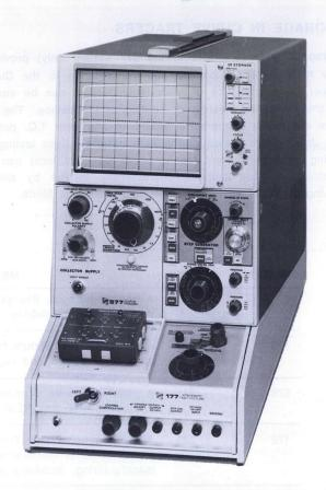
Offset—The amplitude of the entire set of steps can be offset in a continuously variable and calibrated manner to either AID or OPPOSE steps. Maximum range of offset is 10 full-amplitude steps.
