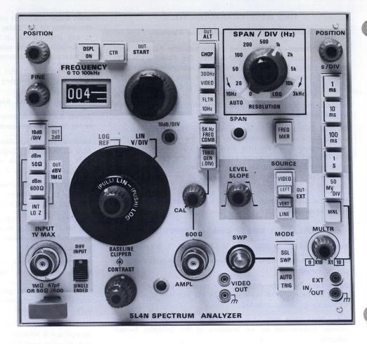
The new 5L4N is a low cost, high performance spectrum analyzer plug-in designed to operate over the frequency range 0 to 100 kHz. Accuracy is  $\pm$  3 kHz (fine tune control midrange and span/div calibrated for 10 kHz). Stability is within 100 Hz over a 1 hour period at a fixed ambient temperature.
