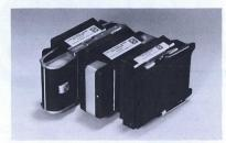
Three optional film backs allow a wide choice of films and provide flexibility of performance. Dark slides included with Polaroid Backs allow interchanging of all three films backs without exposing the film. Each Polaroid Back also includes a split-image focusing plate to allow optional image-type focusing if desired; the Graflok Back has an integral focusing screen and light shield.
