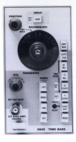
**Single Sweep—**Triggering requirements are the same as normal sweep. When triggered, sweep generator produces one sweep.
