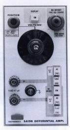
The 5A19N is a low cost differential amplifier featuring variable dc offset and simplicity of controls. It is ideal for monitor and systems applications and operates in the left or middle plug-in compartment of the 5000-Series mainframe for Y-T displays, or in the right compartment for X-Y displays.
