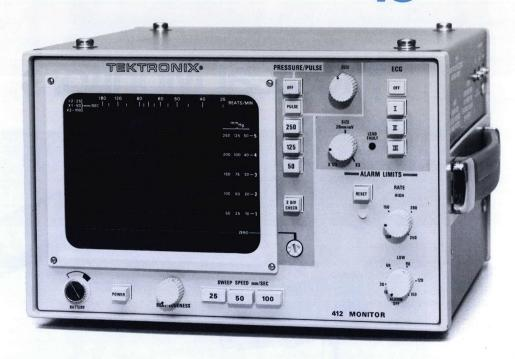
The 412 patient monitor provides either dual- or single-trace operation. In single-trace, ECG or pulse is centered on the large display screen. In dual-trace, the ECG trace is positioned in the upper display area while either pulse or pressure is displayed in the lower area. Pressure is always referenced to the ZERO line.
