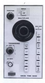
The 5B13N is a low-cost, general-purpose time base for the 5000-Series Oscilloscopes. Sweep rates are selected by push button. The 5B13N is for applications such as basic laboratory use by students, production testing, scientific research and other areas where 100 ms/div to 1  $\mu$ s/div sweep rates are needed.
