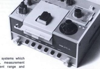
Curve Tracers are self-contained measurement systems which include power supplies, function generators, measurement circuitry and crt displays. Great measurement range and flexibility qualify Curve Tracers for evaluating and analyzing many different types of components. Curve Tracers also are powerful tools for in-circuit troubleshooting.
