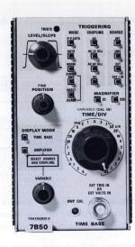
The 7B50 Time Base is recommended for use with the 7600 and Storage FAMILIES to provide bandwidth/sweep speed compatibility. However, it may be used in any 7000-Series mainframe. The 7B50 also has a horizontal amplifier input for uncalibrated X-axis deflection from an external source. The calibrated TIME/DIV range is from 5 ns/div. The 5 ns/div rate is obtained with the X10 MAGNIFIER.
