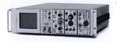
The R7313 requires only 51/4 inches of rack height in a standard 19-inch rack. It is fan-cooled and comes complete with slide-out chassis tracks.
