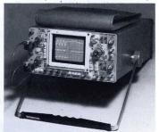
Its bandwidth is dc to at least 100 MHz within -3 dB. Using its X10 magnifier, the 466 achieves a 5-nsec/division sweep rate. Vertical deflection sensitivity is 5 mV/division.
