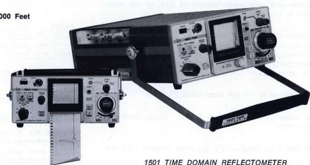
The 1501 is a portable, battery-operated Time Domain Reflectometer (TDR) used to detect and locate faults and to measure impedance variations in transmission cables through the use of test pulses. Resultant reflections from any discontinuities indicate the seriousness and character of the faults. The 1501 TDR is designed for use wherever communication or power transmission cable systems are used.
