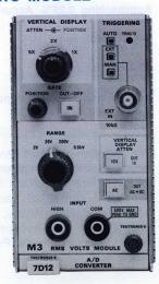
The M3 RMS Volts Module in combination with the 7D12 measures the true rms voltage of signals from 40 Hz to 100 kHz. Voltages up to 1-kV peak can be measured while floating the input connectors.
