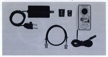
The 134 is used to extend the measurement capabilities of the P6021 or P6022 Current Probe. A CURRENT/DIV switch provides calibrated current steps from 1 mA/div to 1 A/div (with the oscilloscope or plug-in unit adjusted for a deflection factor of 50 mV/div). A passive termination is not required when using a 134 and a P6021 or P6022.
