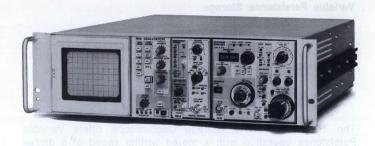
The R7613 requires only 51/4 inches of rack height in a standard 19-inch rack. It is fan-cooled and comes complete with slide-out chassis tracks.
