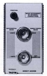
When used in 7900-FAMILY Oscilloscopes, vertical mode switching and CRT READOUT are inoperative, and the use of other plug-ins in the adjacent vertical channel is not possible.
