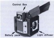
Provides automatic controlled film-fogging to increase writing speed by  $\approx 3$  times for 3000 ASA film and  $\approx 2$  times for 10,000 ASA film. For C-50, C-51, C-53, and C-59 only; not for C-52 and C-58. Please refer to page 246 for details.
