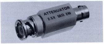
**Characteristics**—dc Resistance is 50  $\Omega$   $\pm$  1  $\Omega$ . Attenuation Accuracy is  $\pm$ 2% dc,  $\pm$ 5% at 2 GHz. Power rating (except 011-0099-00) is 2 watts average.
