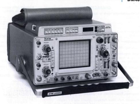
The DM40 or DM43 digital multimeter as part of a TEKTRONIX 464, 465, 466 or 475 provides a truly remarkable measurement package for field service. Both provide accurate differential time measurements between any two points on the display waveform, dc voltage measurements and resistance. Additionally, the DM43, with its included P6430 probe, provides direct-reading probe-tip temperature in °C.
