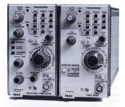
The 7B85/7B80 combination of plug-in time bases for the 7000 Series adds new capability in oscilloscope timing measurements—the time difference between selected points is computed and digitally displayed on the crt. Other features you'll like include 1 ns/div sweep rate, 400 MHz triggering, and variable trigger hold-off.
