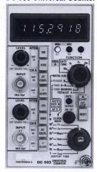
Counting to 100 MHz with six modes: frequency, period ratio, time A-B, time manual, and totalize. Period and ratio averaging for enhanced resolution. P 134.
