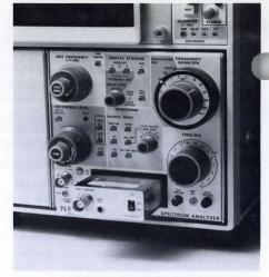
The 7L5 is shown with L1 50  $\Omega$  plug-in input impedance module.
