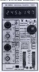
A 225 MHz universal counter offering seven modes: frequency of channel A signal, ratio of channel A to channel B frequency, period of channel B signal, time interval from channel A start to channel B stop, width of channel B pulse, events in channel A during B, and totalize. Time interval averaging with resolution to 100 picoseconds. Features dc trigger level output. P 135.
