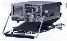
The SONY/TEKTRONIX 314 Portable Storage Oscilloscope provides dual trace storage with 4-hour viewing time and 1 mV/div sensitivity at 10 MHz, all in a compact, rugged package with less than one-half the weight of most other storage oscilloscopes.
