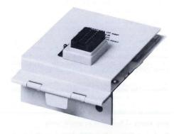
The Standard Op Amp Card is designed to test devices that require single or dual power supplies, have two (differential) high-impedance inputs, and a single output. Common measurements include: offset voltage, positive and negative input current, cmrr, gain, positive and negative psrr, positive and negative supply current, and collector supply current.
