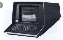
The 4006-1 Computer Display Terminal brings graphic display capability right to your desk top at a new low cost. The 11 inch storage tube provides crisp, clear displays with 800,000 viewable points (1024 X by 780 Y). It has an on-screen capacity of 2590 alphanumeric characters. You can transmit or receive data at selectable rates of 75 to 4800 baud.
