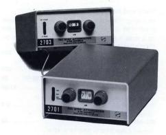
The 2701 and 2703 Step Attenuators are laboratory quality, bench top instruments for attenuation of large value radio frequency signals. The 2701 50  $\Omega$  Attenuator is particularly useful in making receiver sensitivity and distortion measurements. The range of attenuation is 0 to 79 dB, selected in 1 dB steps with tens and units cam swtiches.
