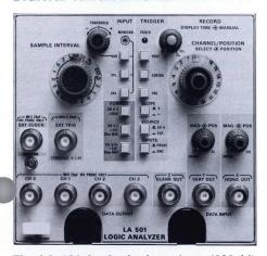
The LA 501 Logic Analyzer is a 4096 bit digital storage unit designed as a 2-wide TM 500 Series Plug-in providing flexible test package configurations for the engineering lab, manufacturing area, and field service applications.
