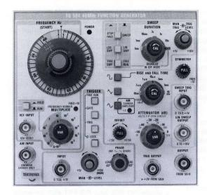
Frequency Range — Sine, Triangle and Square Waveforms: 0.001 Hz to 40 MHz calibrated range. Ramps, Pulses, or Waveforms requiring use of VARIABLE SYMMETRY control: 0.001 Hz to nominally 4 MHz. Multiplier switch has position for user — determined range by capacitor selection. Instrument shipped from factory with capacitor installed for 20 Hz to 20 kHz range.
