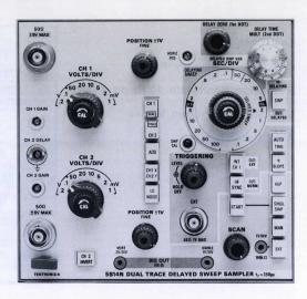
The 5S14N Sampling Unit combines amplifier and time-base functions in one double-width plug-in unit designed to operate in all 5000-Series Mainframes. Combining the Sampling amplifier and time-base functions in one plug-in enables the 5S14N to provide new economy and ease of operation.
