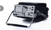
The SONY/TEKTRONIX 335 Portable Oscilloscope provides the fundamental capabilites (35 MHz bandwidth, dual traces, and delayed sweep) for a quite sophisticated level of digital and analog servicing. And these capabilities are housed in an easy-to-carry, 10.5 lb package. The 335 is ruggedly constructed to withstand the hard use of industrial and field applications.
