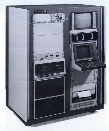
The WP2000-Series WDI analysis configurations are designed to acquire waveforms of transient phenomena and immediately perform full analyses. Other WDI analysis configurations include from 1 to 32 R7912 acquisition units, a controller (for waveform processing), a graphics terminal, a TV video or other monitor, a magnetic tape cassette, a disk or paper tape, and WDI TEK BASIC software.
