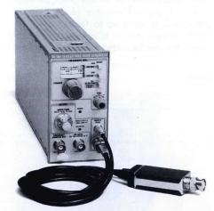
The SG 504 Leveled Sine Wave Generator is primarily intended to extend the capability of the TEKTRONIX Oscilloscope Calibration Package to 1050 MHz. It provides a constant amplitude sine-wave output over the frequency range of 245 MHz to 1050 MHz in two ranges. A reference frequency of either 50 kHz or 6 MHz (selected internally) is activated by a front-panel pushbutton, enabling you to quickly check the reference level setting without changing the dial.
