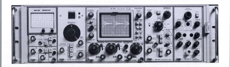
5 MHz Oscilloscope and 2 MHz Monitor
