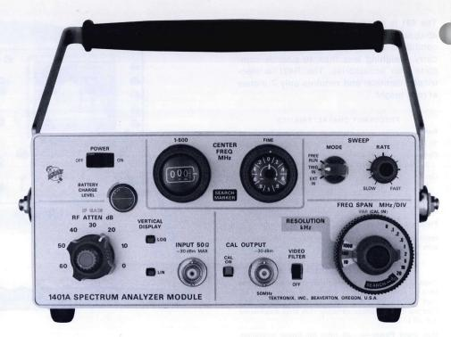
**Display Flatness** — Amplitude variations are within 1.5 dB to 200 MHz and 3 dB to 500 MHz.
