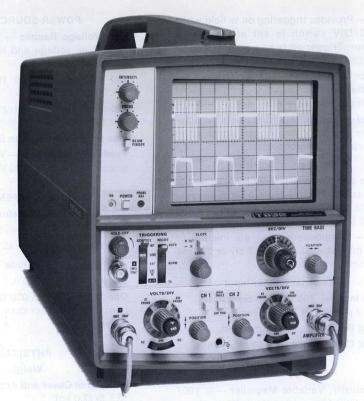
T932 35 MHz Single-Trace Oscilloscope
