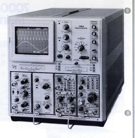
The 7904 and 5¼ in rackmount R7903 are the widest real-time-bandwidth, general-purpose oscilloscopes available today. The 7A19 Amplifier/7904 Mainframe attains 500 MHz at 10 mV. A 7A19 variable delay option allows for the matching of signal transit times of two plug-ins and their probes to better than 50 ps.
