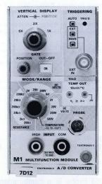
Temperature Mode 4½ Digit Crt Readout 100-μV Resolution Probe Measures Temperature or Voltage
