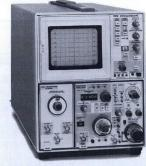
Fig 11. 7K11 Preamplifier Plug-in next to a 7L12 to Increase the Measurement Sensitivity.
