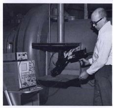
Typical application of the CT-5 clip-on high-current transformer, P6042 dc current probe and 7000-Series Oscilloscope measuring the running current of a 1500 hp delta-connected induction motor.
