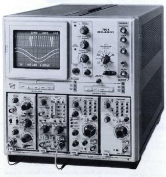
A high performance laboratory instrument system begins with the basic oscilloscope building block—the 7000-Series mainframe. Each mainframe consists of a bright cathode-ray tube, a power supply, electron beam deflection systems, and the switching circuitry necessary to integrate a versatile and complete measurement system.
