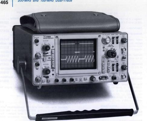
465 pictured above is identical in appearance to the 475 (not shown) except the 475 adds the 0.01 and 0.02 us TIME/DIV and 2 mV VOLTS/DIV switch positions.
