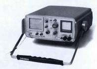
The 1502 and 1503 TDR Cable Testers are small, portable, rugged (qualifed to MIL-T-28800, Type 11, class 2, style A) battery-powered units designed to test any type cable, from lamp cord to coax, under virtually any conditions. The 1502 tests cables up to 2000 feet with resolution to a fraction of an inch, while the 1503 tests cables up to 50,000 feet with a resolution of 3 feet.
