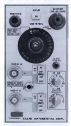
Dc-to-1 MHz Bandwidth 10  $\mu$ V/div to 5 V/div 100,000:1 Cmrr Selectable Upper and Lower -3 dB Points Dc Offset
