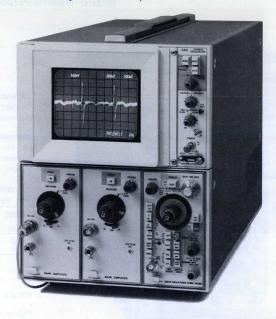
With the 5441 Variable Persistence Storage Oscilloscope, the length of time a waveform persists on the crt is continuously variable simply by turning a dial. View time at normal intensity can be varied from a fraction of a second to more than 5 minutes. In the save mode, signals can be viewed at lower intensity for up to an hour.
