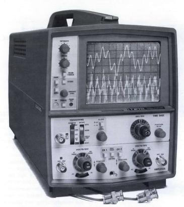
T912 10 MHz Oscilloscope with Storage
