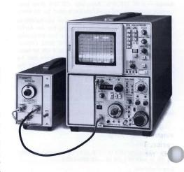
The 7L12 is shown in a 7613 Variable Persistence Mainframe connected to the AM-511 vhf preamplifier for extra sensitivity.
