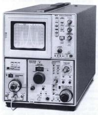
is normally part of a Tektronix Spectrum Analyzer. The flexibility and time savings normally realized with the modern analyzer, help make the analyzer less expensive, usually, than the crowd of older single purpose instruments.
