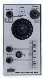
Dc-to-2 MHz Bandwidth 1 mV/div to 20 V/div Dc Offset The 5A19N is a low cost Differential Amplifier featuring variable dc offset and simplicity of controls. It is ideal for monitor and systems applications. It operates in the left or middle plug-in compartment of the 5000-Series Mainframe for Y-T displays, or in the right compartment for X-Y displays.
