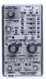
A 7000 Series Oscilloscope plug-in providing six counting modes: time interval, period, frequency (0 to 225 MHz), frequency ratio, totalize, and manual stop watch. p. 62.
