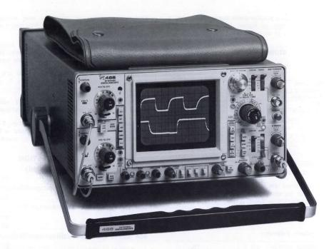
1350 cm/µs Stored Writing Speed (466) Dc to at Least 100 MHz Bandwidth 5 mV/div Vertical Sensitivity at Full Bandwidth
