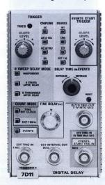
A 7000 Series Oscilloscope plug-in which provides a delay by events trigger by counting pulses from an external source or a delay by time trigger (selectable from 100 ns to 1 sec) by counting pulses from an internal clock. p. 58.
