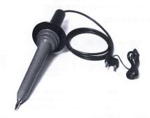
The High Voltage Probe will measure voltages from 1 kV to 40,000 volts with an accuracy of 1% at 25,000 volts. The division ratio is 1000:1. Common uses include measuring anode voltages on monitors or oscilloscopes.
