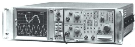
The R7603 requires only 5.25 inches of rack height in a standard 19 inch rack. It is fan cooled and comes complete with slide-out chassis tracks.
