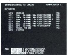
Pull POWER ON: A configuration menu appears describing all card modules in the DAS by slot number location. A sophisticated self-test verification is performed on each module with pass/fail indication. Bottom of screen indicates next step.
