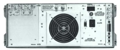
7612D rear panel: the GPIB connector and outputs for an X-Y-Z monitor (right); clock input/output, trigger inputs, and BNC connectors to feed signals to the front panel (left): remote power ON/OFF is also provided through the two central BNC connectors.
