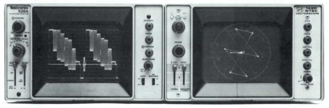
528A Waveform Monitor mounted side by side with a 1420 Vectorscope in optional rack adaptor.
