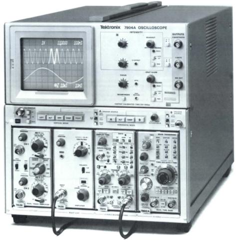
The 7904A and 5.25 inch rackmount R7903 are high bandwidth, general-purpose oscilloscopes. The 7A29 Amplifier/7904A Mainframe attains 500 MHz at 10 mV/div. A 7A29 variable delay option allows for the matching of signal transit times of two plug-ins and their probes to better than 50 ps.
