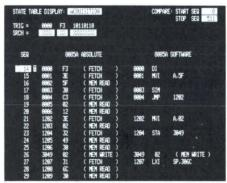
Press START SYSTEM: Data acquisition and pattern generator modules are simultaneously started. When a trigger occurs the DAS immediately defaults to the STATE TABLE format display with the trigger word clearly indicated on screen. Acquisition or pattern generator modules may be started separately by using the START ACQUISITION or START PAT GEN keys.
