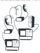
Master/Slave support is provided so that one 1240 (designated as Master) can completely control a remote 1240 (designated as Slave).
