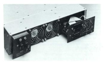
Modular construction and board exchange speed repair and minimize down time.
