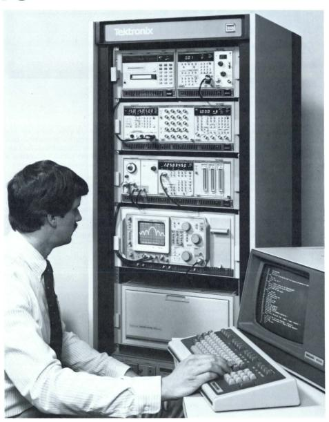
The DM 5010 Digital Multimeter measures dc and true RMS ac volts, ohms, and provides a diode test function. Internal math capabilities include averaging, nulling, offset, scaling, dB, and HI/LO/Pass sorting.
