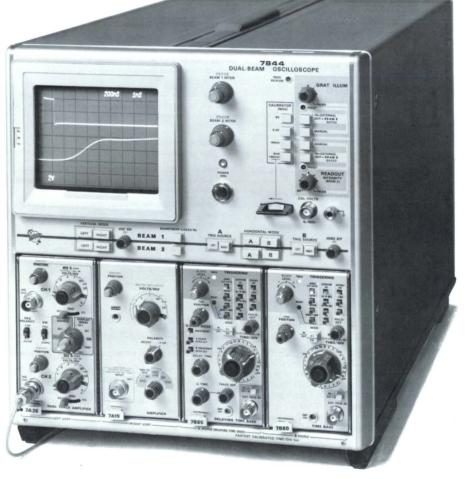
Beam Finder (Beam 1 and Beam 2, Independent Controls) - Limits display within graticule area and intensifies beam.
