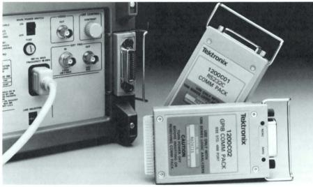
Figure 12.1240 with COMM Pack inserted
