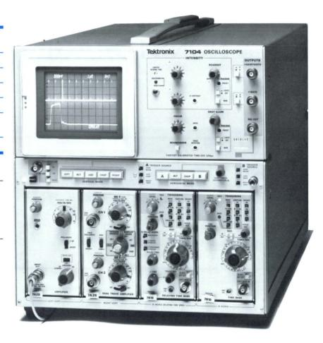
With its sweep speed of 200 ps/div, the 7104 clearly shows a single-shot, 350-ps step, six divisions in amplitude.
