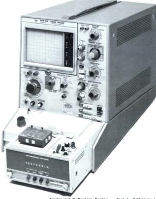
The 172 Programmable Test Fixture, when used with the Tektronix 576 Curve Tracer, permits the operator to program a sequence of tests of J FETs, transistors, and diodes.
