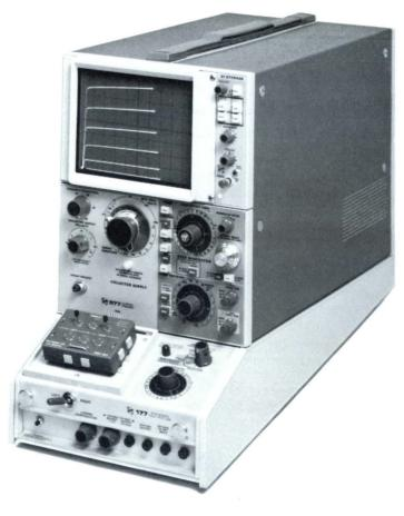
The 577 Curve Tracer System, when used with the 177 Standard Test Fixture, is a smaller and lighter configuration that retains many of the important features and performance of the 576. The 577 also accepts the 178 Linear IC Test Fixture. The major features that separate the 577 from the 576 are a storage CRT and the emphasis on low current measurements with the 577.
