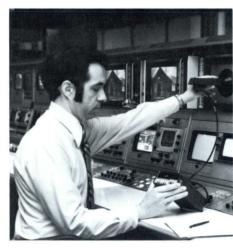
J16-TV System being used for color monitor setup.
