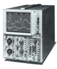
5D10 and 5A26 installed in a 5110 Mainframe
