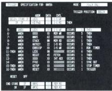
Press TRIGGER SPEC: Use CURSOR SELECT key to scroll through all possible triggering combinations of data acquisition modules, including "ARMS MODE". The 91A24's five word recognizers with 16-level stack are shown. Address and control fields symbolically display labels and control functions.
