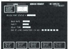
Figure 13. COMM Port Control menu with a 1200C01 RS-232C COMM Pack installed.
