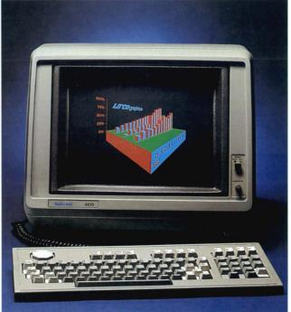
The 4105 is designed to produce complex graphics and pictures and perform the text editing tasks required by professionals in day-to-day data analysis and representation. As a result, it can also easily handle the simple bar graphs and pie charts and block diagrams normally required by business and management. Display courtesy of Integrated Software Systems Corporation. See page 98.
