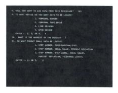
4052A Graphics Computer Controller showing the development of a typical calibration procedure using the ScopeCal Procedure Development Aid program
