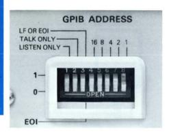
Each GPIB instrument or peripheral, called a device, must be assigned a different system address; this can be done simply by setting switches, usually located on the back panel of the device.
