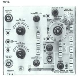
**Dual Trace Delayed Sweep Sampler**
