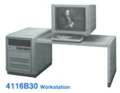
The 4116B can be configured either as a pedestal unit with detached low profile keyboard or in separate display, processing, and keyboard modules for flexibility in configuring workstations (4116B30).
