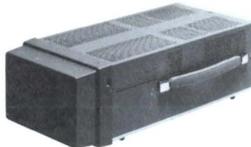
A snap-on front cover, molded of high impact plastic, is available for the TM 503 (shown above), TM 504, and TM 506 mainframes. The cover adds 45 mm (1.75 in) to the length of the TM 503, TM 504, and TM 506 mainframes, and clears the longest knob projections on any of the instruments.
