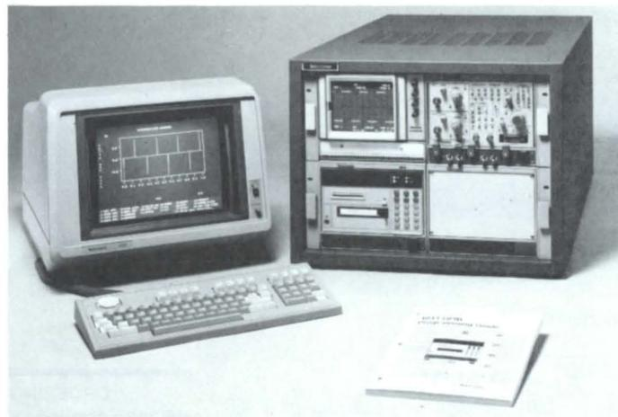
The MP 2401 Measurement Package consists of a display monitor, 7D20T, 4041, and 4105.
