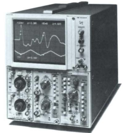
5D10 and 5A26 installed in a 5110 mainframe
