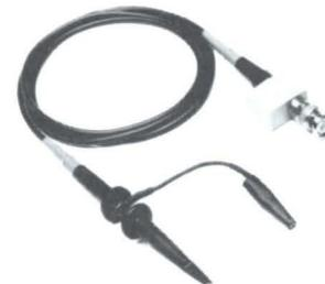
The P6125 is a low-capacitance, 5X attenuation passive probe specially designed for use with counter/timers. It makes possible more accurate time interval measurements of high speed logic signals. Five-times attenuation provides an optimum match between the counter input characteristics and the voltage levels of all common logic families. The low input capacitance permits acquisition of high frequency signals with minimum loading of the circuits under test.
