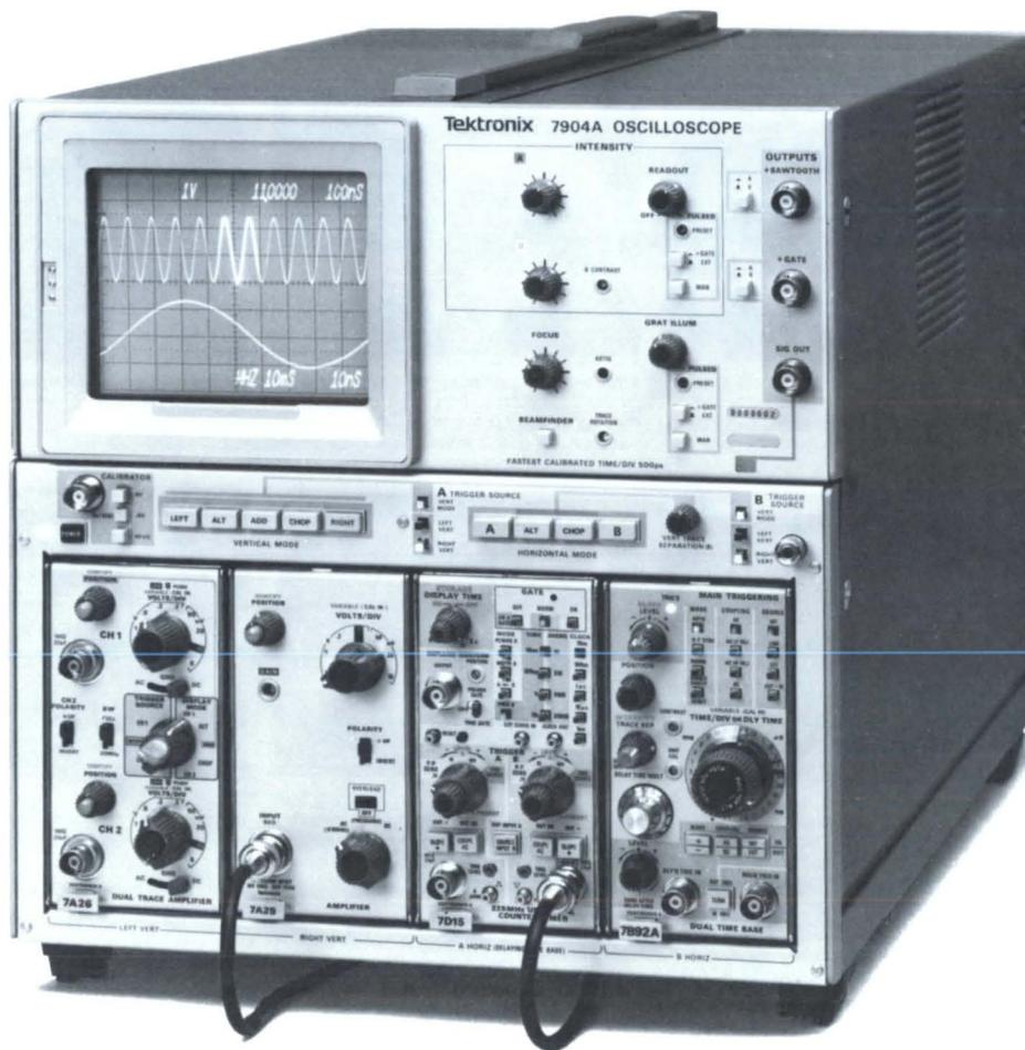
The 7904A and 5.25 inch rackmount R7903 are high bandwidth, general-purpose oscilloscopes. The 7A29 Amplifier/7904A mainframe attains 500 MHz at 10 mV/div. A 7A29 variable delay option allows for the matching of signal transit times of two plug-ins and their probes to better than 50 ps.
