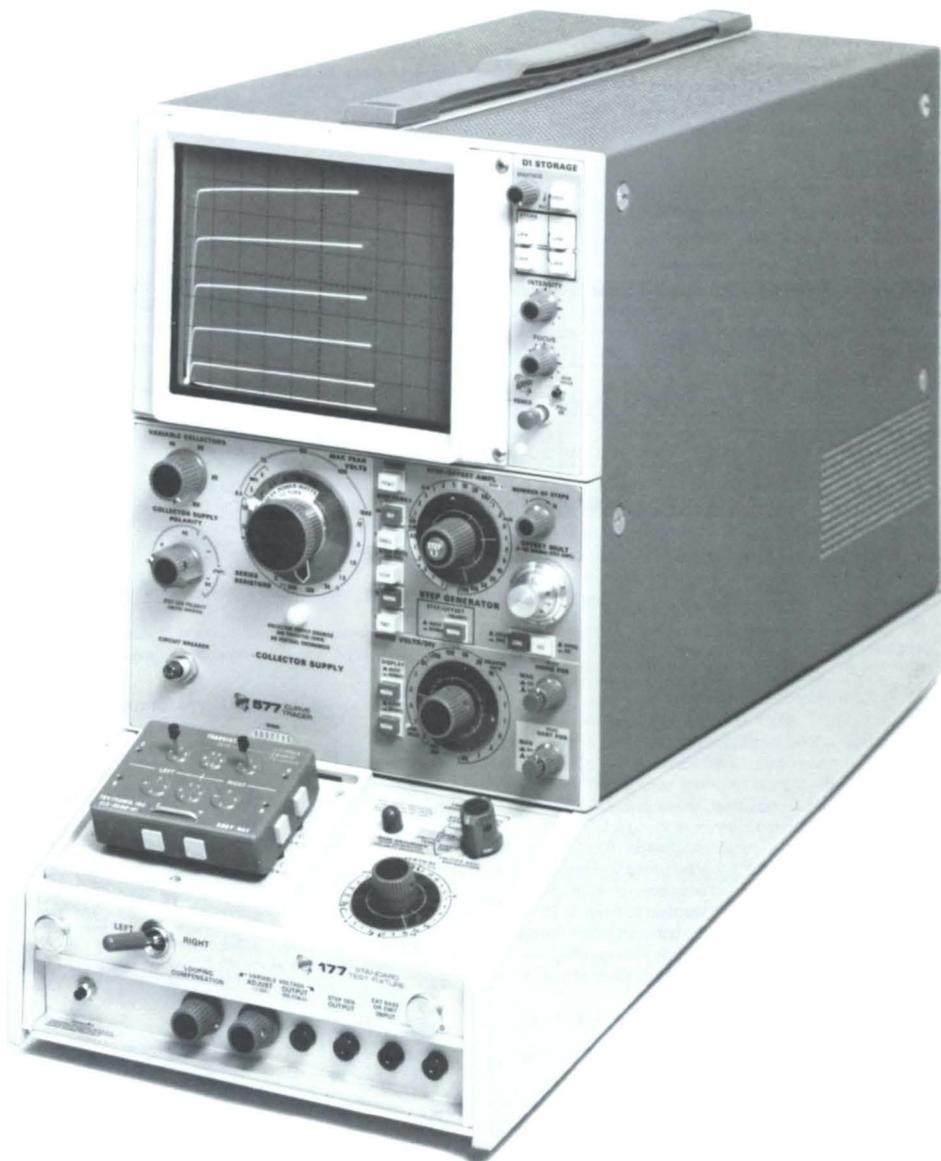
The 577 Curve Tracer System, when used with the 177 Standard Test Fixture, is a smaller and lighter configuration that retains many of the important features and performance of the 576. The 577 also accepts the 178 Linear IC Test Fixture. The major features that separate the 577 from the 576 are a storage CRT (optional) and the emphasis on low current measurements with the 577.
