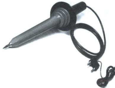
The High Voltage Probe will measure dc voltages from 1 kV to 40 kV with an accuracy of 1% at 25 kV. The division ratio is 1000:1. Common uses include measuring anode voltages on monitors or oscilloscopes. Probe plugs directly into the front end of the multimeter.
