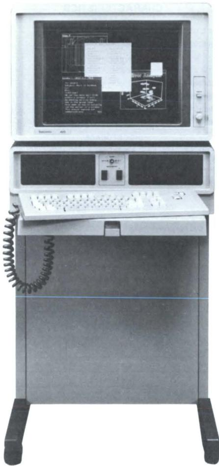
*Pedestal Configuration: Display shows new 4115P51 feature enhancement which enables efficient implementation of host-based window management functions.*
