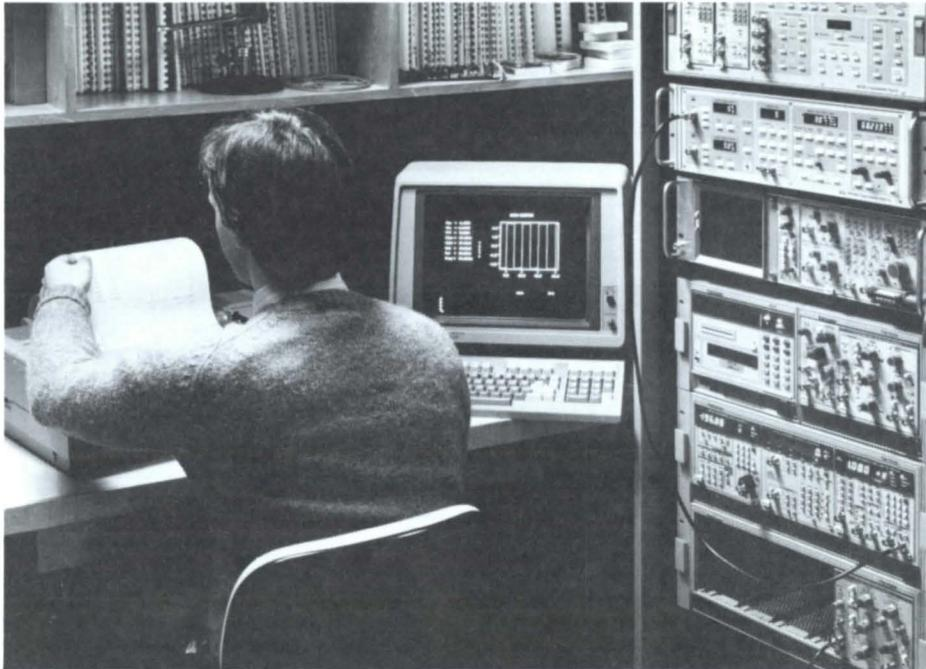
Figure 5. The 390AD can be easily integrated into wide range of GPIB systems. Shown above is a 4695 Color Hard Copy Unit and a 4105 Color Terminal which is connected to a Tektronix 4041 System Controller.
