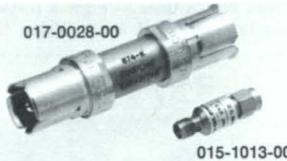
The coupling capacitor is a short length of coaxial line with a disk capacitor (4700 pF, ± 20%) in series with the inner conductor. Reflection ratio (in 150 ps tdr system), is 0.03 maximum. Voltage rating is 200 V.
