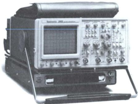
The 1106 with attachment kit fits under the base of a scope. The 1107 attaches with kit to the rear of a scope.
