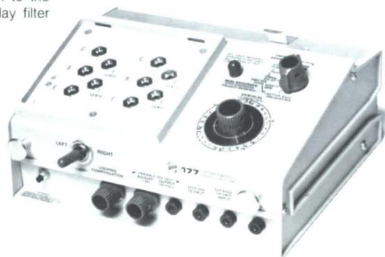
Other innovations in the 577/177 Curve Tracer are an emitter-base breakdown position on the lead selector switch, availability of approximately 95 steps from the step generator, an uncalibrated bias supply, independent magnifiers that increase resolution on either or both CRT axes, and a beam finder.
