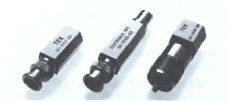
75  $\Omega$  termination. 75  $\Omega$  within 0.2% (at dc). Return loss is  $>52$  dB, dc to 10 MHz, maximum input voltage is 5 V RMS, center conductor to ground.
