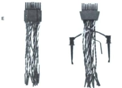
**K. Pattern Generator Lead Set** — 10 + 6 wide comb with VH and VL Pomona Hook Tips, 9 inch, twisted pairs, color coded, connects to 0.025 inch square pins, grabber tips not included.
