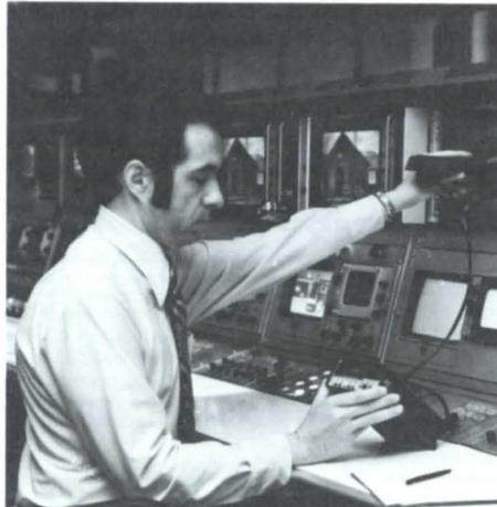
J16-TV System being used for color monitor setup.
