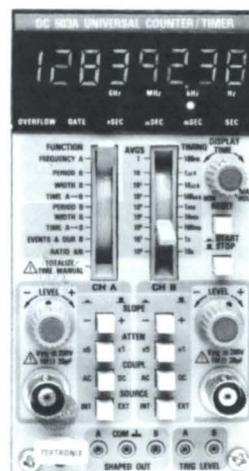
The DC 503A can be equipped with an optional temperature controlled 10 MHz crystal oscillator (Option 01) to obtain a highly stable and precise internal time base. Both the optional oscillator and the standard 10 MHz crystal oscillator provide 100 ns resolution of single-shot time intervals.
