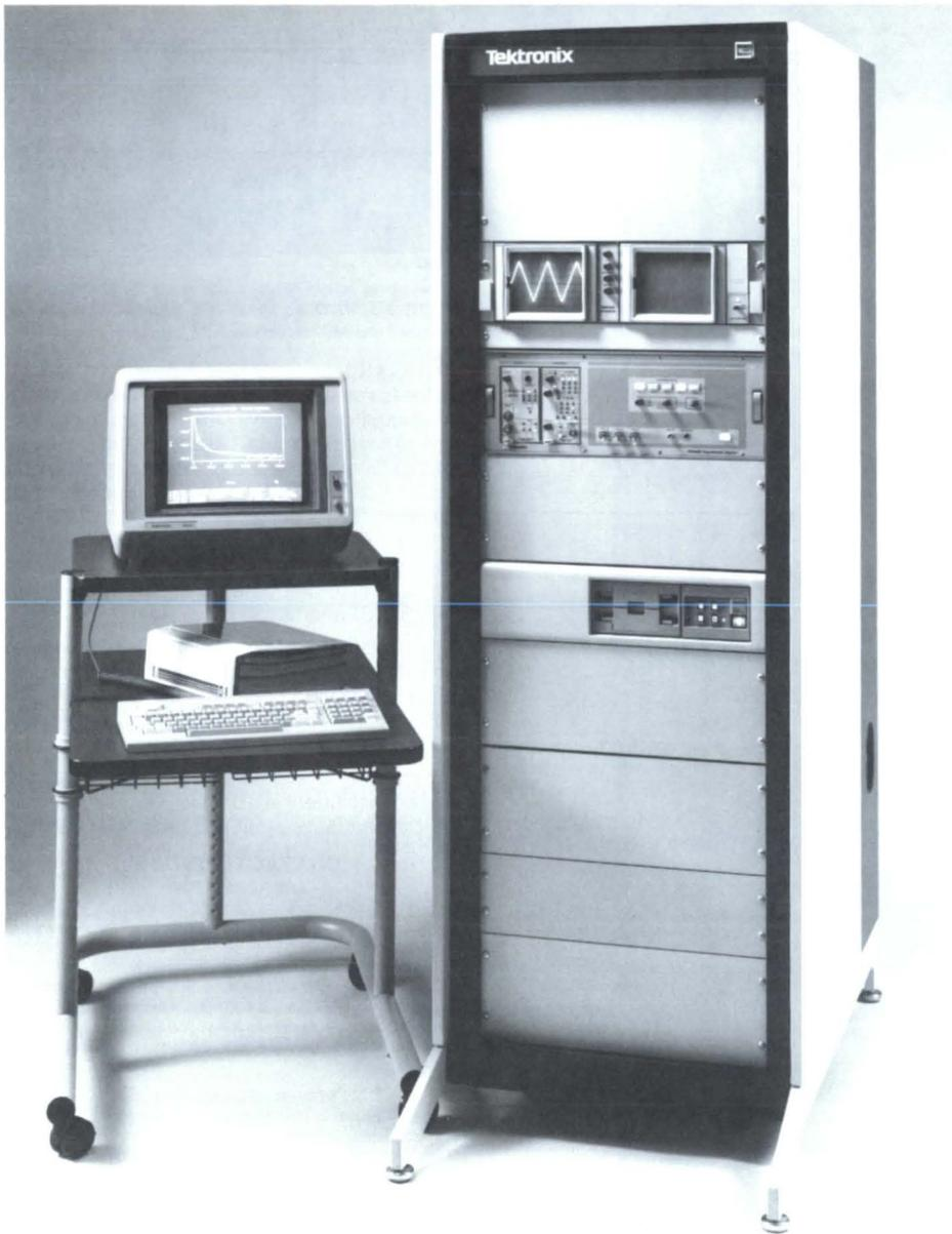
Shown above is the MS 3101. The MS 3201 replaces the 7912AD Programmable Digitizer with a 7612D Programmable Waveform Digitizer (see inset). Cart not included.\*\*
