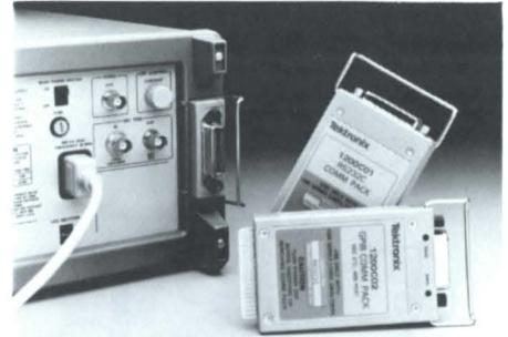
The printer interface consists of the combination of a ROM Pack and a COMM Pack. The 12RC01 Printer Support ROM Pack is used in combination with either the 1200C01 RS-232C COMM Pack (for printers with a serial interface) or the 1200C11 Parallel Printer COMM Pack (for printers with a parallel interface).
