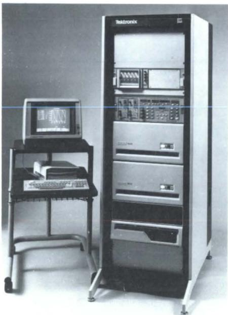
*Tektronix MS 4201 Acquisition/Processing Measurement System using TEK SPS BASIC and a DEC PDP-11 Minicomputer.*
