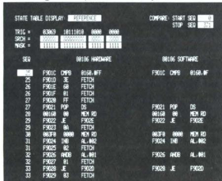
A State Table Display illustrating 80186 EDM Disassembly in hardware and software format.
