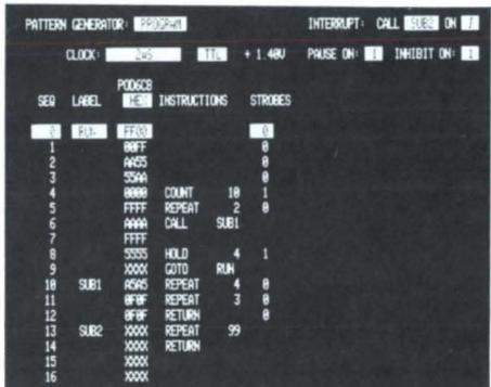
**Press PATTERN GENERATOR:** This menu allows you to construct a pattern generation program 254 lines deep using English-language like commands. Labels may be used to identify program segments and can be called from the main program providing sophisticated patterns for the debug of hardware or software.
