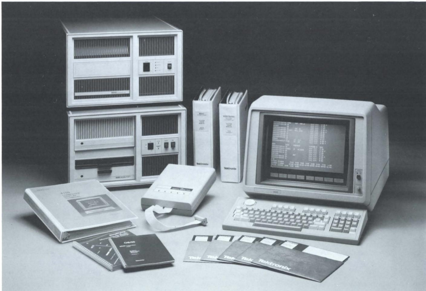
These systems consist of assembler, emulator, probe and firmware, 8561 Multiuser Software Development Unit, 4105 Color Graphics terminal and 8540 Integration Unit with 64 kbytes of memory.
