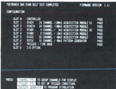
**Pull POWER ON:** A configuration menu appears describing all card modules in the DAS by slot number location. A sophisticated self-test verification is performed on each module with pass/fail indication. Bottom of screen indicates next step.
