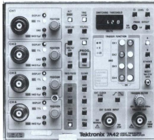
The 7A42 Logic Triggered Vertical Amplifier is a two-wide 7000 Series plug-in that provides a significant new dimension to oscilloscope measurements through the combination of oscilloscope and logic analyzer technologies. The 7A42 logic triggering permits digital signals to be displayed in analog form for high resolution measurements of both time and amplitude characteristics.
