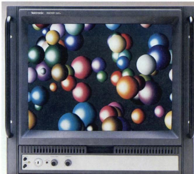
*The photograph of a 690SR screen shows the image created by an experimental system which uses dither to decrease edge effects and contouring allowing minimization of the size of the image memory. See page 186.*
