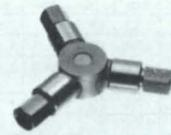
This coaxial tee is designed for use in broad-band 50 Ω systems where the mismatch introduced by ordinary "Tee" connectors is undesirable. Load isolation is nominally 6 dB while the voltage attenuation ratio is nominally 2X (input to either load arm, other load arm terminated in a standard 50 Ω termination). Maximum vswr is 1.50 from dc to 12.00 GHz and 1.90 from 12.01 to 18.00 GHz.
