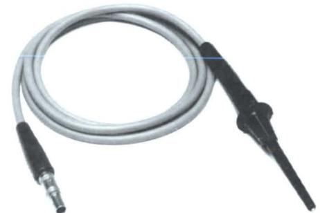
The P6601 Probe is a temperature measuring device designed to operate with the DM 502A and DM 501A Digital Multimeters. The temperature sensing element consists of a thin-film platinum resistor on the tip of the probe. Measurements are made by touching the probe tip to the surface whose temperature is in question. The thermal signal is transmitted to the associated digital multimeter through a two-conductor cable.
