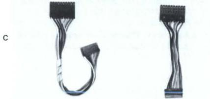
**I. Harmonica Lead Set** — 10 wide comb to 10 position single row connector, for 0.025 inch square pins on 0.1 inch centers, 5 inch, color coded.
