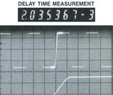
Figure 5. Delay time is measured from the start of the A sweep to the start of the intensified zone.
