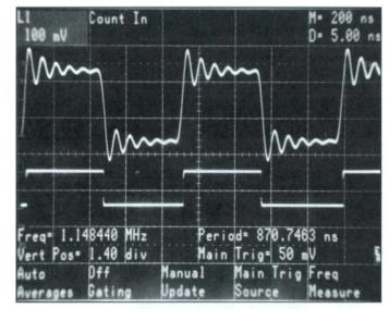
Here the Count In trace (lower trace) shows that the counter/timer is being properly triggered for the desired measurement.
