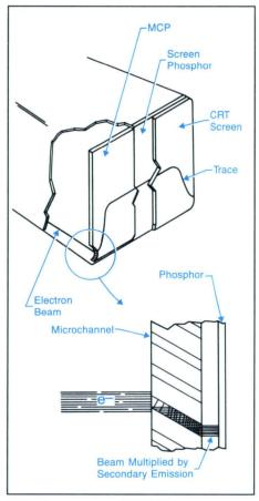
Microchannel-plate (MCP) CRT configuration.
