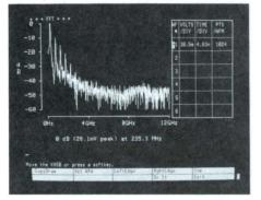
Computing and displaying frequency-domain data using an HP Series 200 Controller and Tek 7854 or 7D20 digitizing oscilloscope.
