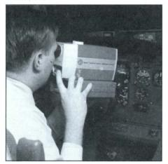
Measuring Luminance with the Tektronix J16/J6523.
