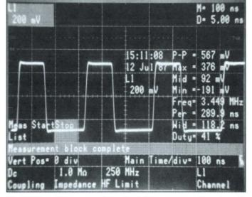
The 11300 oscilloscopes make up to eight measurements, automatically, on the selected signal.
