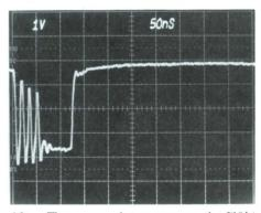
After—The same pulse as seen on the 7104/ R7103 readily indicates that the problem is input-signal bounce.
