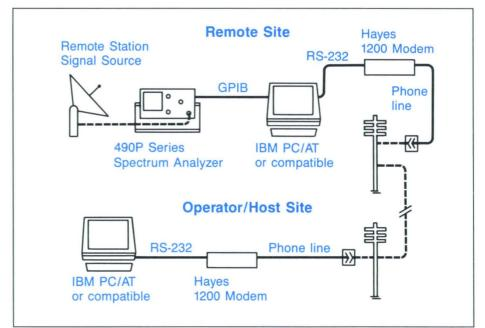
Equipment setup for remote site signal monitoring.
