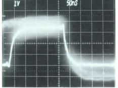
Before—A pulse train on a TEK 7904A doesn't reveal the low-level glitch occurring every tenthousandth pulse. (The TEK 7904A was previously the world's fastest writing-rate scope.)
