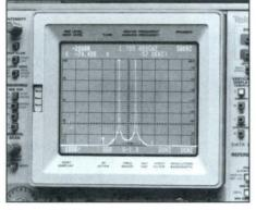
$\label{eq:last_constraint} Intermodulation\ measurement\ using\ alternate\ CRT.$
