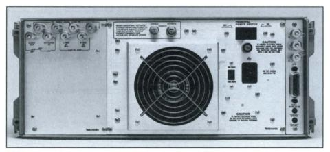
7612D rear panel: the GPIB connector and outputs for an XYZ monitor (right); clock input/output, trigger inputs, and BNC connectors to feed signals to the front panel (left); remote power ON/OFF is also provided through the two central BNC connectors.
