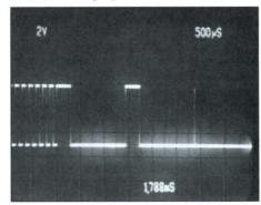
Glitch Capture—The 7934 captures a glitch (near the 8th) using a 7A29 plug-in and variable-persistence storage.
