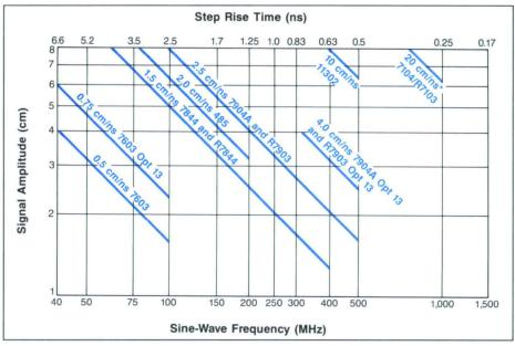
Amplitude vs speed and photographic writing rate comparison of 7000-Series mainframes using BE (P11) phosphors (Option 78), 20,000 ASA film, and the C-51 (f/1.2, 1:0.5) Camera.
