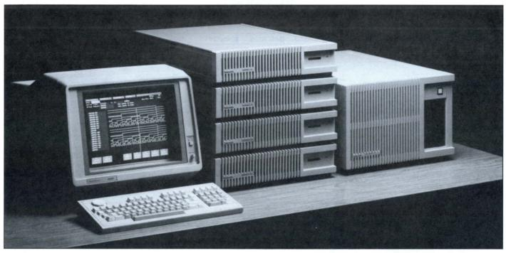
Fastest digital analysis system in the world-DAS 9219 mainframe and color display with four 8-channel, 2 GHz 92HS8 modules.
