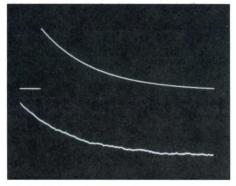
The initial portion of an exponential decay is recorded on Channel A (top trace); Channel B, set at a higher sensitivity and triggered to record after Channel A has finished, captures the remaining pulse tail with increased vertical resolution (bottom trace).
