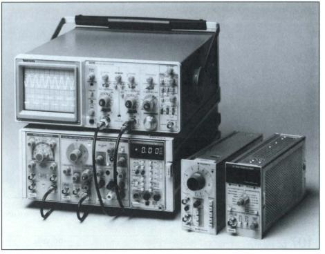
Intermediate Lab Station with optional plug-ins.
