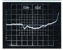
Comparison of the line distortion of the 92HS8 probe attached to a nominal 500- $\Omega$  test point on an ECL-based circuit (top), versus that of a typical 100-MHz probe.
