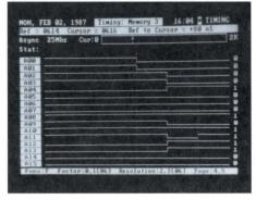
Timing Diagram. Use the reference cursor to measure pulse widths or the time between edges.
