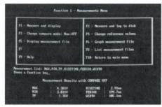
Interaction with the software is simplified through the use of function-key-driven menus as shown above in the Measurement menu.
