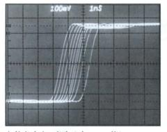
A digital circuit that shows no jitter on a conventional oscilloscope is found to have a 2.0-ns jitter when viewed with the distinct imageviewing capability of the 7104/R7103.
