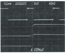
With the mainframe still selecting Alt sweeps, delaying and both delayed sweeps are shown. The digital readout on the lower CRT edge shows the time between the two sweep delays. The Trace Separation knob is used to position the second delayed sweep below the first delayed sweep with up to three divisions of separation.
