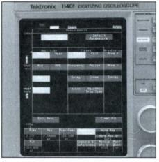
The 11401 and 11402 perform a wide range of amplitude, timing, and area/energy measurements. The measurements are automatic, accurate, easily accessible and clearly annotated for repeatable results.
