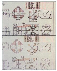
Graphics printing with (top) and without (bottom) the Tektronix 4510A Rasterizer.
