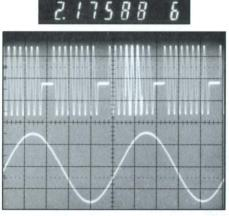
Figure 1. With the B sweep triggered, the frequency within the intensified zone on the A sweep is measured.
