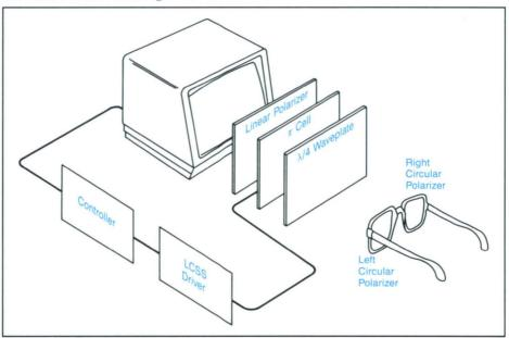
Liquid-crystal, field-sequential stereoscopic display. To view a Tek LCSS display system, the user wears glasses that are much like polarized sunglasses. Unlike user-worn devices in other field-sequential systems, these glasses do not restrict head movement or position. The viewer, wearing these glasses, can look elsewhere without restriction. Users are not tethered or harnessed to the 3-D system.
