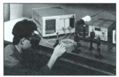
Optical waveform characterization is now much easier to do with the P6701 and P6702 Optical to Electrical Converters. The signals converted by these optical probes are then easily analyzed with the 11000-Series display and measurement system. See Accessories section for more information.
