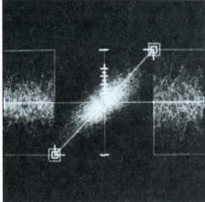
Live audio, left and right channels, time versus amplitude sweep display, and Lissajous pattern (center) with correct stereo phase.
