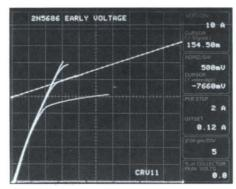
F-line cursor used to calculate and display early voltage (-7.66 V).
