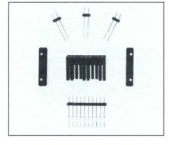
C. Circuit Board Mounted Probe Connector Kit—10+6-wide comb to 0.025-inch square pins on 0.15-inch centers, with mounting tabs, for PC mounting, mounting hole dimensions 0.80 inch wide X0.95 inch long. Interfaces to the following probes: P6452, P6455, P6456, P6457, P6460, and P6462. Seven piece kit. Order 020-1027-00
