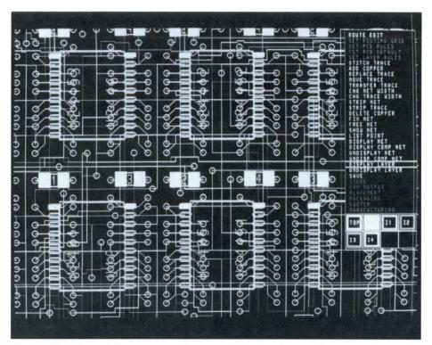
The PCB WorkSystem fully supports surface mount technology by providing color-coded graphic representation of components on top and bottom surfaces of the board.
