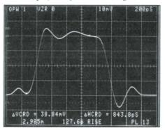
Digital-Storage 7854. Here, the 7854 measures the 127.6-ps rise time of a 38.83-mV pulse displayed at a sweep speed of 200 ps/div.
