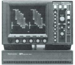
1740 Waveform/Vector Monitors with optional carrying case and battery pack.
