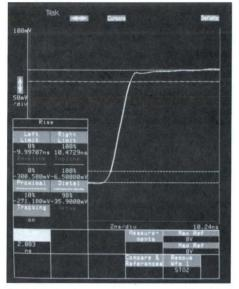
High bandwidth allows capture and measurement of fast rise times. Measurements can be customized and annotated to clearly show where and how the measurement is being made.
