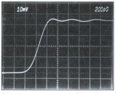
With its sweep speed of 200 ps/div, the 7104/R7103 clearly shows a single-shot, 350-ps step, five divisions in amplitude.
