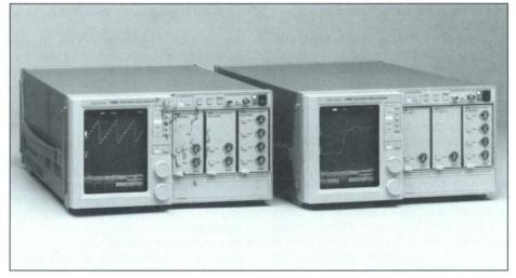
The 11401 and 11402 are the first in a line of high bandwidth, programmable digitizing oscilloscopes. The 11401/11402 are ideal for digitizing and accurately measuring repetitive waveforms. 10–14 bit vertical resolution, 20 MS's A/D conversion system provides a cost-effective solution to a wide range of measurement problems.
