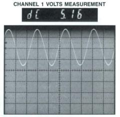
Figure 4. The average dc or true ac RMS component of a waveform is measured directly through channel 1 or from the floating DMM input.
