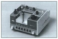
178 Linear-IC Test Fixture.
