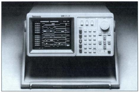
Expanded 1241 Timing Diagram With Glitches.
