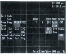
The 11301 and 11302 are fully programmable over either GPIB or RS-232. Setup of the GPIB (above) and RS-232 (below) interfaces is done directly through a touch-screen menu.
