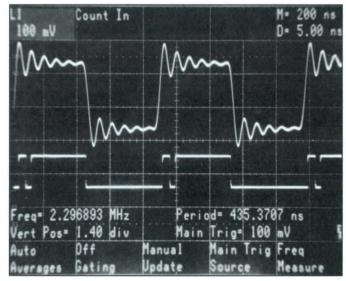
The Count In trace (lower trace) shows clearly that the counter/ timer is miscounting because of the ripple on the top of the signal.
