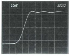
Nonstorage 1-GHz 7104/R7103. This 300-ps rise time is displayed on a 7104 Oscilloscope. Readout indicates 10-mV/div vertical sensitivity and 200-ps/div sweep speed. The 7104 and R7103 provide ultra-bright displays that permit the viewing of a single-shot transient event up to the maximum bandwidth of the oscilloscope (1 GHz) in ambient light.
