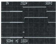
Figure 2. The propagation delay time between the input of a delay line (upper trace) and the output of the delay line (middle trace) is measured digitally. Lower trace is 7D15 pseudo gate display. CRT readout displays the result of 151.0 ns.
