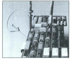
Probe Accessories shown in use on a circuit board. A circuit board connector (131-2766-03) is used to connect the probe to the test point for minimal signal distortion and maximum measurement convenience. Other connectors and adapters are available.
