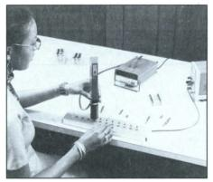
J6505 Red LED Test Probe Typical Measurement Application • Output of Red LEDs (600-710 nm)
