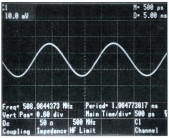
The 500-MHz combination of 11302 mainframe and 11A71 single-trace amplifier allows accurate frequency measurements of small signals to 500 MHz or more with 113000's built-in universal counter/timer.
