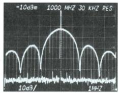
Spectrum Analysis. Max Hold feature of the 7L14 Spectrum Analyzer plug-in in a 7000-Series mainframe produces perfectly proportioned Sin x/x spectrum of low-rep-rate burst of 2.66 MHz, 6.67  $\mu$ s in width.
