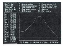
Zoom—By enlarging a designated area between two cursors, you can analyze a waveform segment in greater detail. This is a zoom of part of the waveform shown on the bottom of the previous page.
