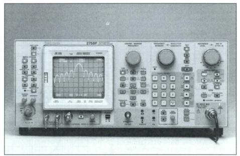
marked signals only 10 Hz apart—or count the exact delta frequency between two marked signals—even with greatly differing amplitudes. You also have the flexibility of tying in with a system clock, using the instrument's external reference lock capacity.
