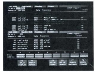
This display shows data acquired simultaneously from two microprocessors using separate 92A60/92A90 modules. The display in the lower window includes register deduction.
