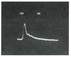
Analog-Storage, 500-MHz 7934. Transient Capture—A 7A29 plug-in and the 7934's Fast Variable-Persistence storage mode in reduced scan capture a single-shot electrostatic discharge.
