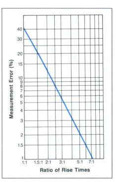
Given either specification (bandwidth or rise time), you can derive the other and determine if the instrument is suitable for your applications. The rule of thumb for timing measurements is to use an instrument with a rise time at least five times faster than the measurement you expect to make. A 5:1 ratio gives you a rise time
