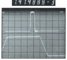
Figure 3. With the B sweep triggered, the width to be measured is within the intensified zone and polarity is selected by the B trigger slope control.
