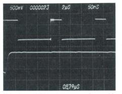
Delaying and delayed sweeps are shown with the mainframe selecting Alt sweep modes. The delay time to the start of the delayed sweep is digitally presented on the lower edge of the CRT.
