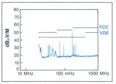
Sample graph from radiated emissions test.
