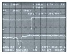
Waveform-Parameter Extraction and 2-ns glitch capture combine for DAC evaluation. The scope displays a DAC output (top waveform) with the glitch highlighted by an intensified zone. In the bottom waveform, the glitch is expanded and stored for comparison and width measurement.
