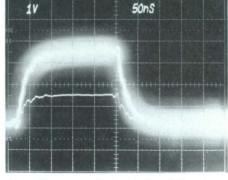
After—The same pulse train viewed directly on the 7104/R7103, with one-thousand times the brightness of conventional scopes. The researcher can now analyze the pulse with the naked eye and take pictures with ease.
