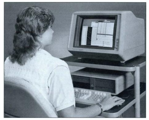
puter. The MicroVAX II is configured with 3M bytes of memory, a 31M byte hard disk, 95MB cartridge tape, and GPIB and Ethernet interfaces.
