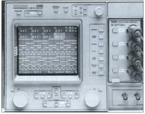
Both 11000-Series mainframes easily display eight separate traces with the deflection factor of each conveniently displayed on screen. All oscilloscope control is centered on or near the CRT, "where the action is."
