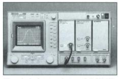
View single-shot transients at full 500-MHz bandwidth with the microchannel-plate CRT of the 11302.
