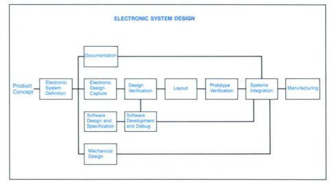
Tektronix Aided Engineering provides an integrated design, evaluation and test solution for the electronic system development process which significantly improves engineering productivity and reduces time to market.
