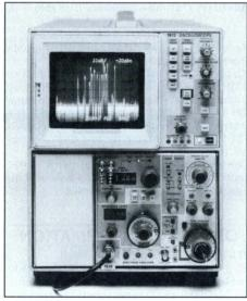
7L12 with 016-0155-00 Blank Panel in 7613 Option 06 Variable Persistence mainframe with internal spectrum analyzer graticule.
