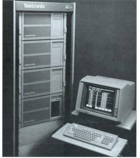
Up to three expansion mainframes can be connected to the DAS 9219 mainframe, in daisychain fashion, for a total of 28 slots. In an Automated Test Environment, the DAS 9200 can be set up and controlled over either RS-232 or GPIB interfaces.
