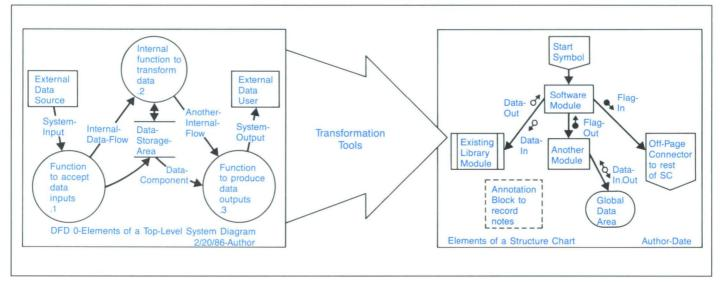
TekCASE Analyst/RT Tools create a set of interrelated data flow diagrams and descriptions that show the active functions of the system and its interfaces.
