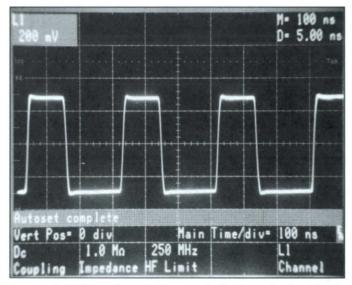
A press of a button at the probe tip or on the front panel automatically sets up the controls of the 11300 oscilloscopes for a triggered on-screen display of the selected signal.
