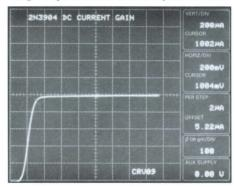
Dot Cursor Mode-Position an intensified dot cursor to any point on the waveform and read out the vertical and horizontal coordinates. The dot cursor is also useful when sending data over the GPIB:
