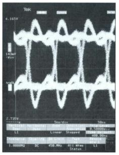
Eye patterns can be created for checking bit error rates on communications systems.
