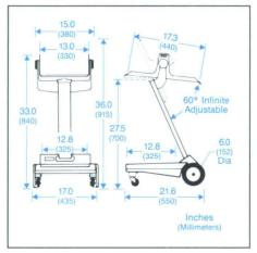
**Construction**—Base of thermoset polyester. Column and top of tray made of high-strength aluminum.
