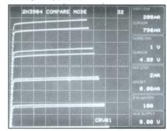
Waveform Comparisons-Simultaneously display real-time characteristic curves of a DUT, along with a previously acquired family of curves that are digitally stored in internal memory. Thus, you quickly and conveniently compare the DUT with reference data.
