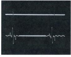
A signal with two echoes recorded at a uniform sampling rate (top trace), the same signal recorded at an increased sampling rate during each echo (bottom trace), to capture each echo with increased resolution.
