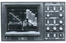
1710B Waveform Monitor-Dual Filter Display
