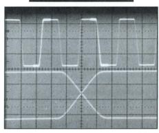
Figure 6. The time between the two intensified zones on the A sweep is measured with up to 10-picosecond resolution.
