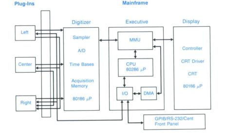
The 11400-Series digitizing-scope architecture applies extensive processing power to waveform acquisition, measurement, and display.
