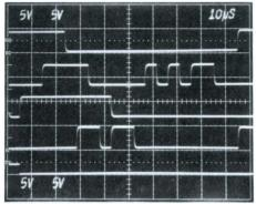
Up to four logic signals can be displayed by the 7A42 in true analog form. Additionally, the Trigger-View trace provides the ability to view exactly when the programmed Trigger Function is satisfied.
