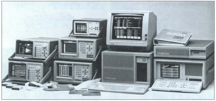
The Tektronix Logic Analyzer family includes the DAS 9200, DAS 9100, 1240/1241, 1220, 1225, and the 300 Series Logic Analyzers (not shown).
