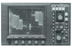
1750 Waveform/Vector Monitor—Dual Filter/ Simultaneous Display.
