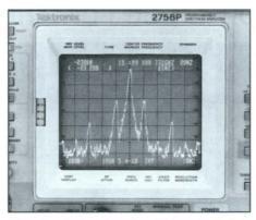
Close-in sidebands using 10 Hz Resolution Bandwidth.
