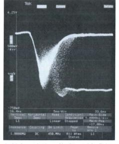
A high-resolution display with Point-Accumulate Mode along with powerful triggering makes it much easier to capture and display common digital-fault conditions like metastable states, glitches, and race conditions.
