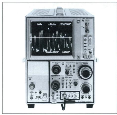
7L5 Option 25 Spectrum Analyzer with L3 (50  $\Omega$ , 600  $\Omega$ , 1 M $\Omega$ ) plug-in module in a 7603 Option 06 mainframe with internal spectrum analyzer graticule. The L3-1 module (shown at upper right) is switch selectable to 75  $\Omega$ , 600  $\Omega$  or 1 M $\Omega$ .
