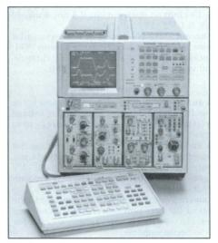
7854 Digital Storage (400-MHz Waveform Processing).
