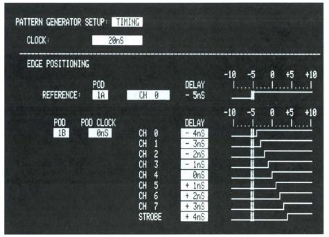
The 91S16/91S32 50-MHz pattern generator modules let you adjust the timing relationships between output clocks and data channels in 1 ns increments.
