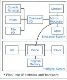
Once prototype hardware is available, designers gradually move from using emulation system resources to using prototype resources (mode 1). The final step is to use all of the prototype resources (mode 2) to execute the program. Because of the transparent nature of Tek emulators, your prototype will reliably perform in mode 2 as it will in actual operation with the emulator disconnected.
