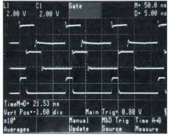
Here the 11300 universal counter/timer measures 21.53 nanoseconds of propagation delay between the leading edge of signal L1 (left plug-in, channel 1) and the leading edge of signal C1 (center plugin, channel 1). Gate trace (bottom trace) clearly shows the time interval being measured.
