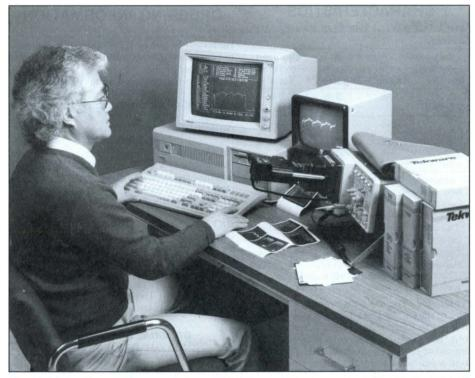
The Digitizing Camera System consists of C1001 Camera, frame store board inside the PC, DCS software, and cables. The system is shown with Tek PEP301 Controller and HC01 Hard Copy Unit.
