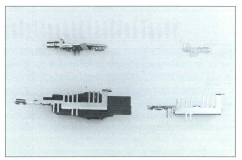
Shown above is the P6507 entire probe (top left), base (right), and P6501, entire probe (lower left), base (right).
