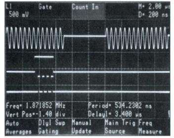
The 11300 oscilloscope delayed sweep supplies the gating signal (middle trace) for burst measurements. The Count In trace (bottom trace) shows the events being counted during the gate interval.
