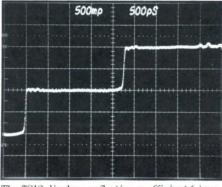
The 7S12 displays reflection coefficient ( $\rho$ ) versus distance on a device-under-test. Here the 7S12 measures a reflection caused by a crack (open) in a PCB under test. Distance can be read directly from the 7S12 front panel or calculated from the time-base settings.
