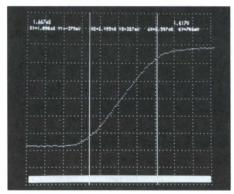
7250 CRT photo of on-screen cursors. Cursors show the vertical and horizontal setting at any two points on the display, plus the difference between these two points.
