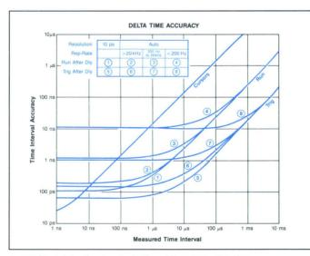
Input Signal is five vertical div with a 2-ns rise time. Measured times are four horizontal div. TJE is negligible for Slew Rates >0.1 div/ns. ΔTime Trigger After Delay assumes visual superposition.
