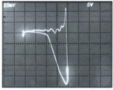
The transient load line of a fast switching transistor in a power-supply prototype (switching time=10 ns) is easily measured for compliance with safe operating area (Horizontal=Voltage; Vertical=Current).
