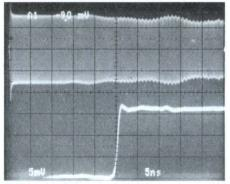
Bandwidth: Tek probe faithfully transmits 300 MHz signal.
