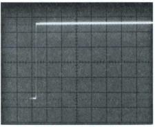
Probe Tip Accessories: Ringing does not exist with the appropriate ground lead from Tek.
