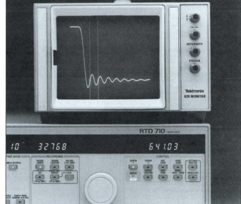
RTD 710 Cursor Display on Tektronix 620 X-Y-Z Monitor.
