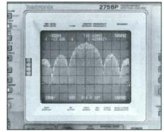
Marker measurement on Pulsed RF using Pulsed Signal processing mode.
