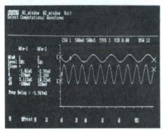
Delay-Time Measurement using an IBM PC/XT/AT as controller with Tek's Time and Amplitude Measurement Software, plus 7D20 Programmable Digitizer and Tek 7603 oscilloscope.
