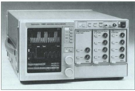
The 11401 Digitizing Oscilloscope with 500-MHz System bandwidth.
