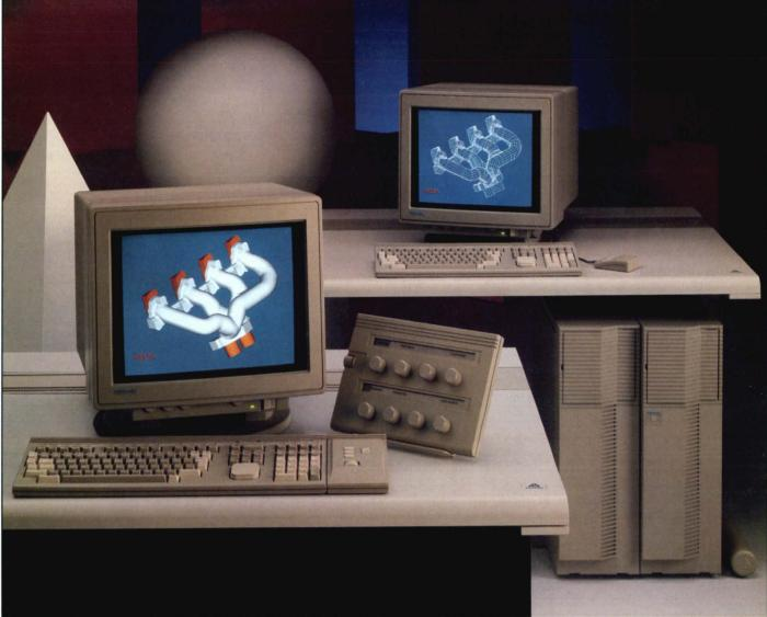
Tektronix 4330 Graphics Workstations provide 3D shaded surface and wireframe modeling systems.
