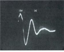
In laser research—The 7934 captures a laser primary and reflected pulse using Fast Variable-Persistence storage (reduced scan) and two 7A29 plug-ins in ADD mode.
