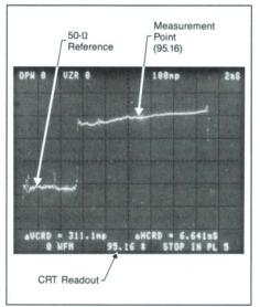
CRT photo shows an automated impedance measurement on a four-foot length of 93- $\Omega$ coax. An easy-to use program allows the operator to obtain a direct readout in ohms (bottom center) after positioning cursors on selected points on the display.
