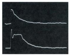
A decaying signal recorded at a 10-us sampling rate (top trace); the same signal can be recorded at a 100-ns sampling rate during the initial portion and switched back to a 10-µs sampling rate (bottom trace) to capture all information on a single-shot signal.
