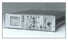
The R7903 requires only 5.25 inches of rack height in a standard 19-inch rack. It is fancooled and comes complete with slideout chassis tracks.
