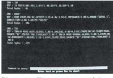
Direct entry of instrument commands is supported with control over GPIB or RS-232 interfaces and screen listing of command responses.
