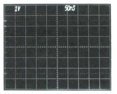
Before—Low-repetition-rate pulse is invisible on a conventional oscilloscope.
