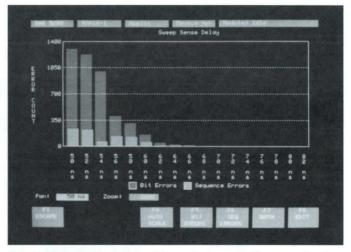
Graphs like this give a clear picture of test results. For example, when timing parameter sweeps are specified, a graph of the number of bit and sequence errors versus the value of the varying parameter can be displayed.
