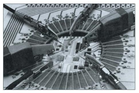
Two types of replaceable tips are offered for extended wear and flexibility: Tungsten for thick film, and Palladium for thin film and IC probing. See Replaceable Tips on the next page.
