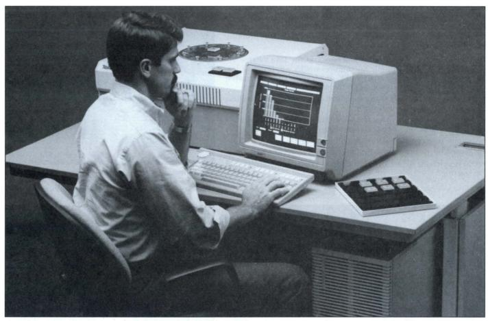
The DAS 9200 personal verification system supports application-specific IC (ASIC) functional verification, analysis, and debugging.
