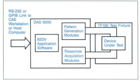
DAS 9200 ASIC verification system configuration.
