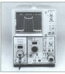
The 7L14 converts the 7603 Oscilloscope to a 1.8-GHz Spectrum Analyzer:
