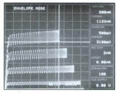
Envelope Mode and Crosshair Cursor-Capture and display maximum and minimum excursions of digitized curves. Detect subtle changes over time that you might otherwise overlook as, for example, DUT thermal drift. The crosshair cursor in this application shows predrift conditions.
