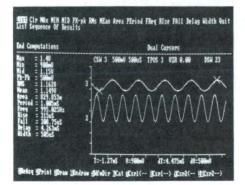
Automatic Pulse-Parameter Analysis using the 7D20/IBM PC Time and Amplitude Measurement Software.
