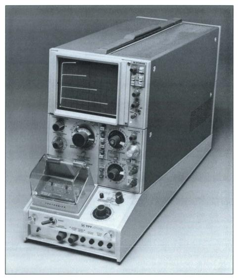
Although the 577/177 Collector Supply has lower power capability (the 576 can deliver approximately 2.2 times as much power to the device under test), approximately the same test current is available; 10 A continuous peaks at line frequency. The 577/177 provides its highest currents at a lower voltage than does the 576.
