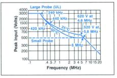
Figure 2. Maximum working voltage between probe common and earth ground.
