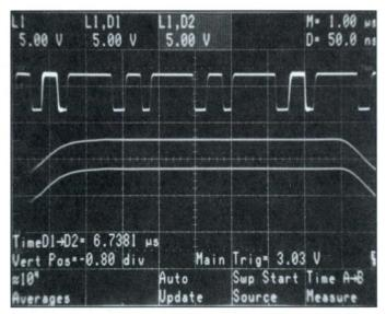
Very accurate pulse-to-pulse timing measurements within a complex pulse train are made simple with the 11300 universal counter-timer and dual delayed sweeps.
