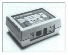
the power to the instrument is interrupted, a protective ground is reestablished, and an audible alarm is sounded. The A6901 also verifies the existence of a functional ground in the power source.
