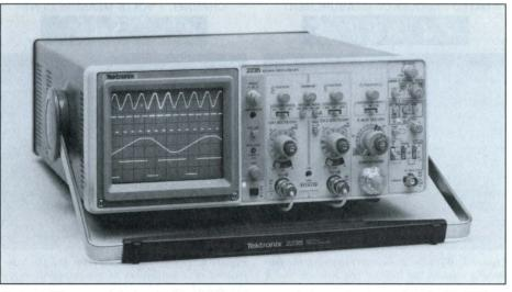
Features like rugged design, lightweight, and an easy-to-learn front panel make the 2235 an ideal service scope. In both service and design, it offers the sensitivity for low-level measurements and sweep rates for fast logic families, plus 10:1 variable holdoff range for complex word triggering. And at the bottom line, it offers the price and reliability to significantly lower the cost of owning a quality scope.
