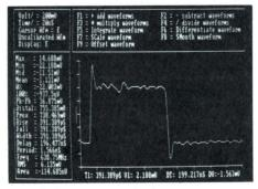
Math operations—Manipulate waveforms mathematically by using such procedures as integration and differentiation, scalar, smoothing, and offsetting (shown on top of the screen).
