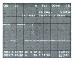
With delay by Events, the 2430A can trigger on a single clock pulse within a series to help capture an intermittent failure due to a race condition. The operator here used Absolute Windowing to select the waveform portion from trigger point "T" to the trailing edge of the glitch, indicated by the X marker.
