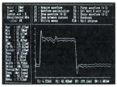
Save-on-delta—Easy-to-use software sequences let you create three types of delta masks. This shows a mask created from two waveforms.
