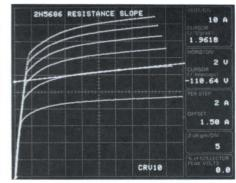
*F*-line cursor used to calculate and display resistance slope (1.96  $\Omega$ ).
