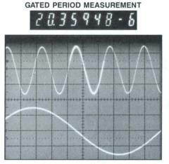
Figure 2. With the B sweep triggered, the period within the intensified zone on the A sweep is measured.
