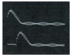
The transient response of a system at powerup recorded with no pretrigger (top trace); by using the pretrigger, the complete response can be digitized (bottom trace).
