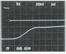
Dual-Beam 7844/R7844. The 400-MHz 7844 Dual-Beam Oscilloscope displays one input signal at two sweep speeds. The 7844 provides full vertical and horizontal crossover switching and full overlap of both vertical amplifiers on its  $8 \times 10$  cm display.
