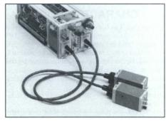
Extenders allow the user to locate the sampling head directly in a test fixture, avoiding potential signal degradation by cables.
