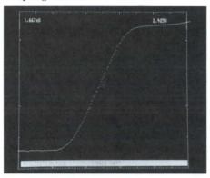
7250 CRT display of pulse rise-time measurement.
