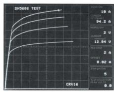
Bipolar-transistor family of curves created using the 371's sweep mode.
