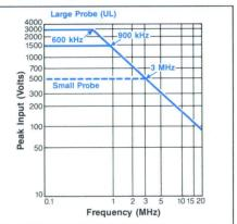
Figure 1. Maximum working voltage between probe input and probe common (all temperatures).
