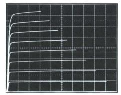
2N3904 transistor characteristic generated by the 7CT1N. Control Settings are indicated on front panel of 7CT1N.
