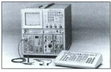
**7854 Waveform Processing Oscilloscope** This two-channel, digital storage oscilloscope has 400-MHz equivalent-time bandwidth. Keystroke programming of local keyboard and remote waveform calculator
