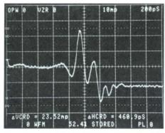
Sampling/Time-Domain Reflectometry. 7854 Waveform-Processing Oscilloscope with 7512 TDR/Sampling plug-in provides time-domain reflectometry and digital processing of sampling. In this photo, the 7854/7S12 measures a discontinuity in millirho/division and calculates an impedance of 52.41  $\Omega$  at the discontinuity.
