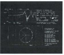
One of many accessory software packages, the RLS System Identification software produces pole/zero system models from measured stimulus/response data.
