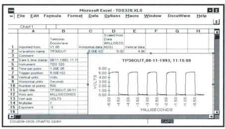
Figure 2 - Exported DocuWave waveform in spreadsheet
