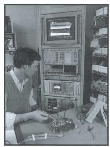
The measurement system shown here measures a microwave carrier signal. The signal is applied to a Tektronix 2784 Opt. 04 Spectrum Analyzer. The IF output of the analyzer is down converted by the RF160, effectively extending the analysis range of the 3052A.
