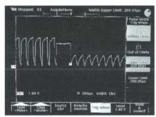
Pulse width triggering can single out faults caused by pulses which are either too narrow or too wide (all TDS 500A and TDS 600A models).
