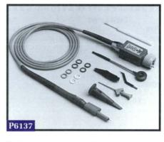
Both probes feature: modular construction, HYBRID/SMT circuitry, a smaller probe head/cable assembly than traditional passive probes, 10X attenuation readout encoding, and a full complement of attachment accessories. Smaller probe tips and light weight cable assemblies allow easy negotiation of dense circuitry or tight spaces.
