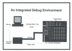
LA CONNECT combines a logic analyzer, a debug monitor, and a source level debugger to provide a real time debug environment for today's fastest and most complex microprocessors.
