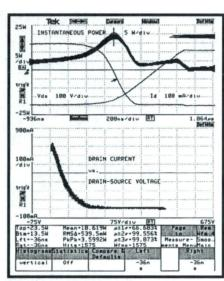
A power measurement display on DSA602A. Current, voltage and instantaneous power in a power FET are shown in the upper display. The operating area of the turn-off transition is shown in the lower screen.
