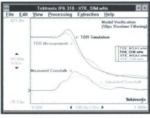
Figure 7. The IPA 310 can create coupled models to predict crosstalk. These models can be verified by comparing the simulated and measured waveforms.
