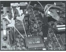
The array of probing accessories provides flexible connections to DUT. The Podlet-Style low-mass probe head simplifies hands free probing.
