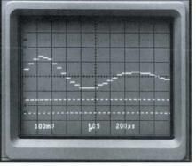
The TVC 501 instantaneously and continuously converts consecutive timing measurements to a time-interval vs. time waveform. The top trace (TVC output) shows the pulse-to-pulse width vs. time variations of the lower stream of pulses.
