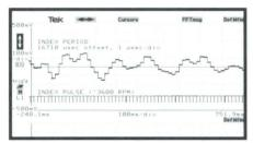
The lower signal shows the once per revolution disk drive index pulse. The TVC measures the pulse-to-pulse period variations and generates the upper waveform. The timing offset was set to 16710 usec to show the  $\pm 2$  µsec period variations.
