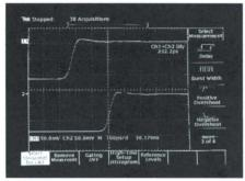
The TDS 820 provides 0.4 ps timing resolution and channel deskew capability to accurately measure delays in today's high-speed digital systems.
