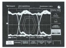
On-board mask drawing capability allows visual comparison of signals to standard masks in communication systems (TDS 820).
