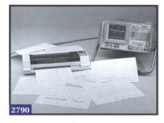
Tektronix 2790 Series Spectrum Analyzers provide convenience features usually not available at the affordable prices of these products. Shown above, a GPIB plotter provides a permanent results record while the spectrum analyzer continues to acquire new signals. Buffer memory storage permits simultaneous operation of the plotter and spectrum analyzer.
