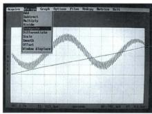
Manipulate waveforms mathematically by using such procedures as integration, differentiation, addition, and subtraction with DCS01GPH
