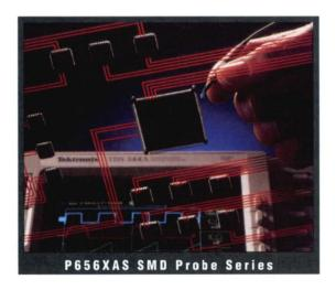
SureFoot<sup>™</sup> is an integral probe tip and miniature guide that enables fault-free hand-probing of fine-pitch SMD packages. Using the IC's leads as guides, SureFoot's non-conductive tines align with the leads before the probe tip can contact the device, thus preventing the probe tip from shorting adjacent pins.
