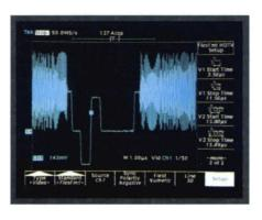
Fortunately, the TDS 644A has a solution: the FlexFormat™ mode. Unique to the TDS family Video Trigger Option, FlexFormat allows you to specify the timing of customized of tri-level sync pulses, input any field rate between 20 and 200 Hz, and define the number of lines and fields in the format. The screen photo above shows an HDTV waveform and some of the FlexFormat menu selections used to acquire it, as viewed on a TDS 644A.
