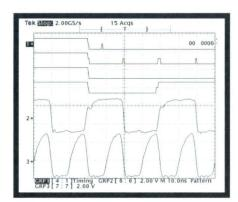
Ground spikes are revealed by the TLS 216 (upper two traces).
