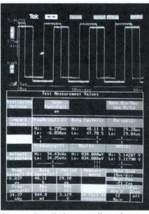
Figure 3. Pass/Fail testing offers a fast, easy method of adjusting circuit operation or sorting parts in production applications.
