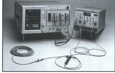
High Resolution Optical Reflection Measurement using OIG 502, OCP 5502 and the CSA 803A.
