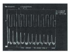
FFT analysis provides an extra dimension of performance with simultaneous displays in the time and frequency domains (optional on TDS 400, monochrome TDS 500A/600A and the TDS 820, standard on color TDS 500A/600A).
