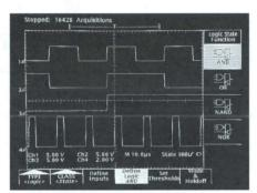
Logic timing analysis is clearly faster and easier with icon-driven state triggering (all TDS 500A and TDS 600A models).
