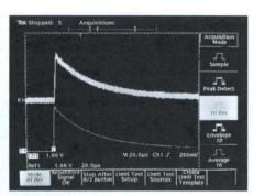
Hi-Res acquisition mode achieves extremely high signal to noise ratios (SNR) on single shot events by oversampling the input signal (all TDS 400 and TDS 500A models).
