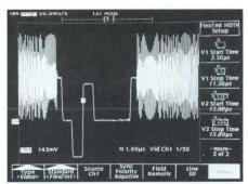
An optional video trigger features line and field selection on standard and user definable HDTV formats (TDS 500A and TDS 600A).
