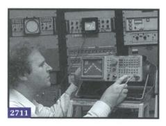
**Display Dynamic Range** – 80 dB max (limited to 40 dB in optional 2712 Quasi-peak Detector mode).
