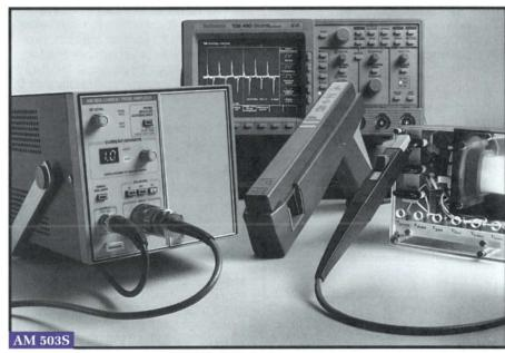
AM 503S current probe system with both A6303 and A6302 current probes. The A6302 is measuring the fluorescent ballast line current which is displayed on a TDS 460 Digitizing Oscilloscope. For information about ballast testing request application note 51W-8614-0.
