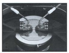
Figure 9. Characterize MCMs, hybrids, and wafers using the TMP 9000 microwave probes.
