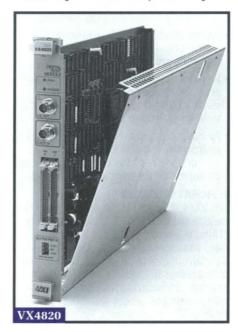
stimulus and real time response compare for up to 64 I/O pins per module and up to 12 modules (768 pins) can be accommodated in a single mainframe. Each pin of the VX4820 Digital Test Module can be programmed for drive HI, drive LO, compare HI, compare LO, drive HI and compare HI, drive LO and compare LO, inhibit ( high impedance). These are programmable for each test vector to support testing of bi-directional bus structures and multi-master systems.
