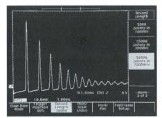
Record lengths of up to 60,000 points (TDS 400 Opt. 1M) enable very high timing resolution on even the most complex waveforms. Or capture unexpected events that happen well before or long after the trigger event.
