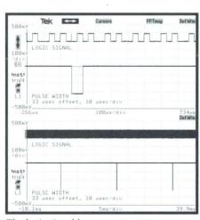
The logic signal has a constant 33 usec pulse width, but there is an occasional glitch. In the width mode, the TVC instantly responds to the glitch and recovers after the next pulse. Over a longer measurement interval (lower screen), the logic signal appears as a blur; the TVC shows that the glitch is periodic.
