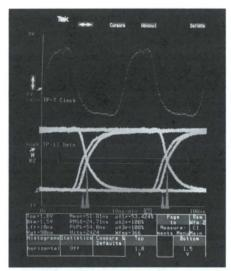
Figure 3. Analyze digital communications using variable persistence display modes. View in X-Y format for constellation display. Apply horizontal or vertical histograms to analyze jitter. Use crosscorrelation for accurate propagation time measurements in extreme-noise environments.
