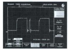
TDS triggering can capture glitches as narrow as 2 ns to help solve prototype circuit problems quickly (all TDS 500A and TDS 600A models).
