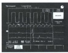
Four channels help show a time-correlated display of both digital control and analog feedback signals (TDS 420, TDS 460, TDS 540A/544A and TDS 640A/644A).
