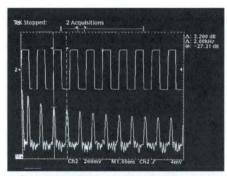
Tektronix' exclusive TriStar™ DSP engine brings simultaneous time and frequency domain analysis to mid-range scopes in the TDS 400, TDS 500A, TDS 600A and TDS 800 products.
