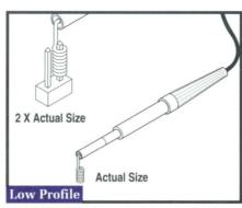
Circuit Boards in System Enclosures - 25 mil square-pin headers on 100 mil centers.
