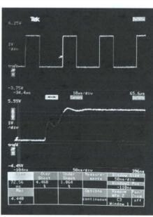
Figure 2. In the Annotation Mode, horizontal cursor bars and highlighting serve to focus your attention on the portion of the waveform being measured.
