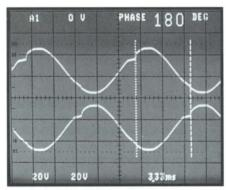
With the delta-time and voltage cursors, you can measure a waveform's parameters including phase.
