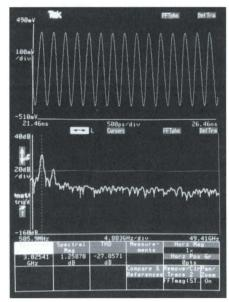
Figure 2. FFT display and measurements in the 11801B offer additional analysis power to the engineer or scientist.
