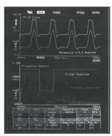
Figure 4. Apply signal processing to perform simulations. Edit the frequency spectrum of a live signal by multiplying its FFT by a filter function. Transform the result back to time-domain using IFFT and see the effects of the digital filter on the live signal. Convolution is also available for filtering.
