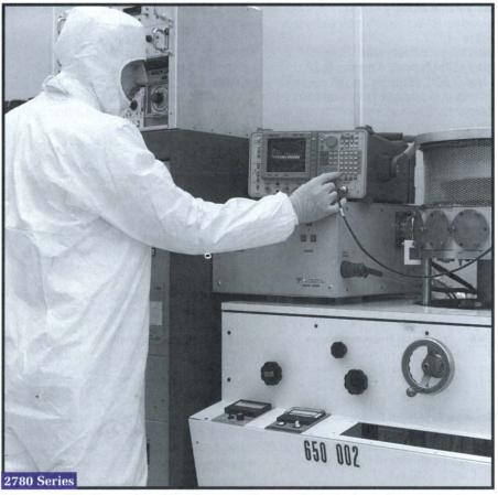
Microwave Chip Research and Development: The 2780 Series is shown here monitoring microwave component research and development in a lab clean room.
