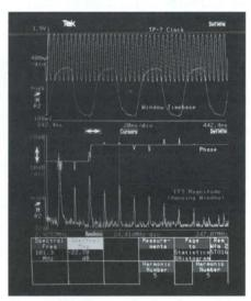
Figure 6. Simultaneously view time and frequency-domain displays of signals at live speeds. Apply harmonic or peak-search cursors for efficient, high-accuracy readout of spectral magnitudes and frequencies. Display magnitude and phase information for repetitive or transient events.
