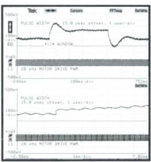
The TVC shows the pulse width variations of a motor drive signal as the controller jogs the speed (upper screen). The 20 kHz PWM signal itself is a blur. On the lower screen the two signals are windowed around the transition. The TVC unveils an instantaneous step in pulse width as well as a pulse width oscillation.
