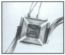
$FlexLead^{TM}$  Adapter offers connection to SMT devices of 20 and 25 mil spacing.
