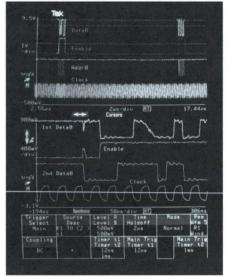
Figure 1. Isolate setup/hold time violations, metastable states and glitches quickly with time-qualified triggering. Apply the window time base to zoom in for more details. Signal paths are time-matched to probe tips for accuracy.
