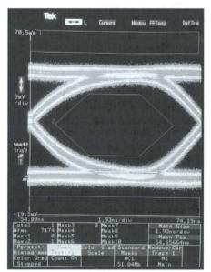
Figure 3. Predefined Telecom masks make verifying digital stream conformance simple.
