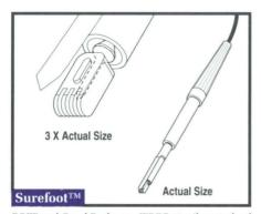
PQFP and Quad Packages - JEDEC 25 mil center lead spacing EIAJ 0.5 and 0.65 mm center lead spacing.
