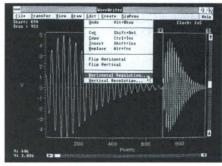
WaveWriter allows easy creation and modification of custom waveforms.
