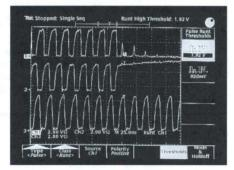
TDS exclusive runt triggering helps isolate invalid logic levels such as those caused by setup and hold violations (all TDS 500A and TDS 600A models).
