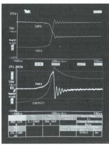
Make accurate, high-bandwidth power measurements and energy calculations with the 11A16 Programmable Current Amplifier and 11A33 Differential Comparator. Current and Voltage maintain their proper phase relationship to 50 MHz.
