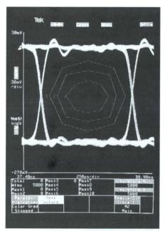
Figure 3: You can perform tolerance testing with the unique mask testing capabilities of the Communications Signal Analyzers.
