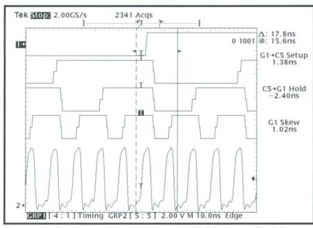
$The \ Logic \ Scope \ features \ twenty-eight \ Automatic \ Measurements \ including \ Setup, Hold \ and \ Skew \ measurements.$
