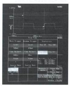
Figure 4: The CSA 404 is equipped with precision Time Interval Hardware for Counter/Timer like measurements. Time Interval measurement resolution of 200 ps single shot and 10 ps averaged provide a higher level of utility than measurements performed by waveform digitizing.
