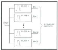
The filter bank consists of a number of parallel resolution filters that are equally spaced in frequency, and have slightly overlapping pass bands. The bandwidth of the resolution filters, is the frequency resolution of the filter bank.
