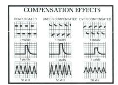
Tip - Always remember to check/adjust the compensation of your probe when you move it between channels or to another scope.
