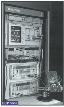
Tektronix Physical Layer Standards Compliance Test System for testing to high speed digital communications standards such as FDDI and SDH/SONET. OCP 5002 shown in TM5006 Modular Instrument Mainframe.
