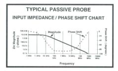
Capacitive loading of voltage probes is the most important consideration when measuring fast-rise time pulses. The time required to charge the input capacitance of the probe from the 10 to 90 % level is:
