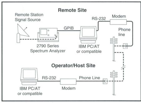
Equipment setup for remote site signal monitoring.
