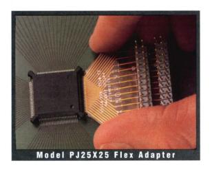
Meaningful measurements simply aren't possible without secure. high-quality connections to the test point(s). **Tektronix** probing solutions range from conventional "pencil" styles to specialized multi-pin IC probe adapters.
