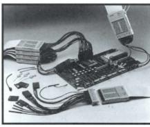
The GPX probing is comprised of four 20 channel lightweight probes. Eight channels can be grouped together in a podlet holder. Each podlet is 100 mil square and easily interfaces to a wide variety of testclips and probing accessories.
