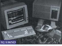
The 92A96SD offers an unprecedented memory depth of 512K bits per channel.
