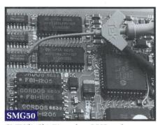
SMT KlipChip $^{\text{TM}}$  used on SOIC package.
