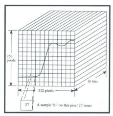
Figure 1: The unique 512 x 256 x 16-Bit data array counts and records the number of times each pixel in the display is activated.
