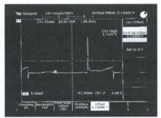
Calibrated vertical offset allows capture and analysis of small signals riding on top of large DC offsets (all TDS 400, TDS 500A and TDS 600A models).
