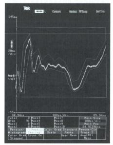
Figure 4. TDR go/no-go impedance measurement suing masks.
