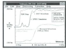
Figure 4. Verify models by comparing simulated and measured waveforms. Filter the measured and simulated waveforms to verify the model at a user specified signal risetime.
