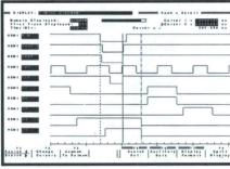
Sampling all 20 channels simultaneously at 2.5 ns, the 30HSM assures that you can make detailed timing measurements even if your design is based on the very newest logic families.
