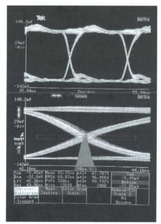
Figure 2: Histograms let you make extremely accurate jitter and noise measurements with one Data Acquisition.
