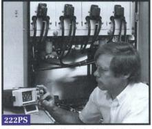
The 220 family of hand-held DSOs helps make measurements in difficult environments safely and accurately.
