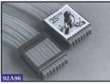
The 92A96 provides accessibility to signals with 8-channel probes as small as a US postage stamp.
