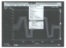
Create the reference memory template waveform for pass/fail testing on 2400 Series Oscilloscopes.
