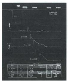
Figure 5. Rapidly capture a sequence of transient events and store them in non-volatile memory. Scan for significant events and apply measurements to individual waveforms or the entire collection. Annotate, hardcopy and transport publication-ready results on 1.44M MS-DOS compatible floppy disk.
