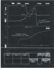
Figure 2. Capture periodic or transient current and voltage signals and accurately compute instantaneous power. Apply FFT to examine harmonics or switching noise. The TVC 501 directly demodulates pulseby-pulse PWM.
