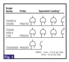
Figure 1 presents a sample conversion of the SMD probe family's capacitive circuit loading to an equivalent number of typical CMOS gates. Being aware of the potential effects of probe loading on the circuit under test can eliminate chasing false indicators, reduce test times, and lead to more accurate and repeatable measurements.
