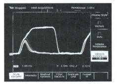
A variable persistence display mode lets you get a statistical view of waveform changes with 16 levels of intensity grading (all TDS models) and color grading with color TDS 500A/600A.
