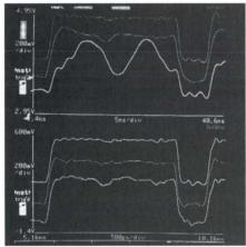
The waveforms above show the effects of ground lead inductance. The top three traces show how the displayed waveform changes as the passive probe's ground lead length is increased from 1/2 in. (top trace) to 6 in. to 12 in. (bottom trace). The bottom three traces show how an Active probe's waveform remains relatively unchanged regardless of ground lead length using the same ground lead sequence as the passive probe in the top three traces.
