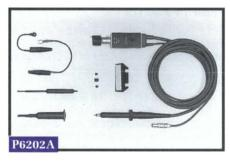
AC or DC coupling selection is available on the P6201 and P6202A FET Probes. When AC coupled, the DC voltage component is blocked allowing viewing of super-imposed signals.
