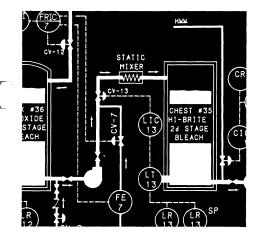
Fig. 2. Plots from the CalComp 1051 serve as artwork masters for the graphic panels.
