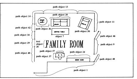
The Graphic Model Exchange (GMX) file generated to create this drawing is listed at the end of this article. Annotations relate code to the room's components.
