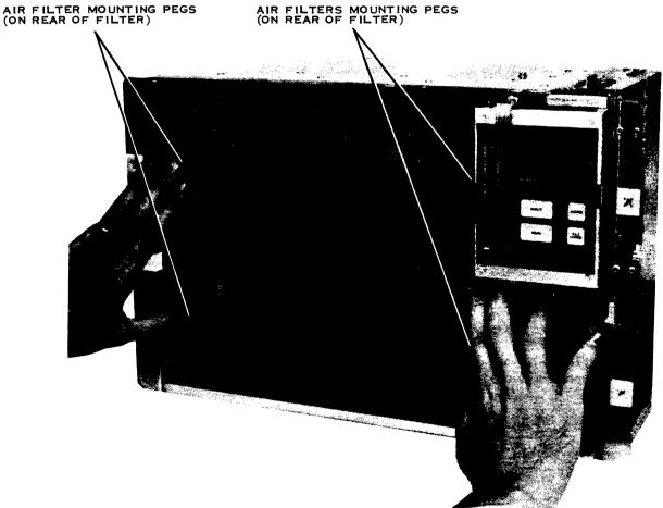
Figure 3-2. Replacing the Air Filter
