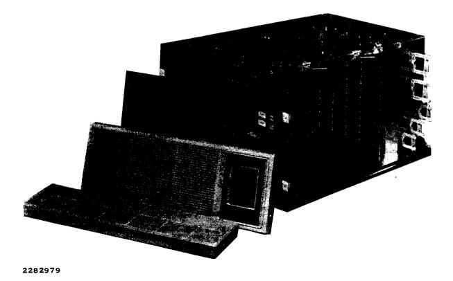
Figure 1-2. Model 990A13 Chassis with Trim Panels Removed
