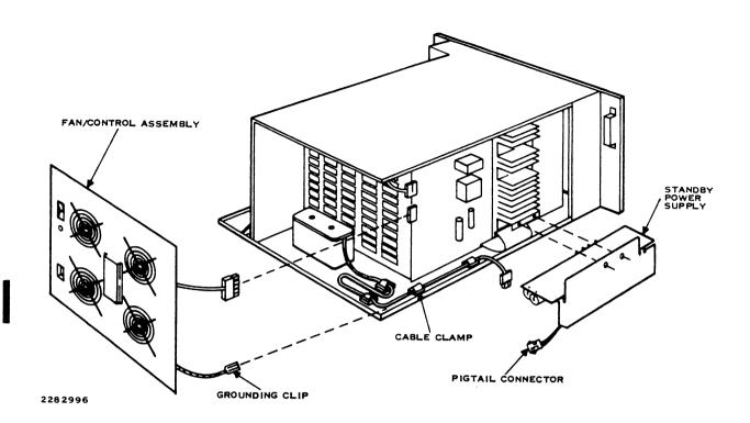
Figure A-2. Battery Cable Clamp Locations
