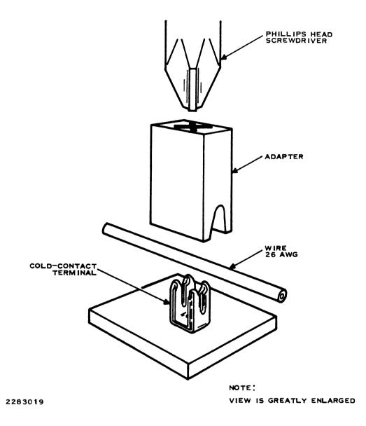
Figure 4-11. Inserting a Wire with the Adapter Tool
