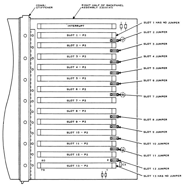
Figure 2-14. TILINE Access-Granted Jumper Locations for 990A13 Chassis
