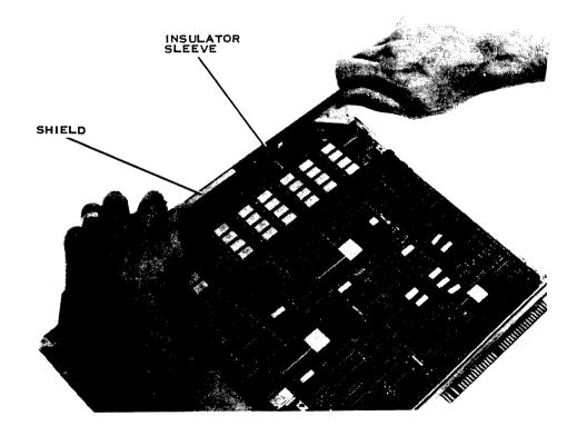
Figure 2-16. Installing/Removing an Insulator Sleeve
