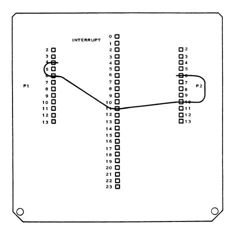
Figure 4-6. Daisy-Chain Connection to One Interrupt Level
