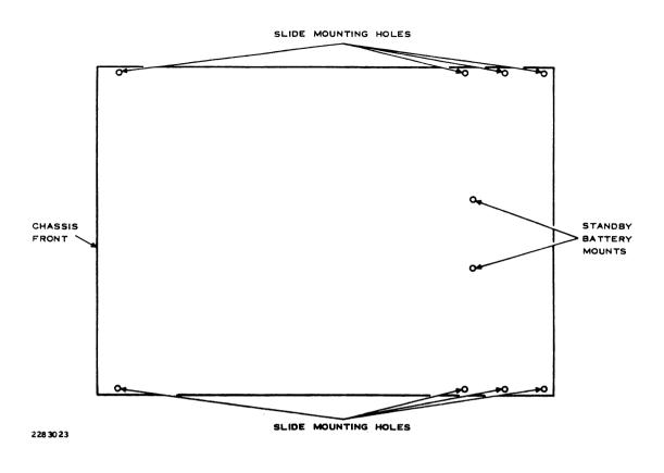
Figure 2-8. Bottom View of Chassis for Mounting
