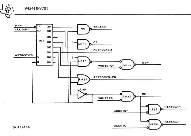
Figure 1-6. Ring Counter Logic
