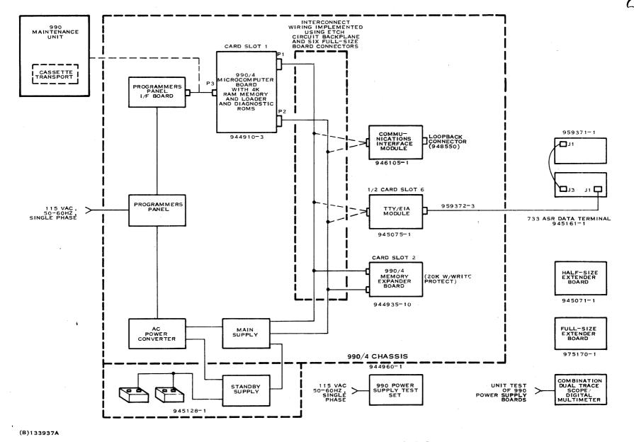
Figure 2-1. Model 990/4 Computer Hot Mock-Up System
