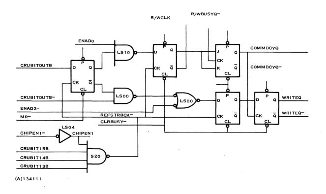
Figure 1-12. Read/Write Control Logic
