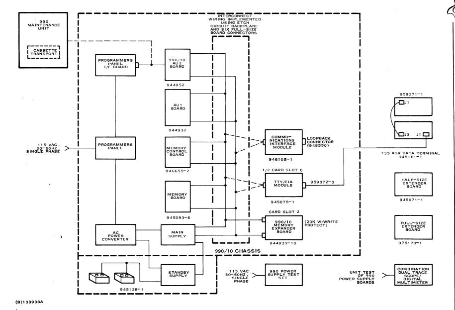
Figure 2-2. Model 990/10 Computer Hot Mock-Up System
