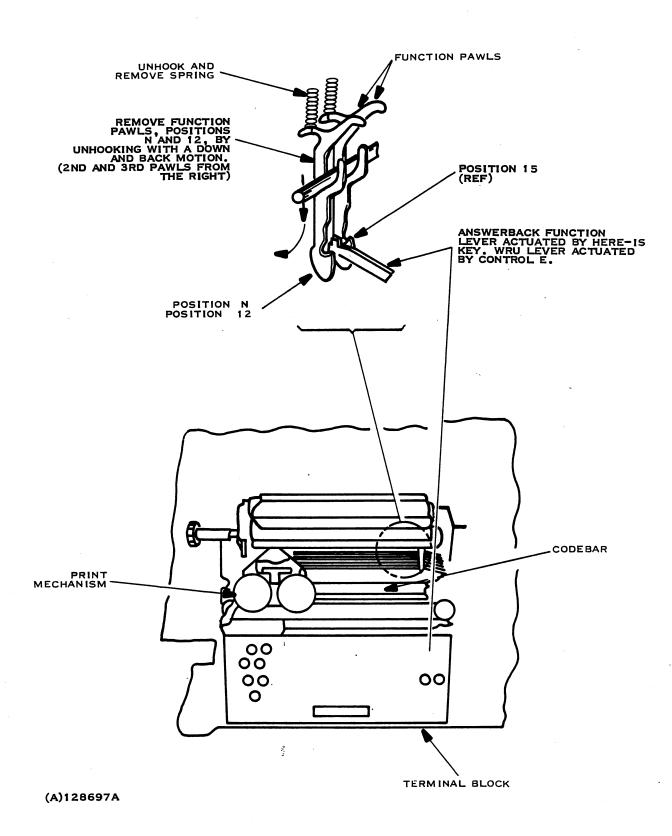
Figure 2-11. Answerback and WRU Function Bar Removal
