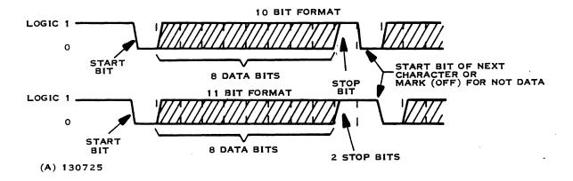
Figure 1-3. Asynchronous (START/STOP) Data Transmission Formats
