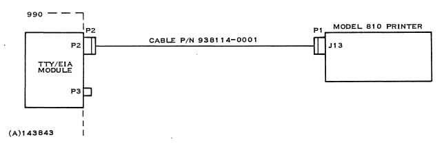
Figure 2-7. 990 Computer/810 Printer Interface, Cable Interconnection
