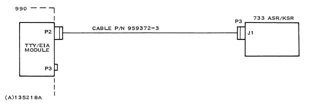
Figure 2-5. 990 Computer/733 ASR/KSR Interface, Cable Interconnection
