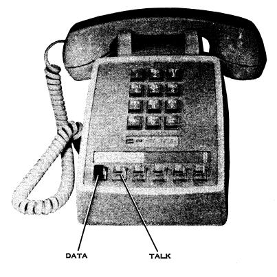
SIX-BUTTON RTC TELEPHONE WITH DATA AND TALK MODES CONTROLLED BY THE FIRST TWO BUTTONS ON THE LEFT
