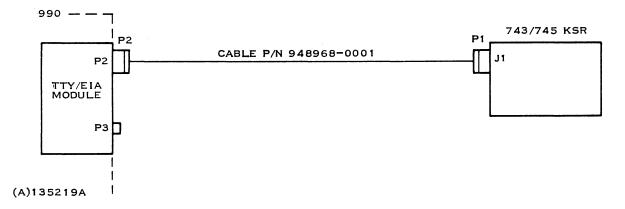
Figure 2-6. 990 Computer/743-745 KSR Interface Cable Interconnection
