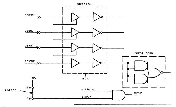
\*With kits 2265150-0001/0002, RCRE is replaced by Ring Indicator. (A) QUAD EIA RECEIVER
