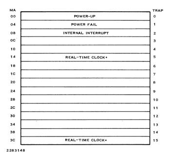
Figure 3-2. Interrupt Traps
