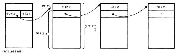
Figure 5-5. Buffer Linkage
