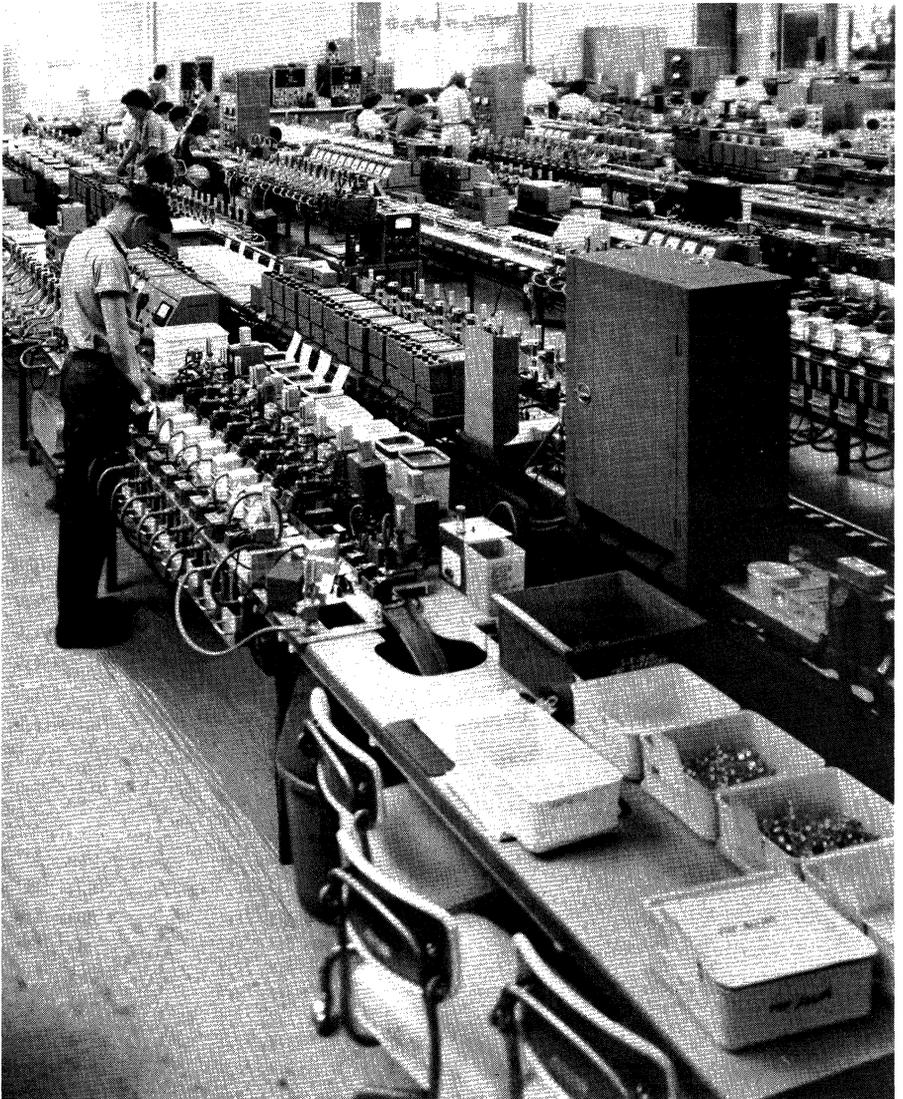
**Centralized Automatic Testers (CATs) automatically test quantities and parameters, and categorize thousands of transistors every hour without danger of human error.**
