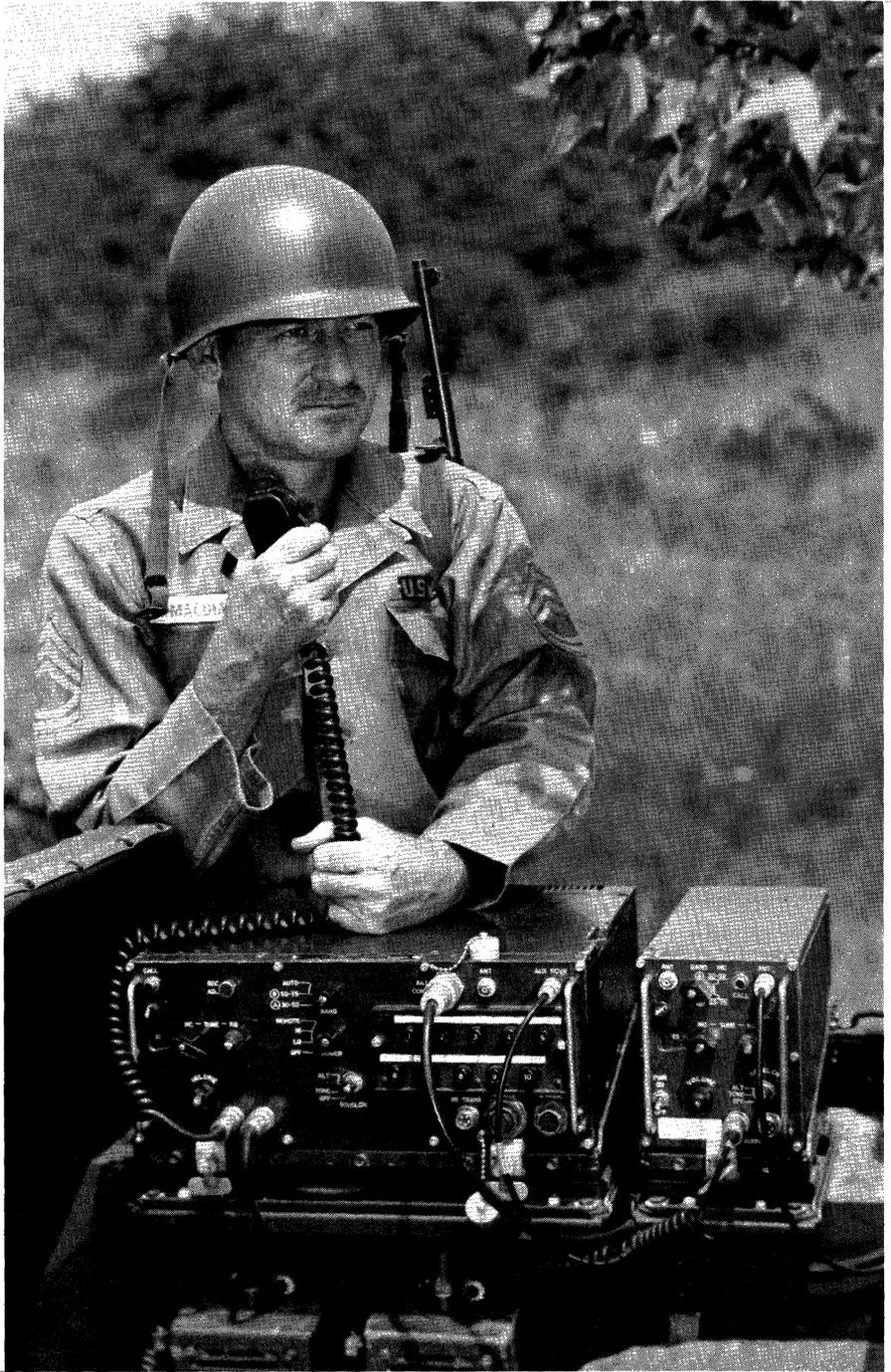
**AN/VRC-12 field radio, using TI transistors and diodes, was developed and is being produced by AVCO Electronics Division, Cincinnati, Ohio. (U.S. Army photograph)**
