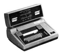
Silent 700 Model 733 ASR with USASCII code and Model 732 ASR with BAU-DOT/CCITT code... available with single or twin magnetic tape cassettes.
