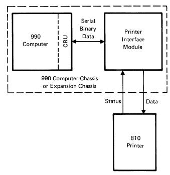
FIGURE 12 - Model 990 Block Diagram
