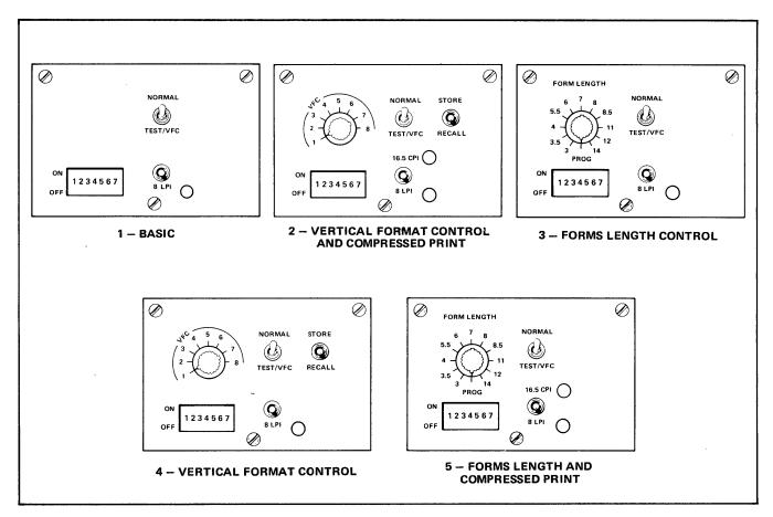
FIGURE 4 — Auxiliary Control Panel Configurations
