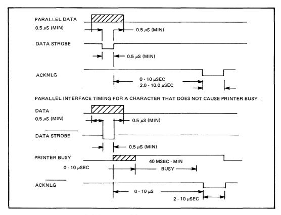
FIGURE 6 - LBP Parallel Interface Timing
