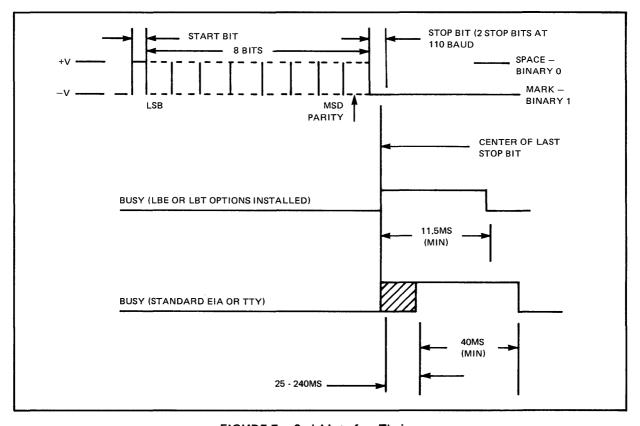
FIGURE 7 — Serial Interface Timing
