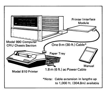
FIGURE 11 — Installation with Model 990 Computer System
