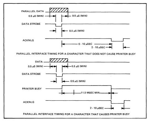
FIGURE 5 - Basic Parallel Interface Timing
