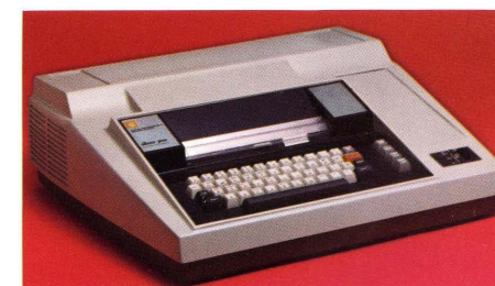
KSR Model 732 KSR with BAUDOT/CCITT code and Model 733 KSR with USASCII code...KSR models that can be easily upgraded to ASR models.
