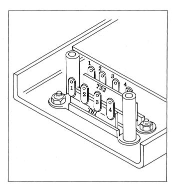
Figure 5-4. Power Supply Terminals
