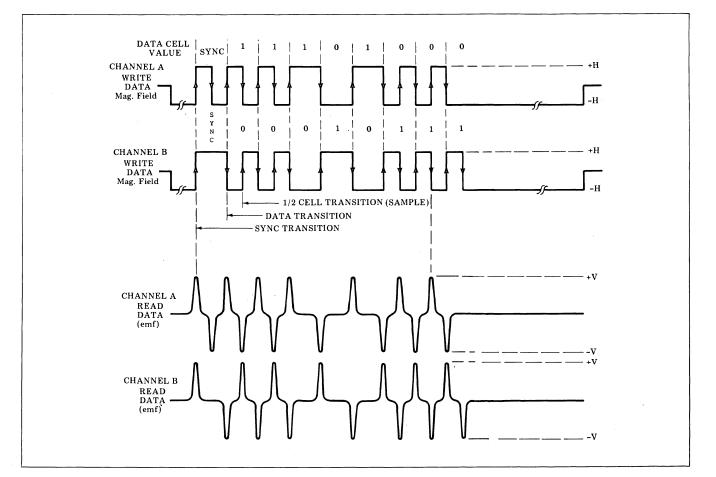
Figure 4-1. Write/Read Waveforms of 16-Bit Data Word 1010100110010101
