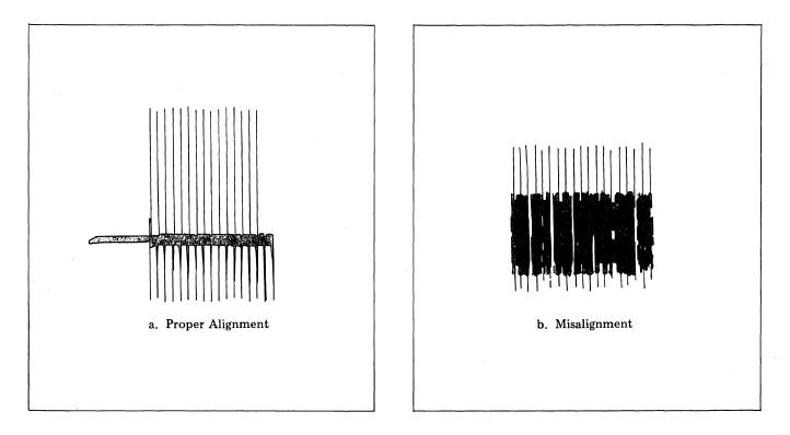
Figure 5-5. Head Alignment Checkout Waveforms
