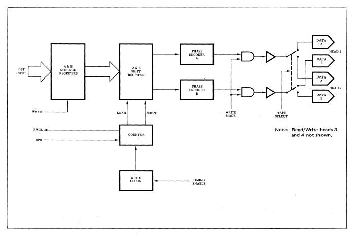
Figure 4-4. Write Operation Block Diagram
