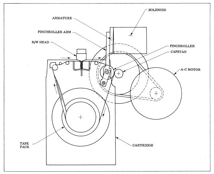
Figure 4-2. Tape Transport Mechanism
