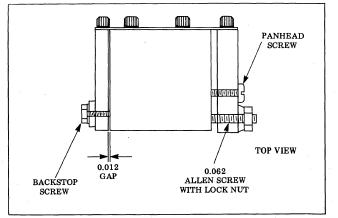
Figure 5-1. Actuator Adjustment Points
