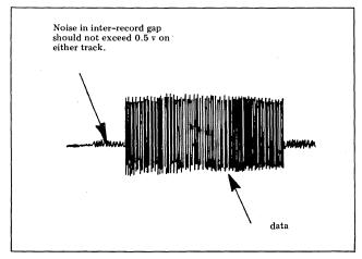
Figure 5-7. Vertical Alignment
