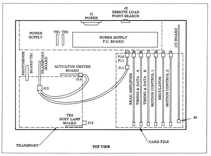
Figure 5-3. Location of Electronics Assemblies, Connectors, and Terminals
