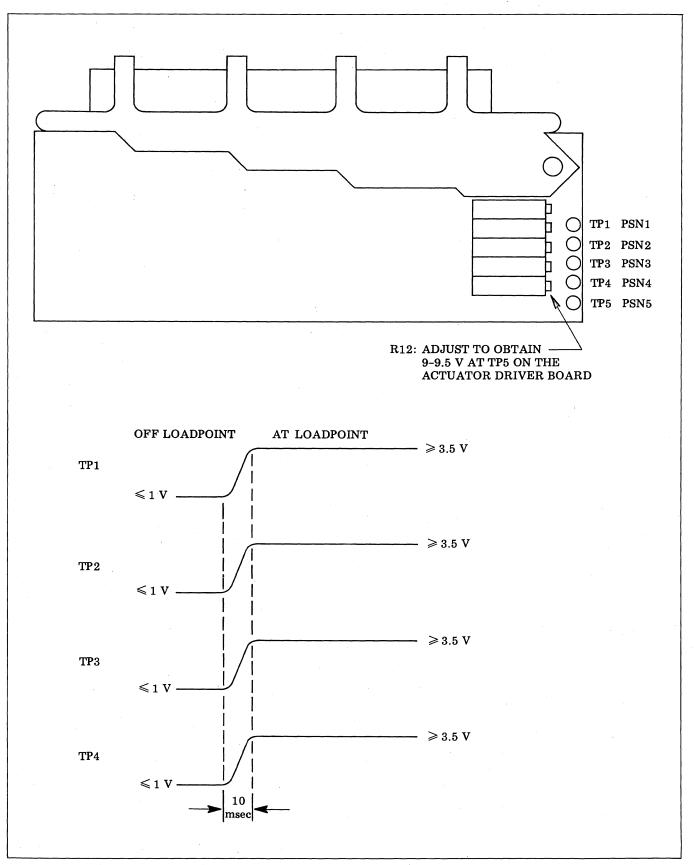
Figure 5-14. Photosense & Lamp Board 10972-0
