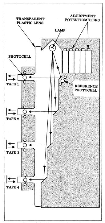
Figure 4-3. Photosense Assembly
