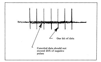
Figure 5-6. Azimuth Alignment
