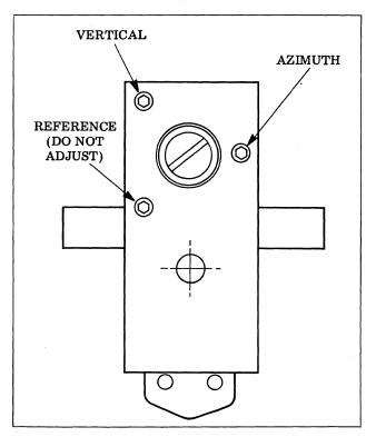
Figure 5-8. Head Adjustment Screws
