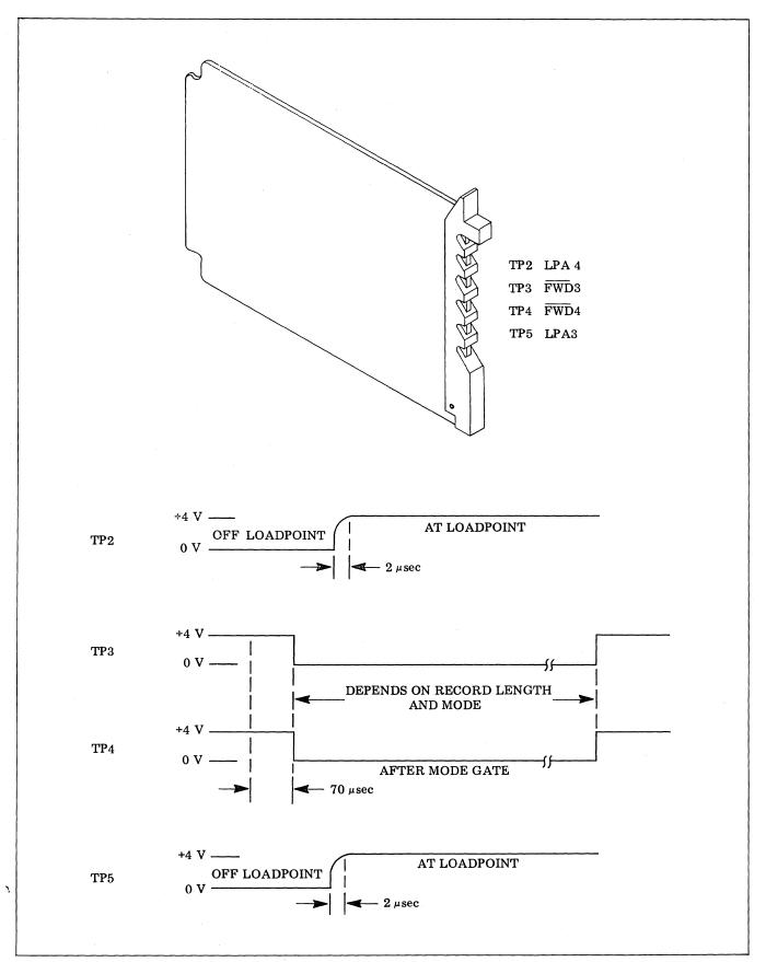
Figure 5-13. Motion Control 2 Board 10968-0
