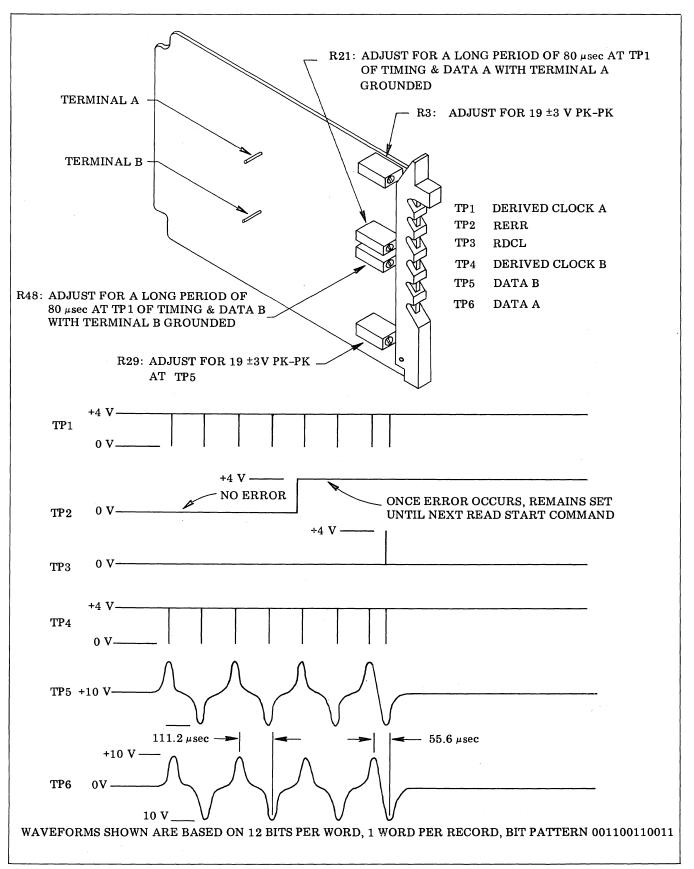
Figure 5-9. Read Amplifier Board 10746-1
