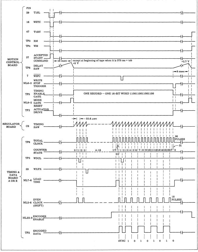
Figure 4-5. Write Timing Diagram
