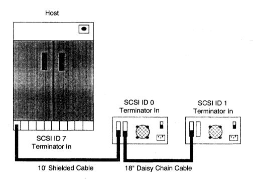
Figure 3-2 Multiple Host/Single Drive Configuration
