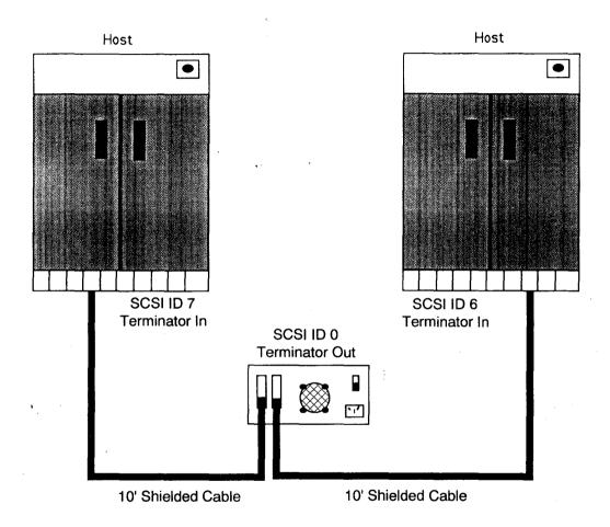
Figure 3-3 Multiple Drive/Multiple Host Configuration
