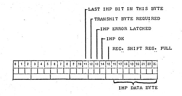
IF THE RECEIVER ON (RON) CONTROL BIT IS SET, THEN ATTENTION 2 WILL BE SENT TO THE CHIO WHENEVER THE RECEIVE SHIFT REGISTER IS FULL. IF ATTENTIONS ARE DISABLED THEN THE INTERFACE MAY BE HANDLED BY TESTING ON THE REC. SHIFT REG. FULL STATUS BIT. RON AND REC. SHIFT REG. FULL MAY COME ON IN EITHER ORDER TO SET ATTN 2.
