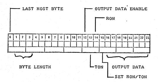
DATA AND CONTROL FIELD LOADING IS SEPARATELY ENABLEABLE BY BITS 12 AND 15 RESPECTIVELY. THEY MAY BE BOTH ON (AS WHEN OUTPUTTING THE FIRST OR LAST BYTE SAY) OR NEITHER ON (AS WHEN A POT IS DONE SOLELY TO MAINTAIN THE HOST OK TIMER TO THE IMP, TO BE DISCUSSED LATER).
