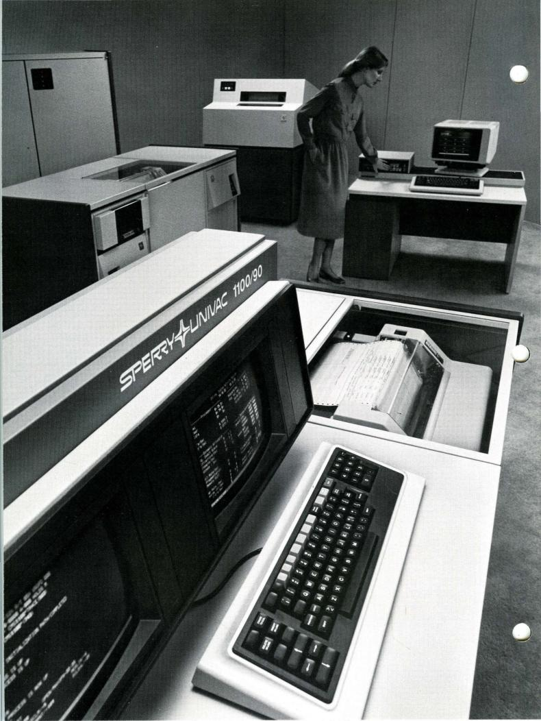
Front-end/Network Processors include the Distributed Communications Processor (DCP) family, which is a highly sophisticated computing system designed especially for communications network processing. These systems may be installed on-site connected to the 1100/90 system by input/output channels or connected remotely by high-speed communications lines.
