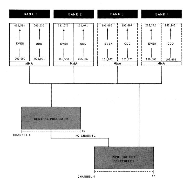
Figure 2---6. Single Processor with 1/O Controller and Interleaved Storage
