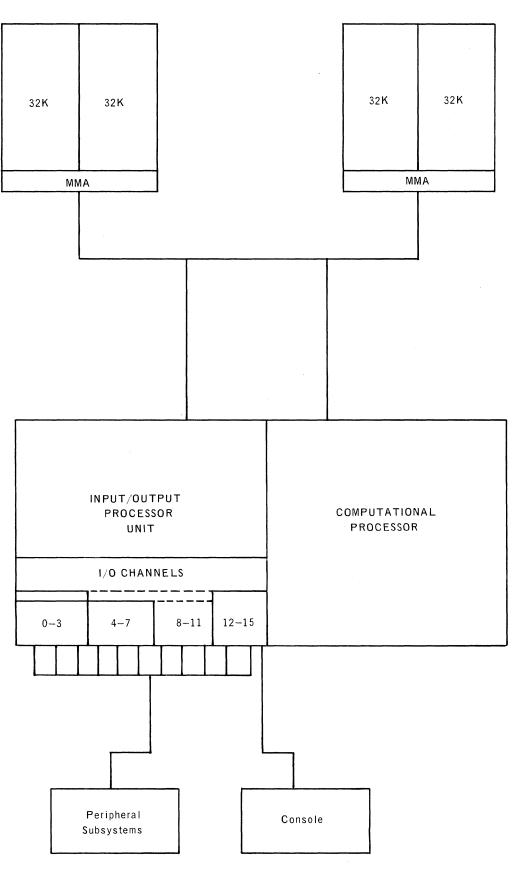
Figure 5-1. UNIVAC 1108 Shared Processing System
