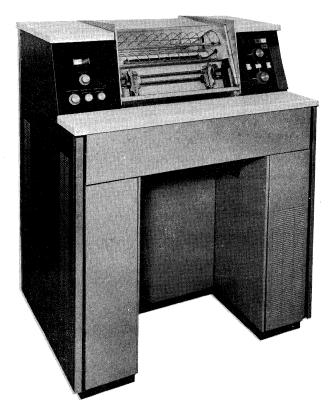
The UNIVAC High Speed Printer Subsystem provides the UNIVAC 1108 System with an output printing unit that is capable of printing single or multiple copies of data. Each line of output data may contain up to 132 printed characters. Printing operations occur on a request acknowledge basis allowing the processor to perform other processing functions while the printer is printing data.
