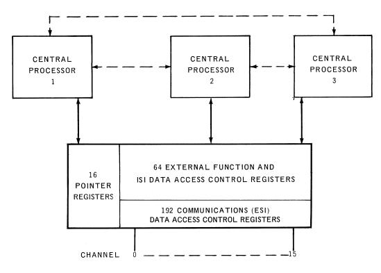
Figure 2-1. The Input/Output Controller
