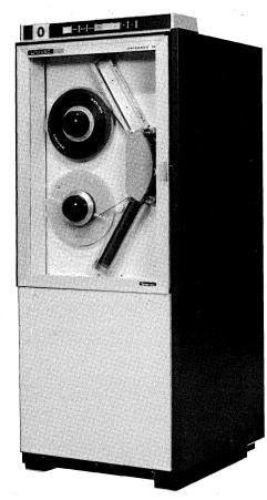
The UNISERVO 12 Magnetic Tape Subsystem is a low-cost medium performance subsystem with 7- or 9-track, 1600 frames per inch, and phase encoding as the available tape formats. One master tape unit, with a power supply and control circuits, controls up to three slave units. Up to 12 tape units are synchronously controlled by a UNISERVO 12/16 control unit.
