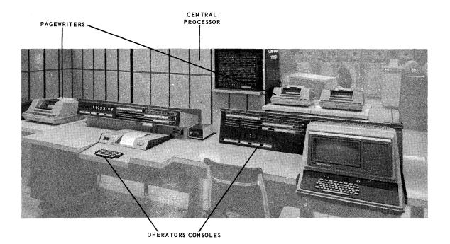
Figure 1–1. The Central Processor and Operator's Console
