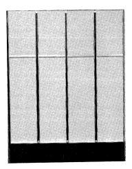
The FH-880 Magnetic Drum Subsystem has three times the capacity of the FH-432 drum; however, its access time is four times greater than the FH-432 drum.
