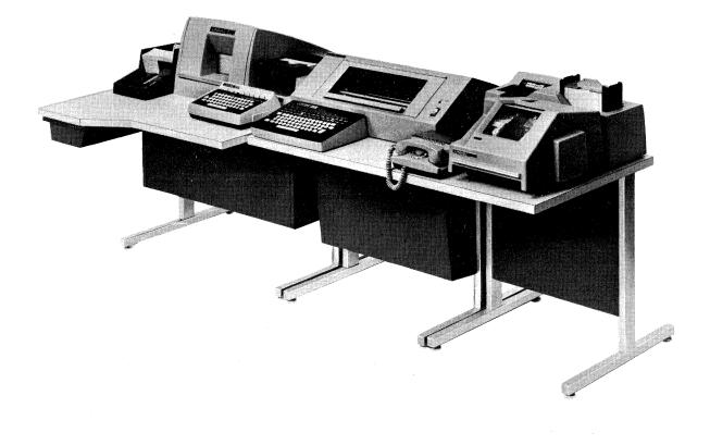
The Data Communication Terminal (DCT) 1000 is a fully buffered 30 character per second incremental printer which can be expanded to include a keyboard, card reader, card punch, paper tape reader/punch, and an auxiliary printer. The DCT 1000 transmits data or receives data from a local or remote computer or to a remote DCT 1000 in a conversational or batch mode.
