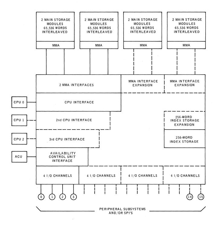
Solid lines indicate basic unit. Dotted lines indicate optional expansion units.
