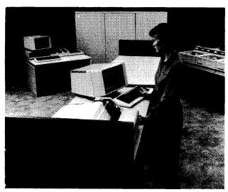
Sperry's 1100/70 Series of mainframe computers is available in an entry-level model that has a single central processor with 2MB of main memory expandable to 16MB (1100/71 B1) and a multiprocessor version that has four central processors, 64K bytes of buffer storage, and 4MB of main memory expandable to 32MB (1100/74 H2).
