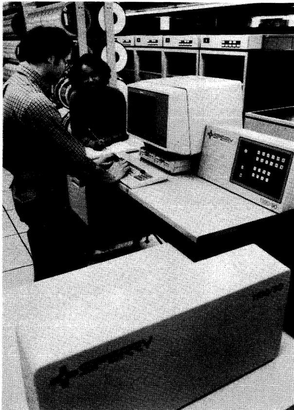
Sperry's latest addition to the 1100/90 Series is the single processor 1100/91 SV rated at 5.5 MIPS and the dual processor 1100/92 SV rated at 10.2 MIPS. These two models offer Sperry 1100/60 and 1100/70 users a lower entry point into the 1100/90 Series.
