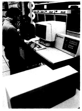
Sperry's 1100/90 SV models offer 1100/60 and 1100/70 users a lower entry point into the 1100/90 Series. The uniprocessor 1100/91 SV is rated at 5.5 MIPS, while the dual-processor 1100/92 SV is rated at 10.2 MIPS.
