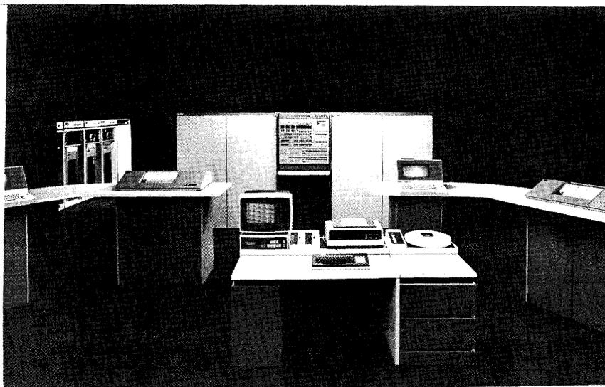
*The UNIVAC 1100/80 is the most powerful member of the 1100 Series family and is now available in five distinct models. Originally, only the single-processor 1100/81 and the dual-processor 1100/82 were offered. In October 1977, three more models were added: the low-end 1100/80 and the three- and four-CPU 1100/83 and 1100/84.*
