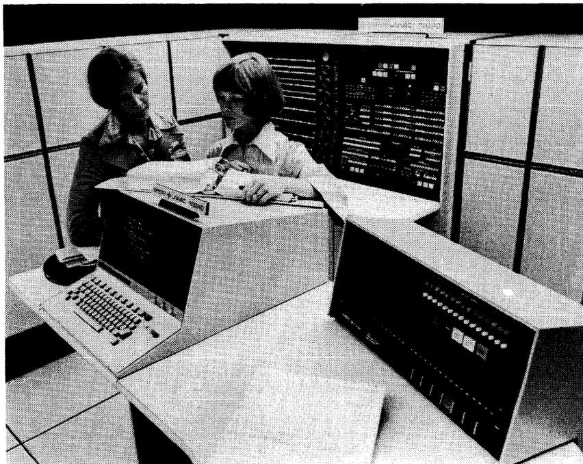
*The UNIVAC 1100/40 has an architecture similar to that of the earlier UNIVAC 1110 and employs the same two-level main storage/extended storage scheme. It differs from the earlier system in the use of faster bipolar memory for main storage instead of the 1110's plated-wire technology and in the use of 800-nanosecond error-correcting MOS memory for extended storage instead of core. The use of denser semiconductor memory permitted the 1100/40 to have twice the memory capacity of the 1110.*
