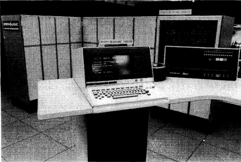
*The UNIVAC 1100/20 was the direct successor to the 1108. It has the same instruction set as the earlier model but features a modified addressing structure that permits improved multiprogramming. Early in 1978, UNIVAC introduced enhancements to the lower-priced 1100/10 system that boosted its performance level by 20 to 30 percent, making the 1100/10 a more cost-effective system than the 1100/20.*
