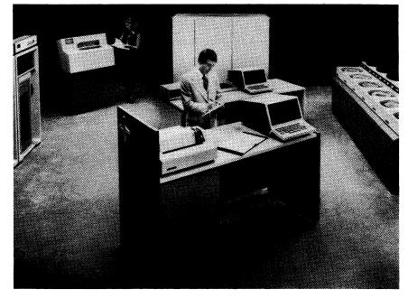
The 1100/60 System has been enhanced to support up to 4 central processors and up to 8192K words of main memory. A single processor configuration can include a maximum of four consoles; a multiprocessor configuration, a maximum of seven consoles.
