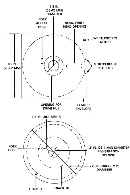
Figure 2-2. Typical Flexible Diskette Medium
