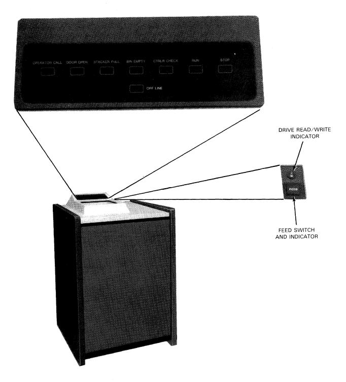
Figure 4–2. Operator Panel Controls and Indicators
