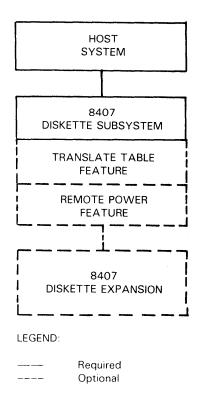
Figure 2–1. 8407 Diskette Drive Configurator
