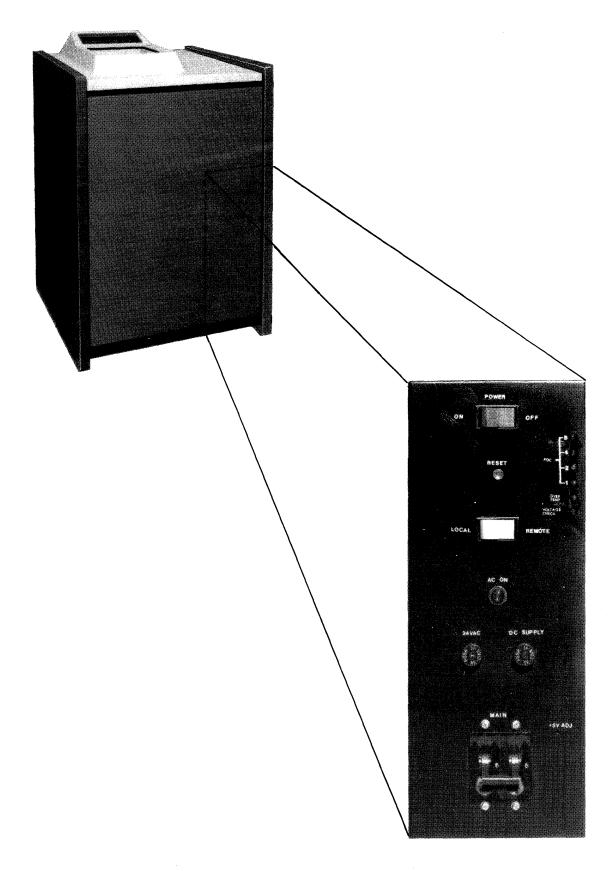
Figure 4—1. Power Panel Controls and Indicators
