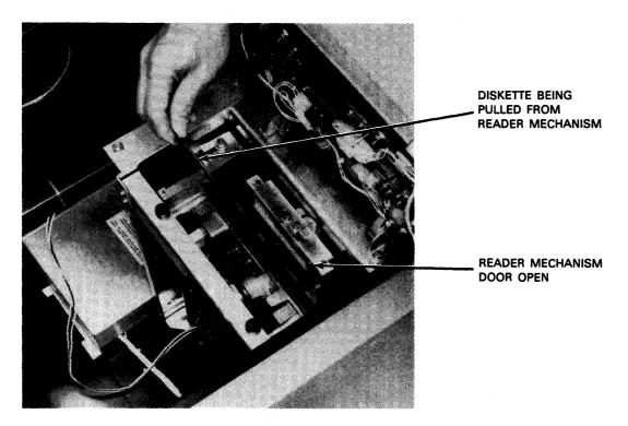
e. Removing jammed diskette from reader mechanism
