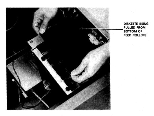
d. Removing jammed diskette from feed rollers
