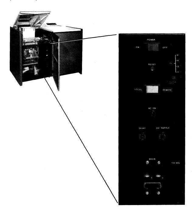
Figure 3-2. Power Control Panel
