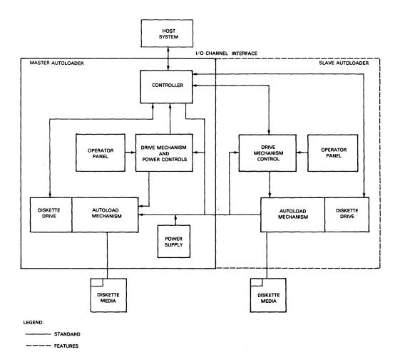
Figure 2-1. Block Diagram of 8407 Diskette Drive Functions
