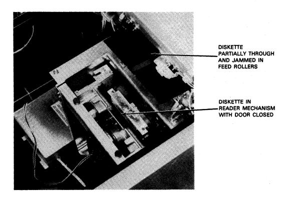
c. Jammed diskettes in feed rollers and reader mechanism
