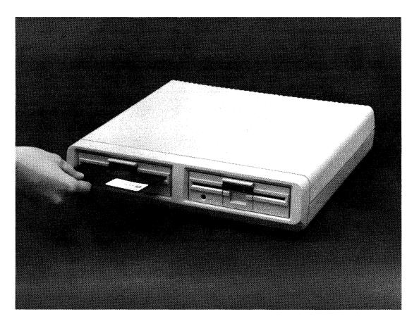
Figure 3–2. Inserting a Diskette into the Diskette Subsystem
