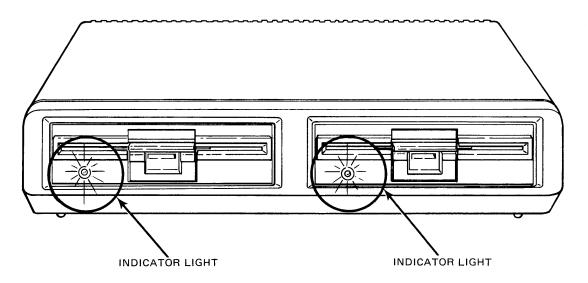
Figure 2–4. Indicator Lights on the Diskette Subsystem
