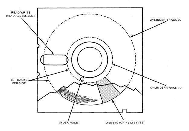
Figure 3–3. Track and Sector Format for Double-Density Diskettes (512 Bytes per Sector)
