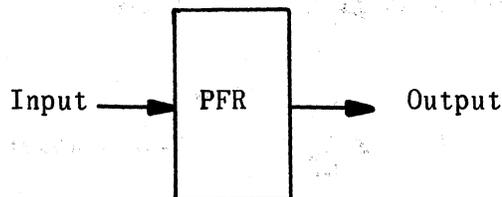
A delay of 0.5  $\mu$ sec exists between the input of the pulseformer and the output.
