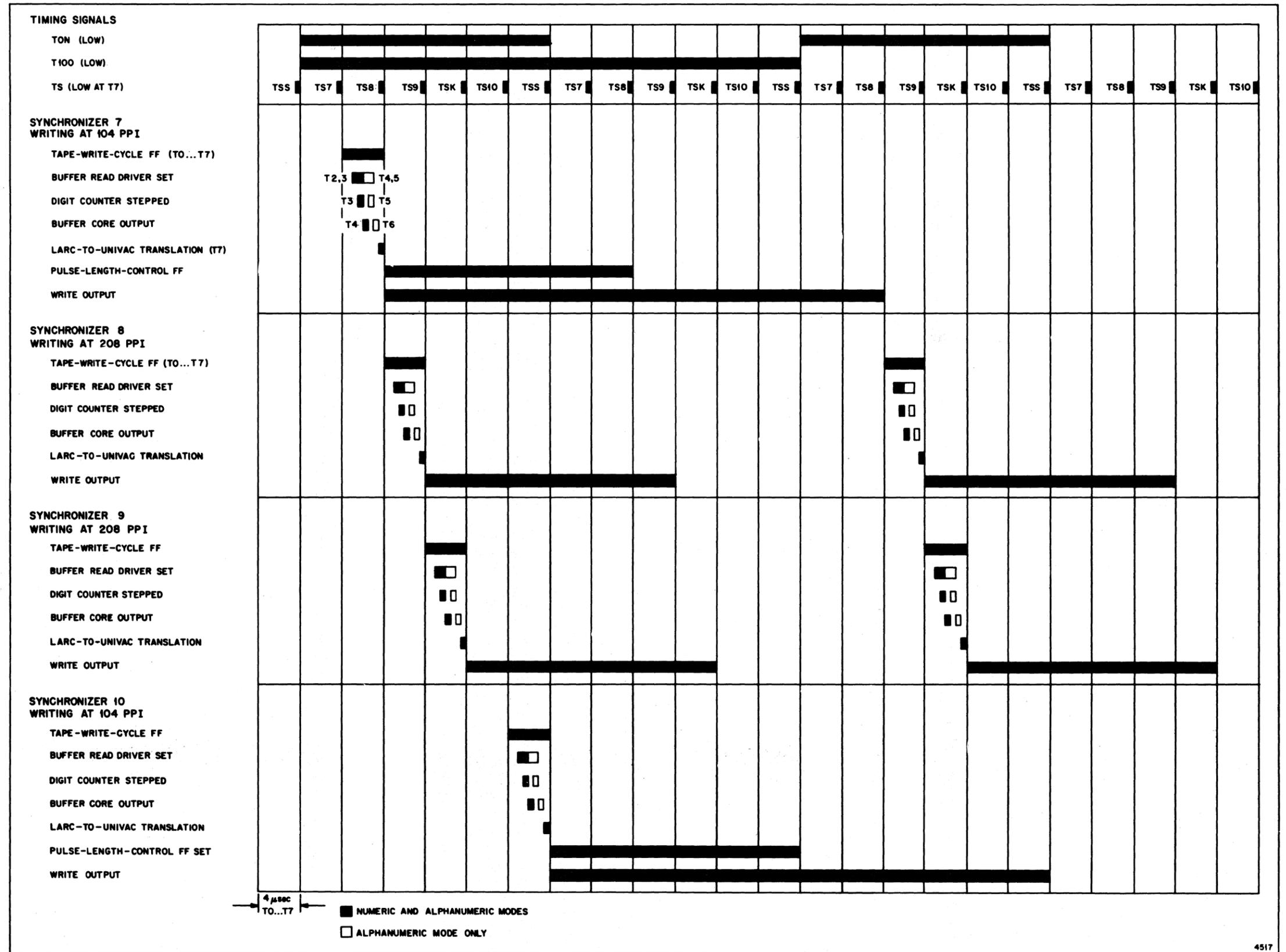
Figure 5-1. Write Cycle Timing, Larc System, Serial 1
