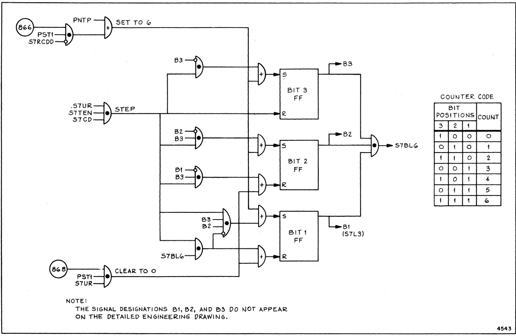
Figure 6-3. Univac Blockette Counter (D 807 888)
