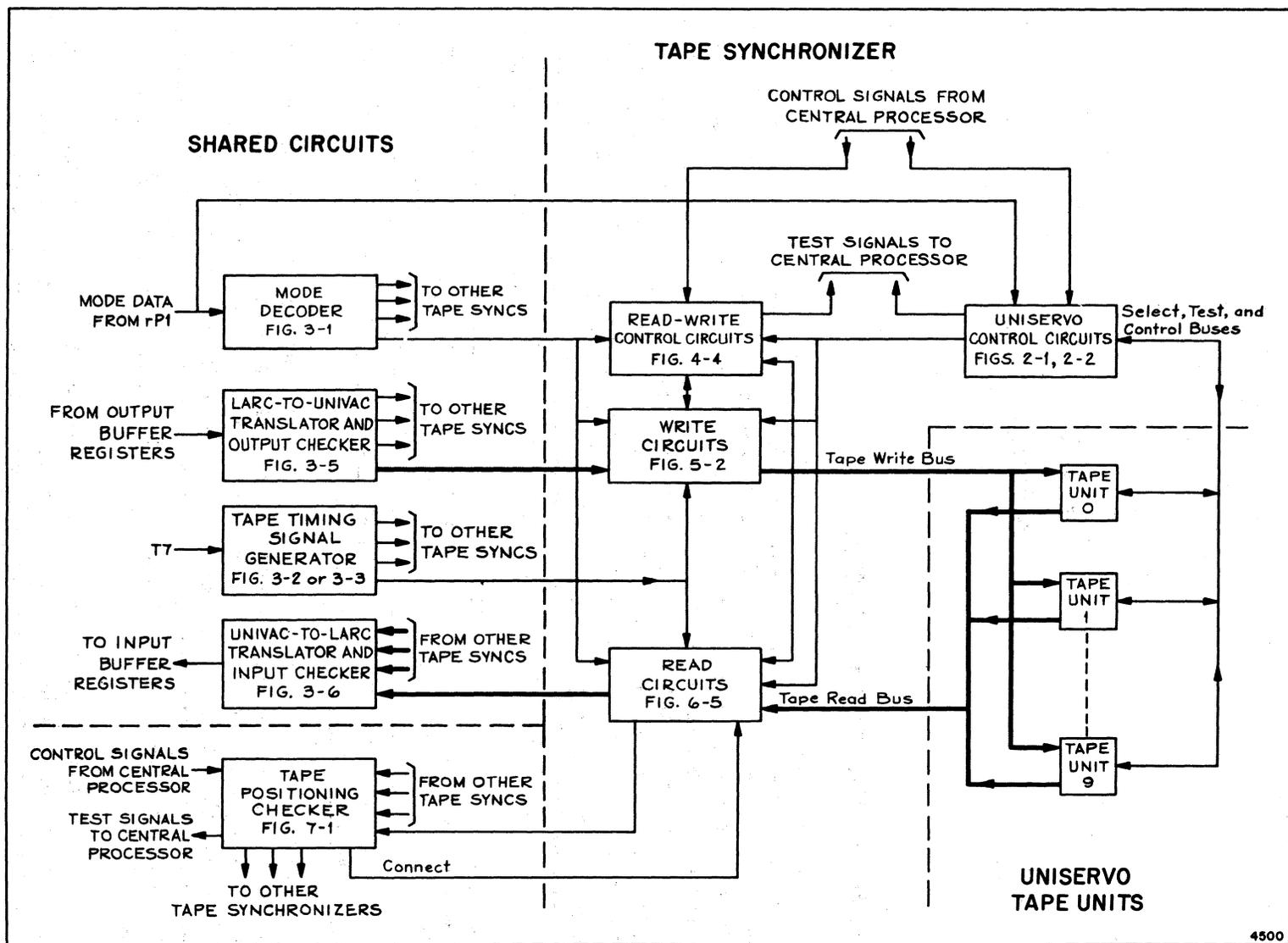
Figure 1-1. Magnetic Tape Synchronizer System, Block Diagram
