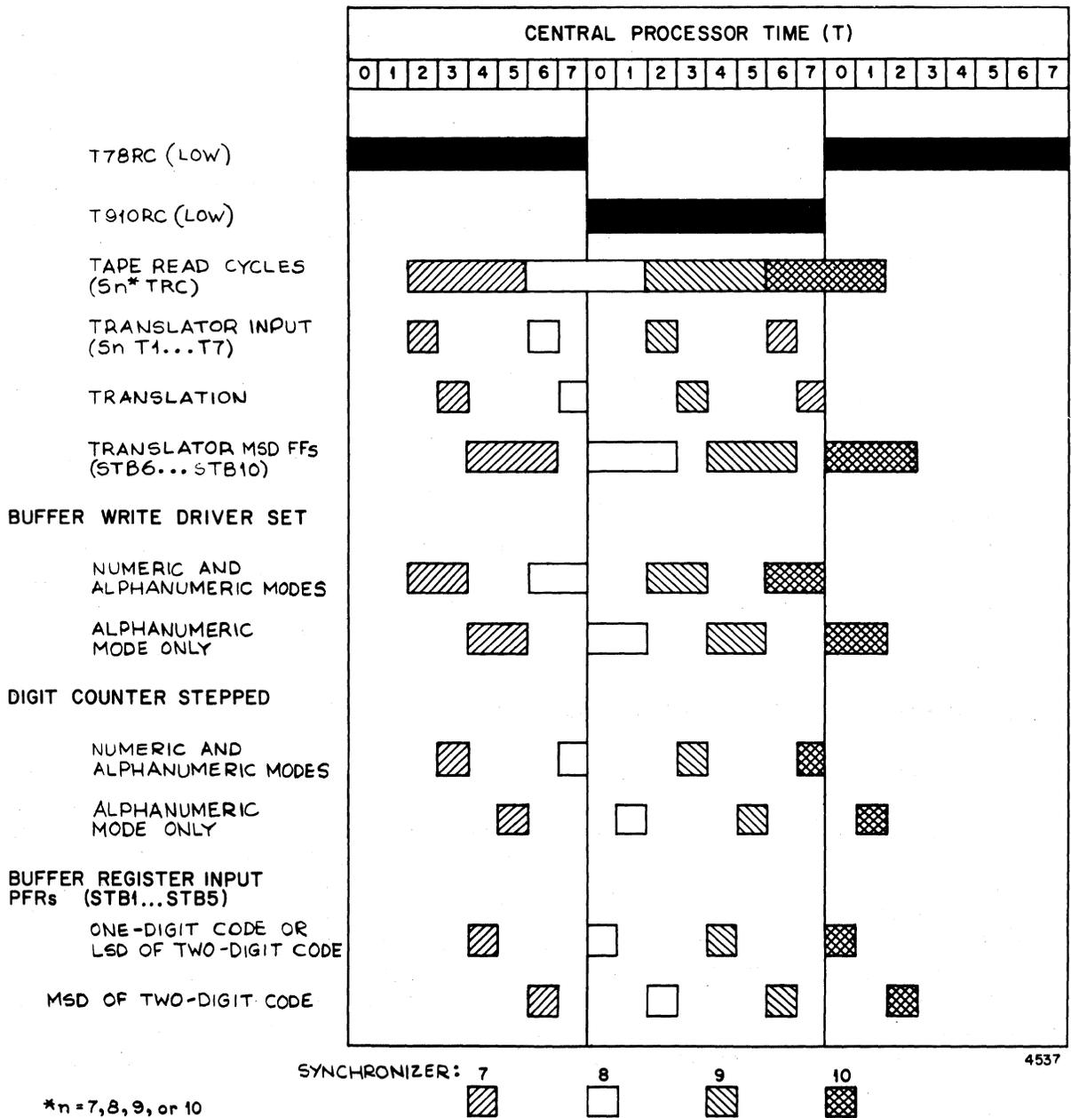
Figure 6-2. Input Timing for Four Consecutive Read Cycles on Different Synchronizers
