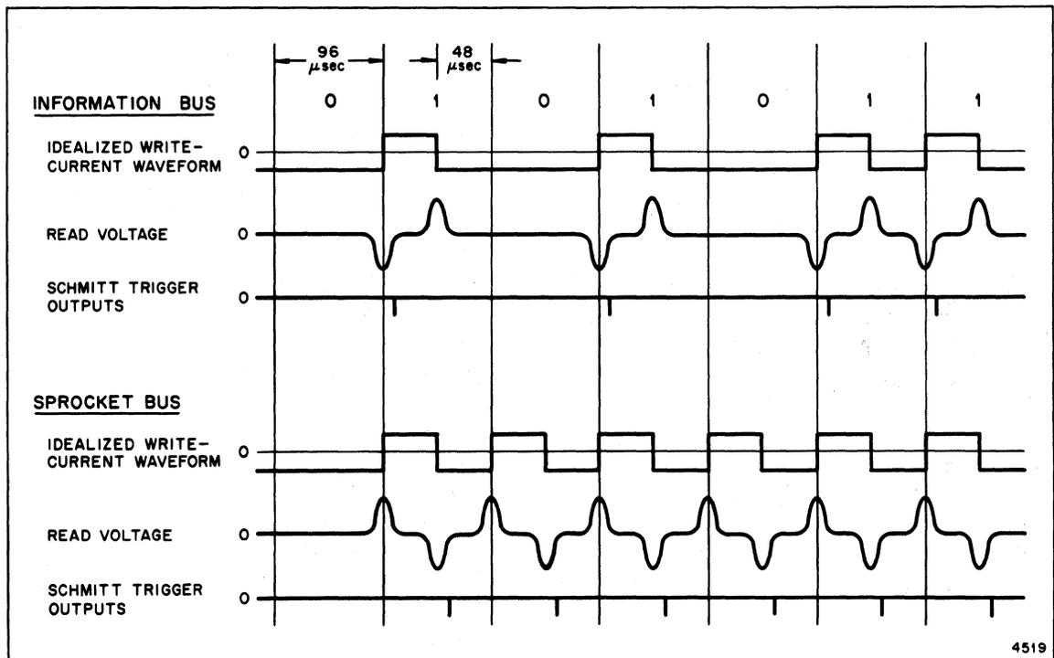
Figure 6-1. Read and Write Waveforms at 104 PPI
