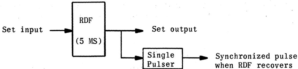
A single pulser following an RDF produces a synchronized output pulse when the RDF recovers.
