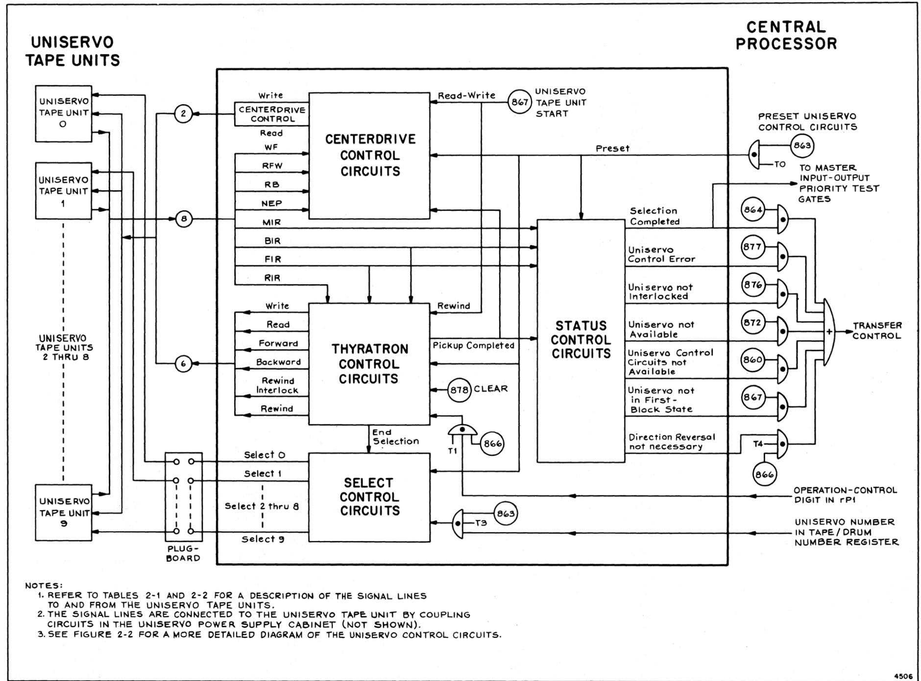
Figure 2-1. Uniservo Control Circuits, Block Diagram
