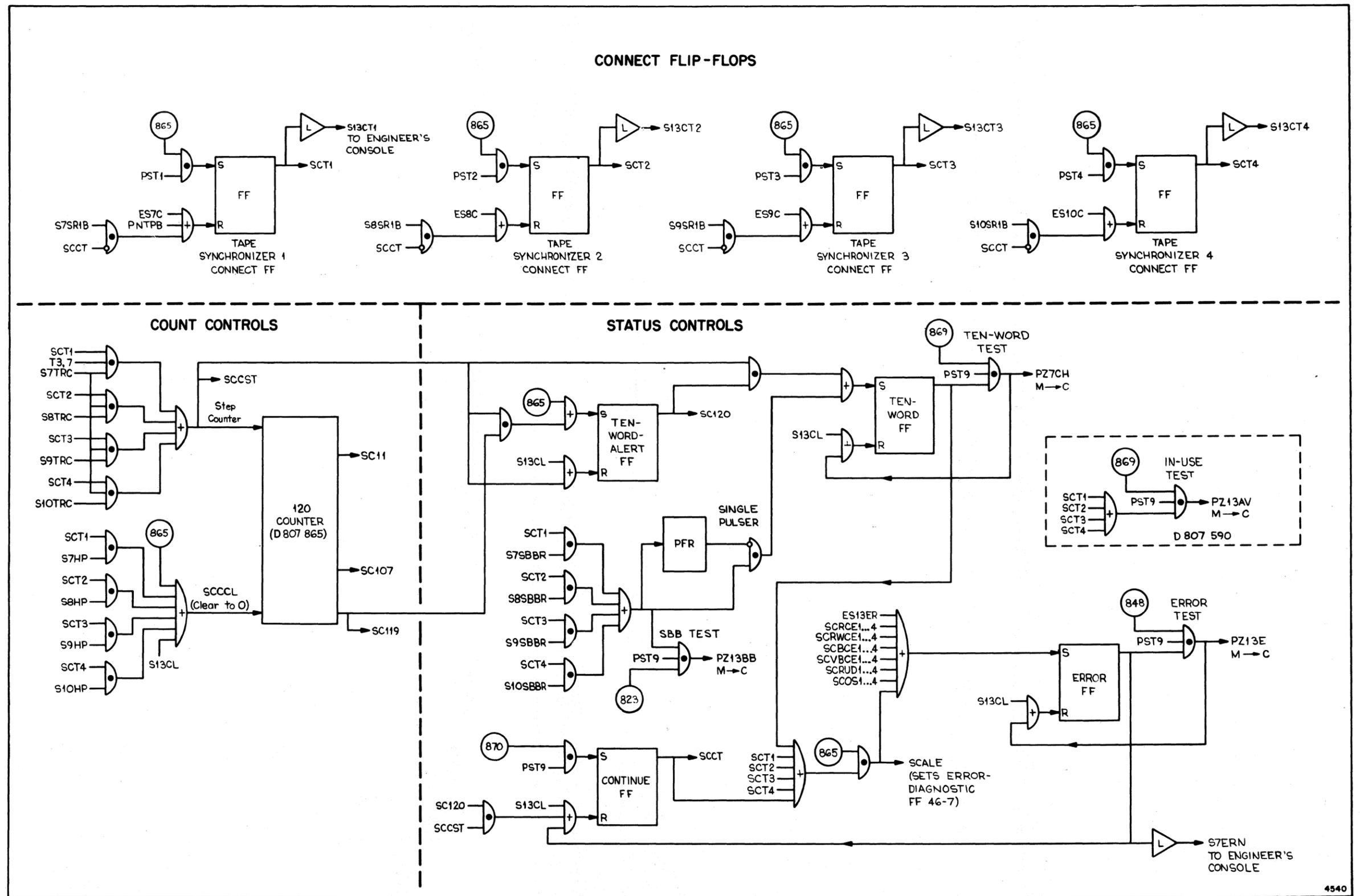
Figure 7-1. Tape Positioning Checker (D 807 865 and D 807 866)
