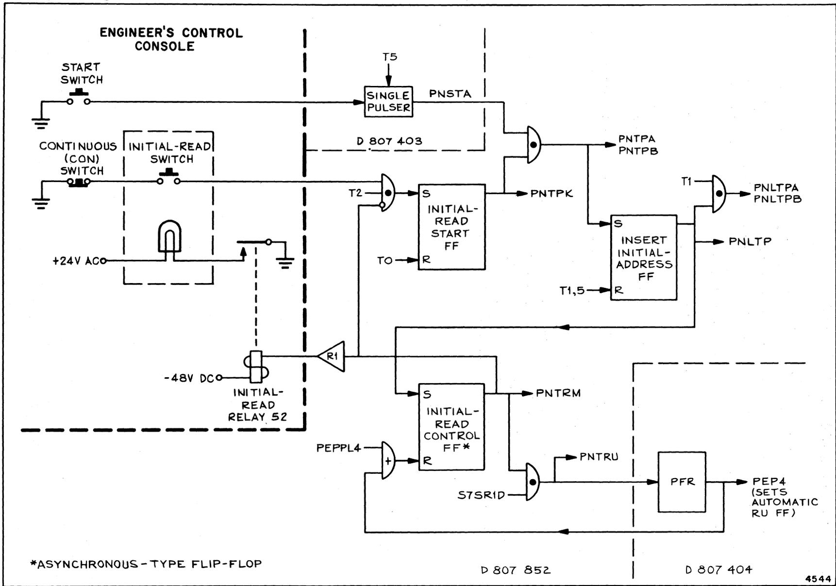
Figure A-1. Initial-Read Circuits (D 807 852)
