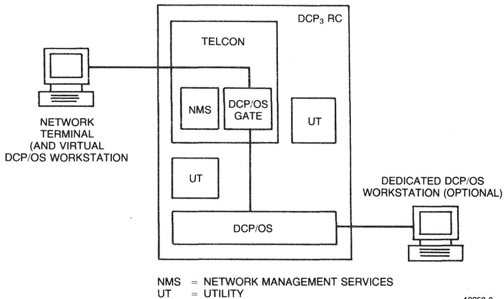
Figure 3-2. Communicating with the DCP/OS
