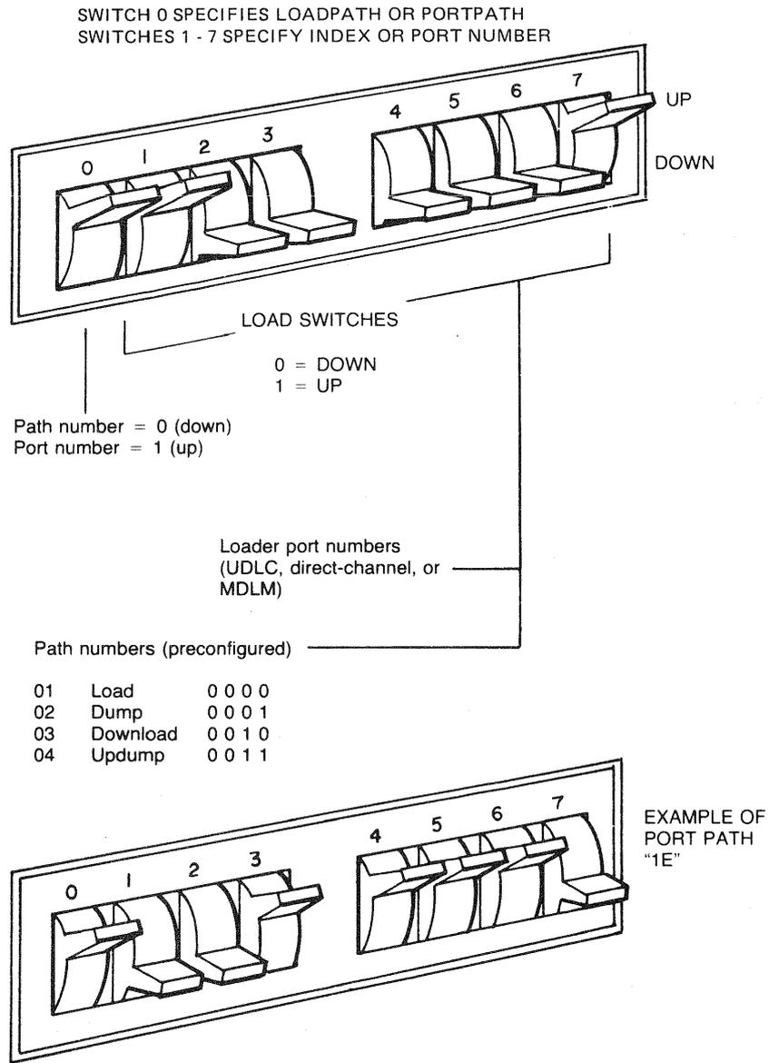
Figure 3-3. Example Load Switch Settings
