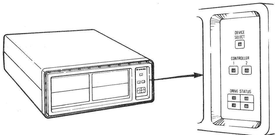
Figure 5-1. 8441 Subsystem Control Panel
