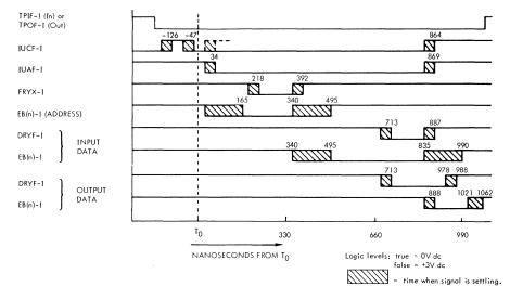
\* THE INTERRUPT CLOCK (IUCF-I) RATE IS FIXED AT A PERIOD OF 330 SECONDS.
