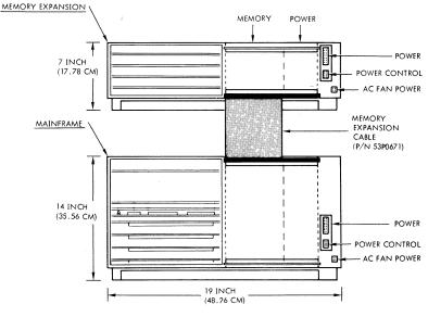
Figure 1-6. Memory Expansion (Rear View)
