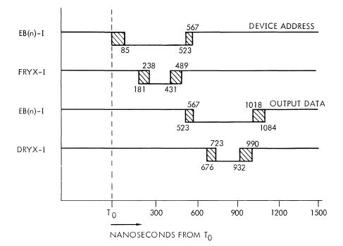
$T_0$  is the start of the I/O microflow for the data transfer out instruction
