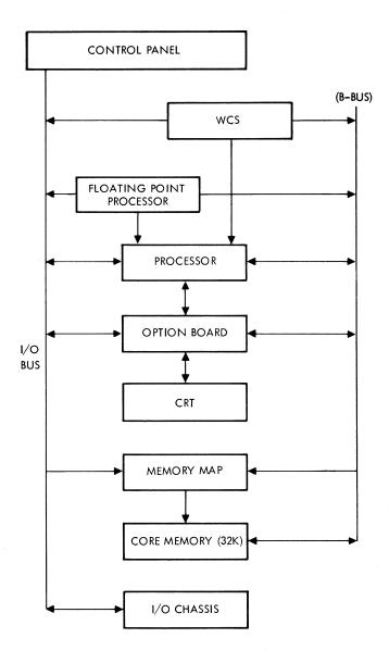
Figure 9-7. WCS and FPP Block Diagram
