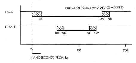
$T_{0}$  is the start of the  $I\!/\!O$  microflow for the external control instruction.
