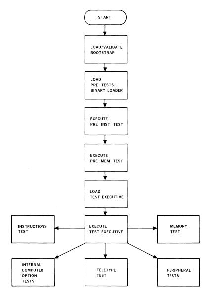
NOTE: The Test Executive operates with only one test program in memory at a time.
