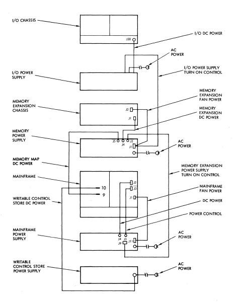
Figure 1-8. Power Distribution/Control (Rear View)
