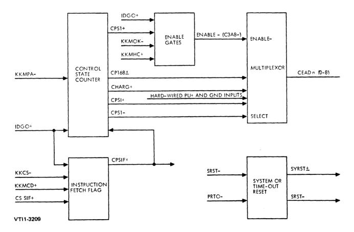
Figure 4-25. Central Processor Control, Block Diagram
