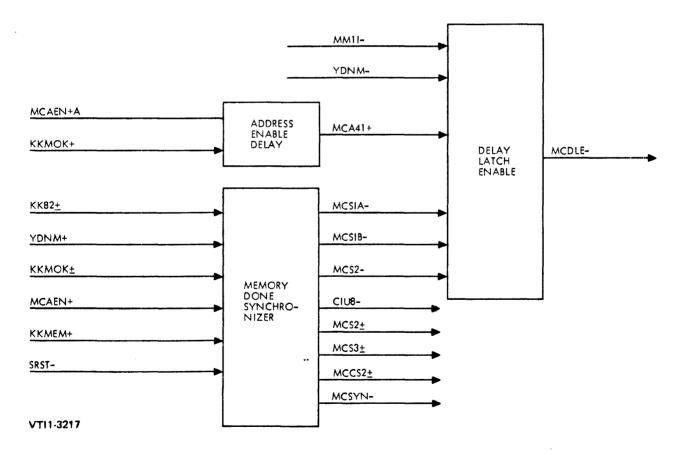
Figure 4-30. Memory Sequencer, Block Diagram
