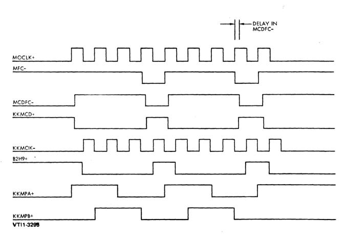
Figure 4-34. Retiming Clock Generator Waveforms
