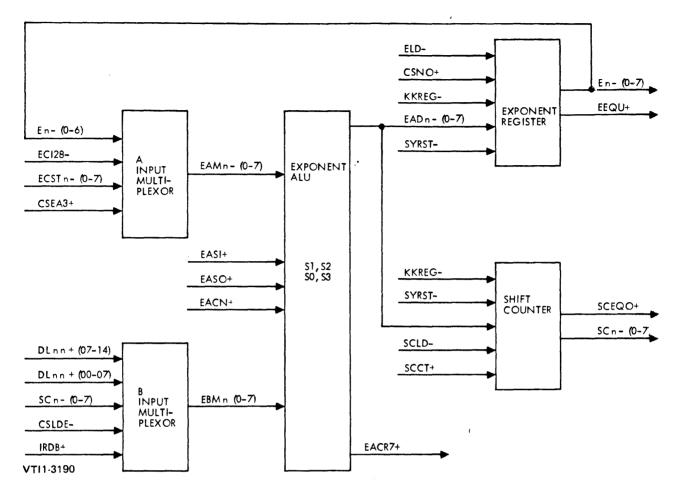
Figure 4-53. Exponent Loop, Block Diagram
