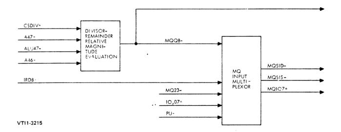
Figure 4-49. MQ Control, Block Diagram
