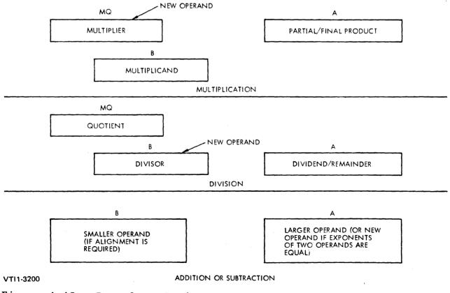
Figure 4-45. Data Loop Register Usages
