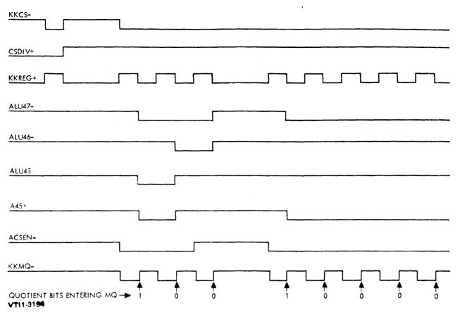
Figure 4-37. Timing at Start of CSDIV Microinstruction  $\begin{pmatrix} 0.11111100 - - \\ 0.11100000 - - \end{pmatrix}$
