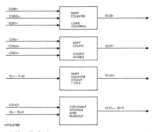
Figure 4-55. Shift Counter Control and Constant Storage
