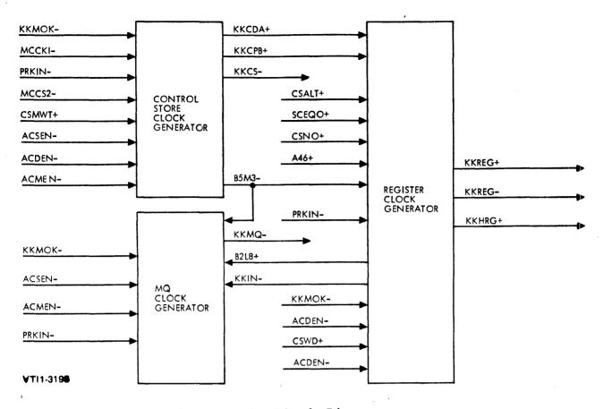
Figure 4-32. Clock Control, Block Diagram
