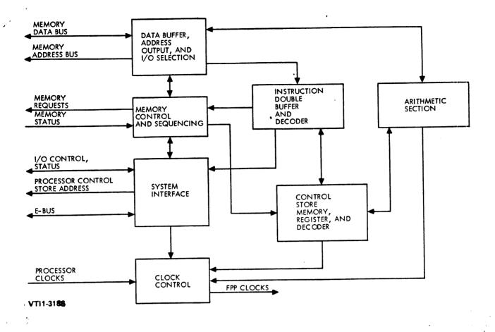
Figure 4-1. FPP Simplified Functional Block Diagram
