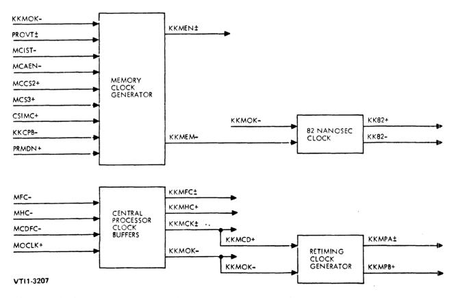
Figure 4-33. System Clock Generator, Block Diagram
