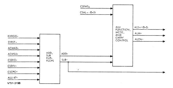
Figure 4-50. ALU Control, Block Diagram
