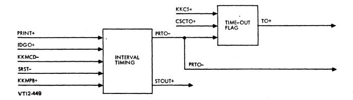
Figure 4-27. Priority Control, Block Diagram
