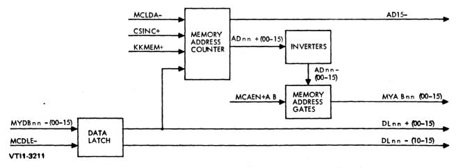
Figure 4-39. Data Latch and Address Output, Block Diagram
