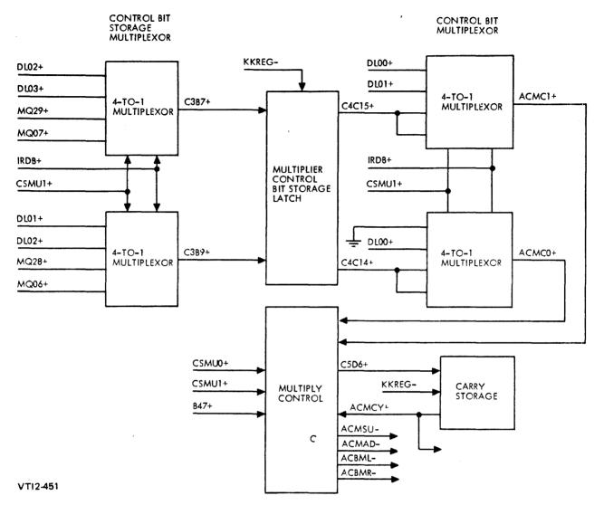
Figure 4-47. Multiply Control, Block Diagram
