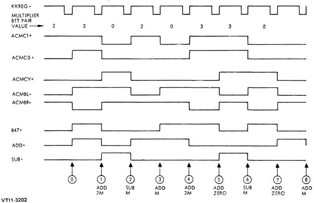
Figure 4-48. Example of Multiply Control Timing
