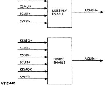
Figure 4-35. Arithmetic Clock Control, Block Diagram
