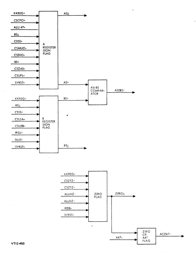
Figure 4-51. Sign and Zero Flags, Block Diagram
