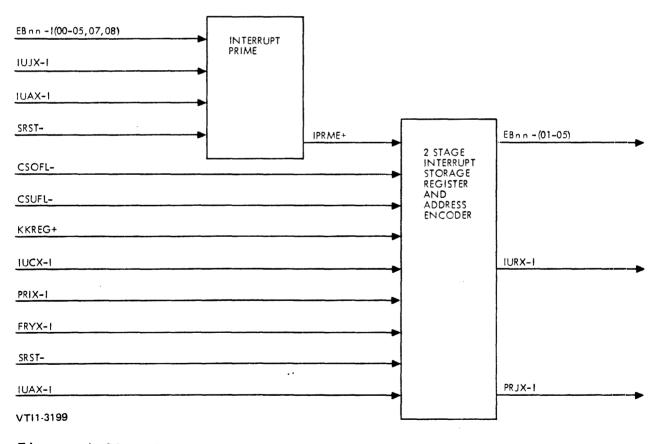
Figure 4-29. Interrupt Interface, Block Diagram
