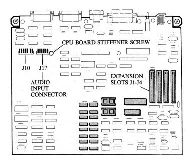
4.2 256K CPU BOARD OR 256K CPU BOARD WITH GATE ARRAYS
