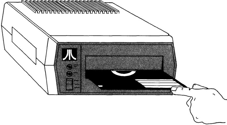
Now turn the computer on by pushing the power switch to the ON position. If your computer was already on, turn it off, pause a moment, then turn it back on. The switch is located on the right side of the computer, just past the 2-CHAN-3 switch. On the console, the red light just below the START button will also light. The drive takes about half a minute to load VisiCalc into RAM memory.
